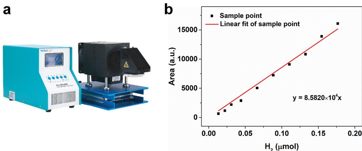
**Figure S11.** (a) The used xenon lamp PLS-SXE300D. (b) H<sub>2</sub> peak area verse the number of moles of hydrogen and polynomial fit of sample point to be H<sub>2</sub> normalized curve.
