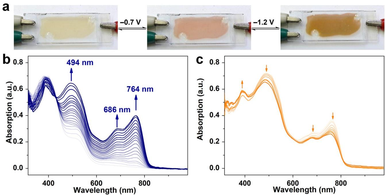
**Figure S9.** (a) Solution-based electrochromic device with **5c** (no electrolyte). (b) Spectroelectrochemistry of **5c** for first reduction. (b) Spectroelectrochemistry of **5c** for second reduction.
