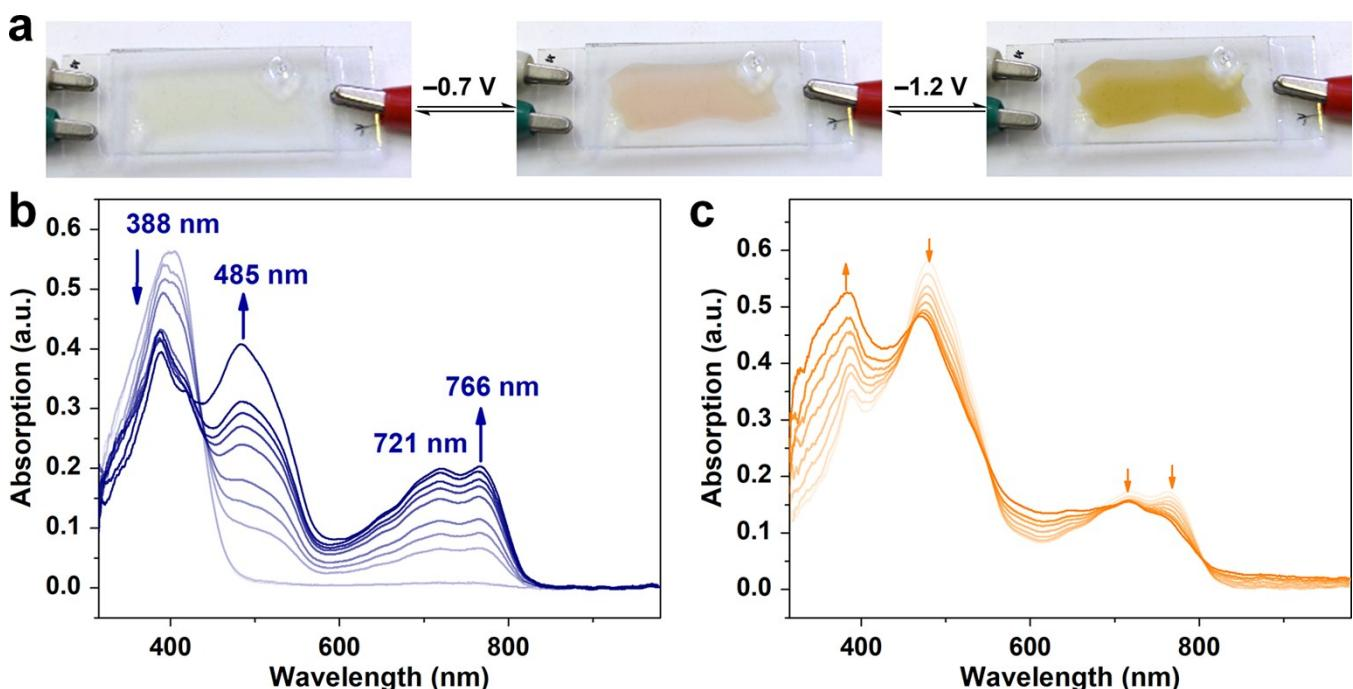
**Figure S7.** (a) Solution-based electrochromic device with **5a** (no electrolyte). (b) Spectroelectrochemistry of **5a** for first reduction. (b) Spectroelectrochemistry of **5a** for second reduction.
