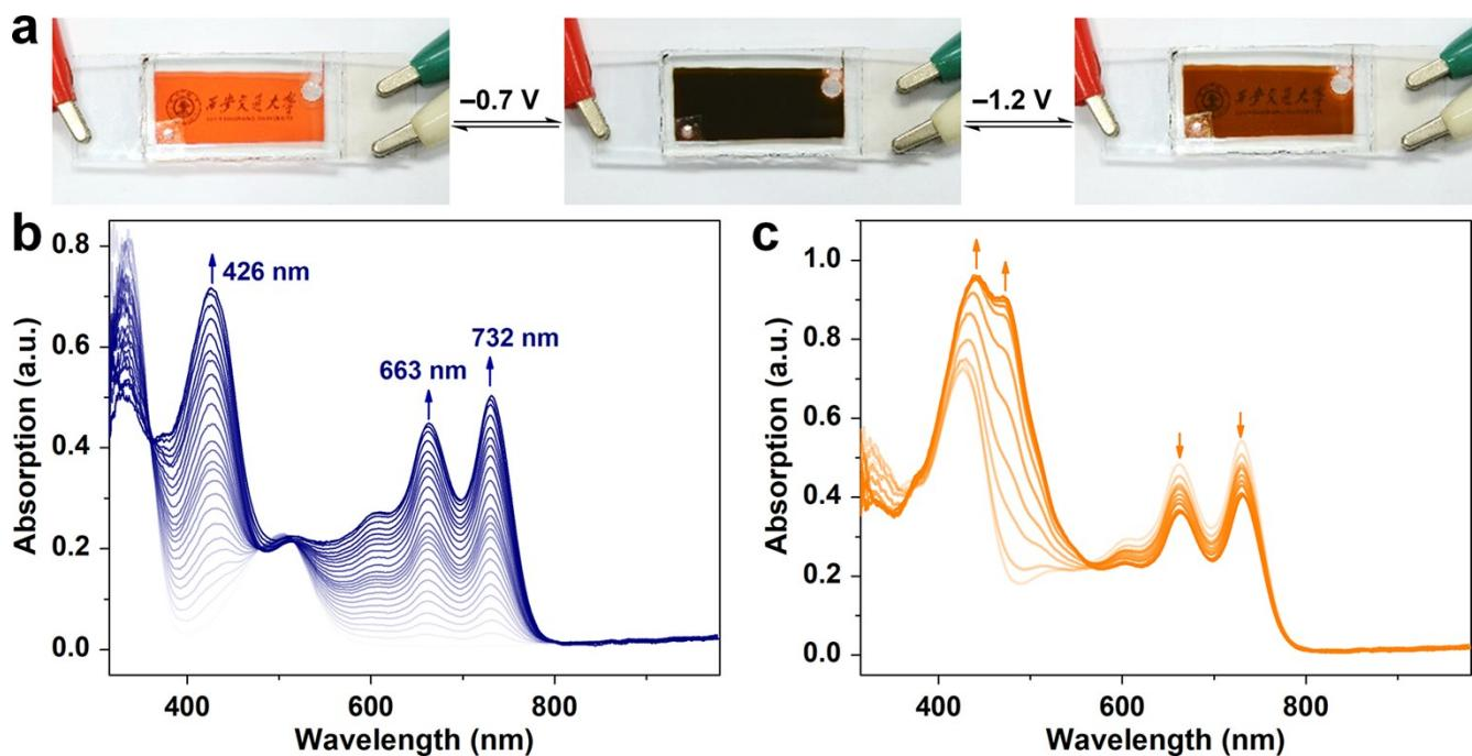
**Figure S6.** (a) Solution-based electrochromic device with **3c** (no electrolyte). (b) Spectroelectrochemistry of **3c** for first reduction. (b) Spectroelectrochemistry of **3c** for second reduction.
