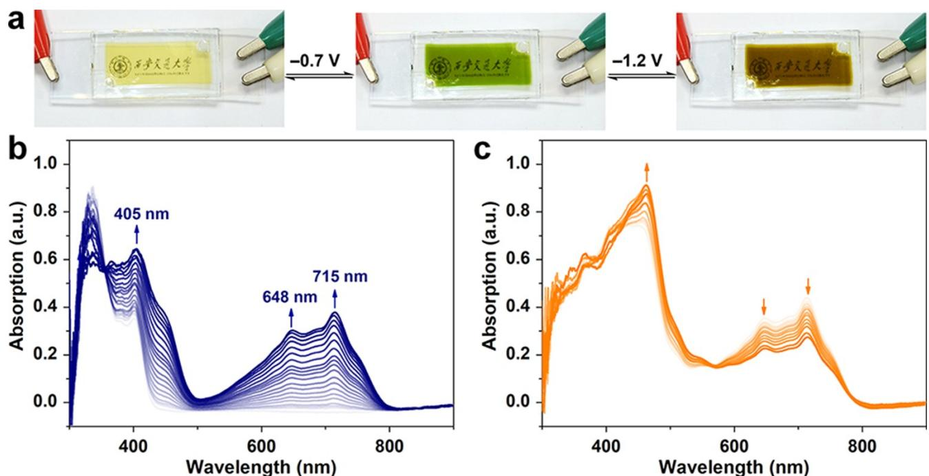
**Figure S5.** (a) Solution-based electrochromic device with **3a** (no electrolyte). (b) Spectroelectrochemistry of **3a** for first reduction. (b) Spectroelectrochemistry of **3a** for second reduction.
