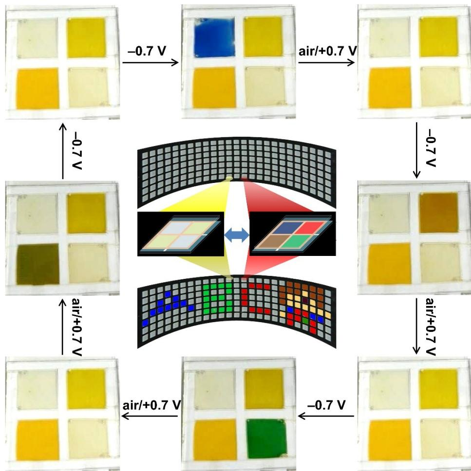
**Figure S10.** Colorful display of ECDs with four-latticed pixel matrix and schematic diagram of flexible E-link in the center.
