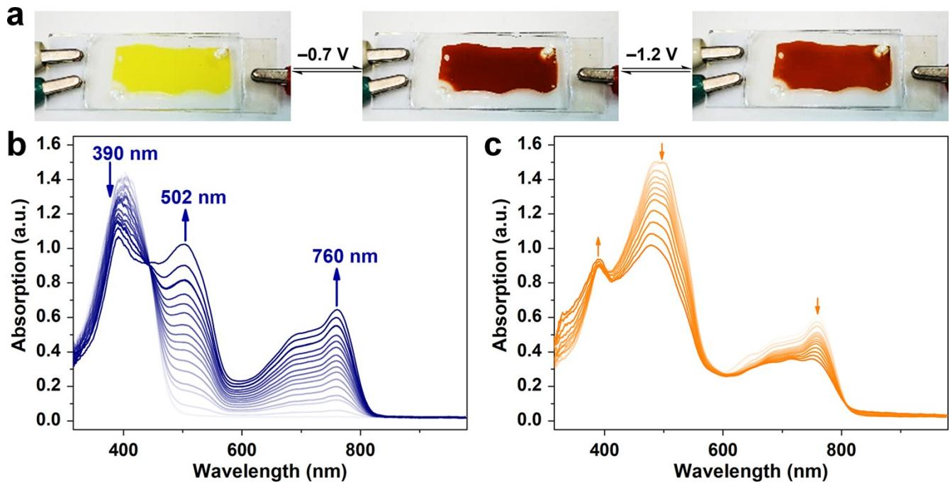
**Figure S8.** (a) Solution-based electrochromic device with **5b** (no electrolyte). (b) Spectroelectrochemistry of **5b** for first reduction. (b) Spectroelectrochemistry of **5b** for second reduction.
