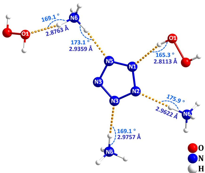
Fig. S2. Five types of hydrogen bonds in  $\text{NH}_4\text{N}_5 \cdot \frac{1}{2}\text{H}_2\text{O}_2$  at 150K.
