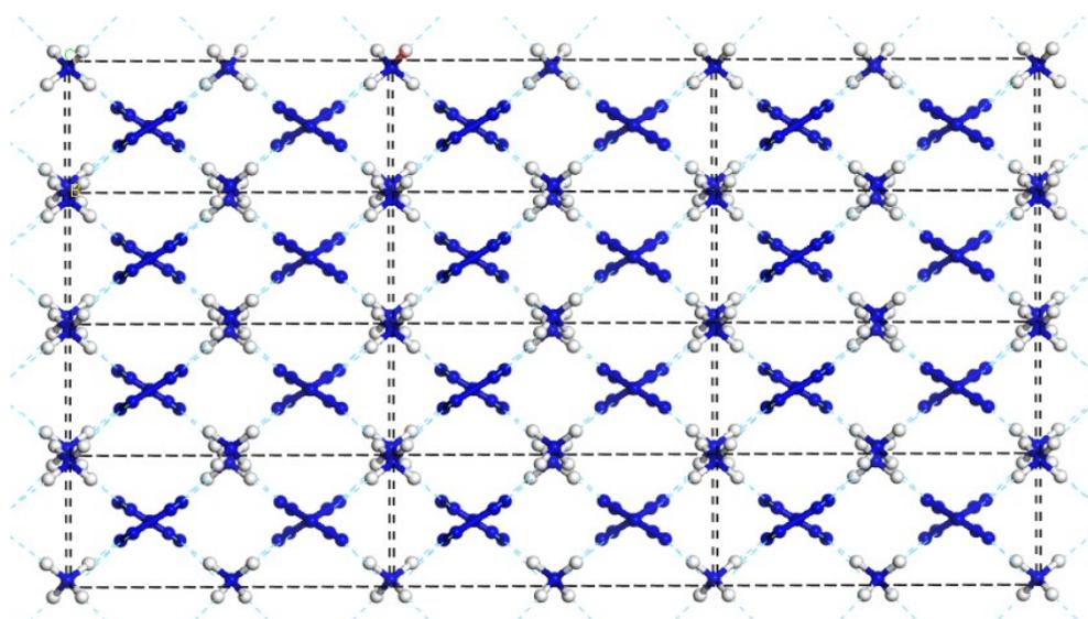
**Fig. S4.** The packing diagram of  $\text{NH}_4\text{N}_5$  viewed along the c axis.
