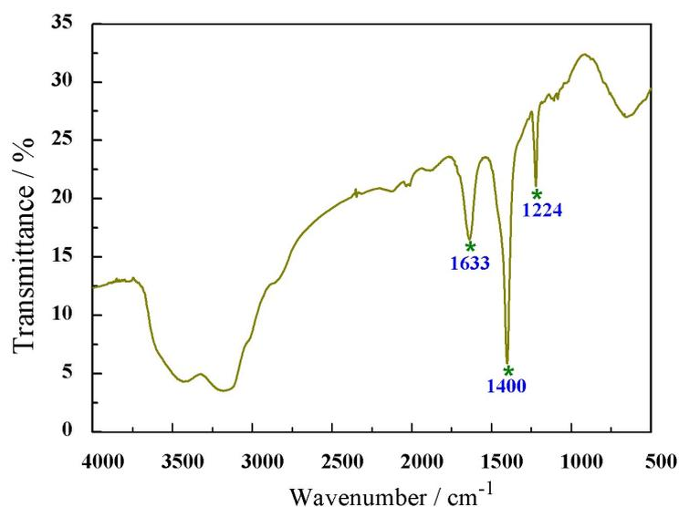
**Fig. S5.** Infrared spectra of  $\text{NH}_4\text{N}_5 \cdot \frac{1}{2}\text{H}_2\text{O}_2$ , which indicates cyclo- $\text{N}_5^-$  has an absorption peak in the IR band at  $1224 \text{ cm}^{-1}$ , which matches the reported vibrational peak at  $1224 \text{ cm}^{-1}$ .<sup>5</sup>
