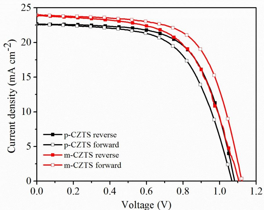
Fig. S7. Typical J-V curves for FAPbI<sub>3</sub> perovskite solar cells employing both p-CZTS and m-CZTS hole transporting layers.
