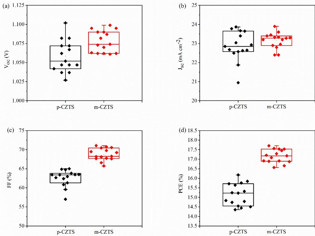
Fig. S6. Statistical photovoltaic parameters (a)  $V_{oc}$ , (b)  $J_{sc}$ , (c) FF, and (d) PCE for  $\text{FAPbI}_3$  perovskite solar cells employing both p-CZTS and m-CZTS hole transporting layer.
