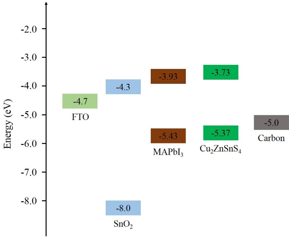
Fig. S2. Energy band diagram of the perovskite solar cells. The band levels of FTO, SnO<sub>2</sub>, MAPbI<sub>3</sub>, Cu<sub>2</sub>ZnSnS<sub>4</sub> and Carbon are extracted from references[1, 2].
