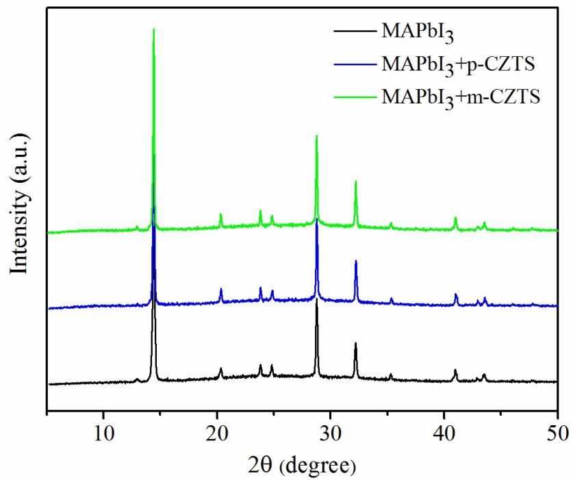
Fig. S4. XRD patterns for MAPbI<sub>3</sub> film, MAPbI<sub>3</sub>/p-CZTS film, and MAPbI<sub>3</sub>/m-CZTS film.
