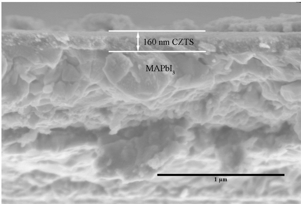
Fig. S3. Cross sectional SEM image of a typical p-CZTS film deposited on MAPbI<sub>3</sub>. The thickness of p-CZTS film is estimated to be 160 nm.
