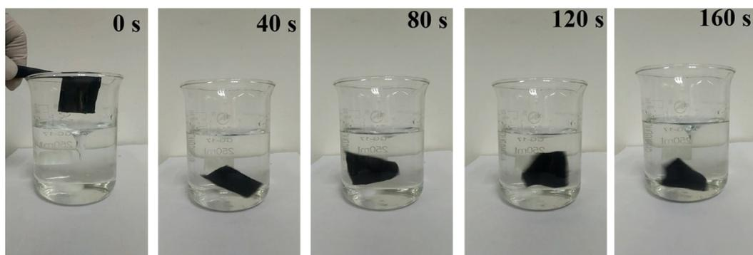
**Fig. S5** Digital images of the mechanical washing process of M-textile-17.3.
