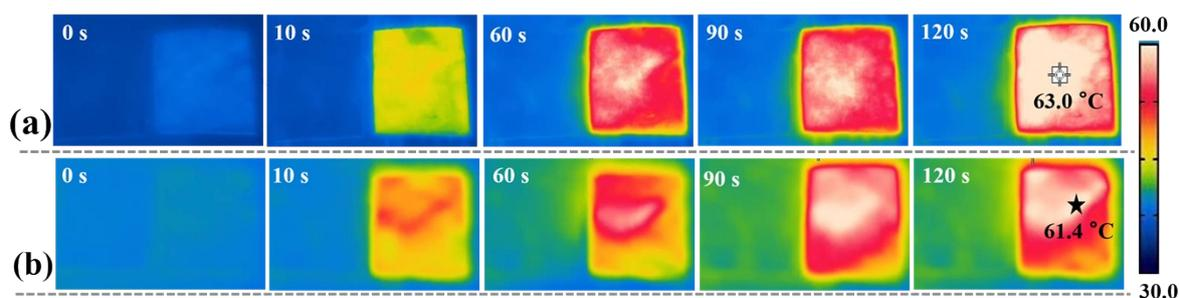
**Fig. S15** IR images of the M-textile-17.3 exposed to sunlight at 12 AM a) before and b) after machine washing of 100 minutes.
