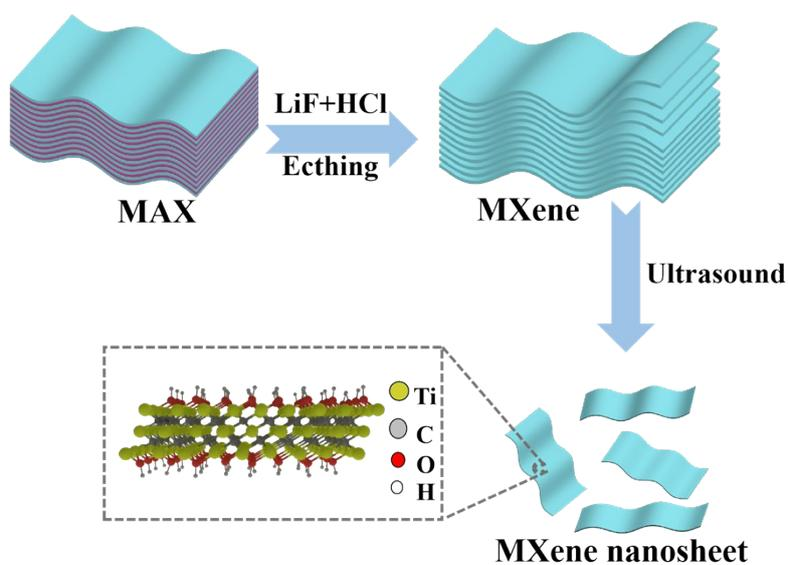
**Fig. S1** Schematic illustration of the process for etching  $\text{Ti}_3\text{C}_2\text{Tx}$  MXene.
