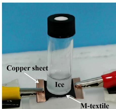
**Fig. S10** Schematic diagram of electric heating deicing device based on M-textile.
