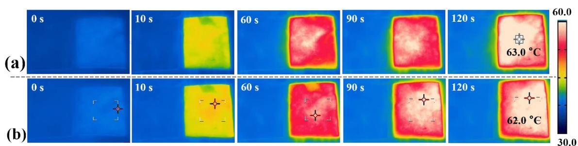
**Fig. S14** IR images of a) 1st and b) 20th cyclic photothermal conversion performance of M-textile-17.3 including exposing to sunlight (2 min) and then shading sunlight (2 min) at 12 AM.
