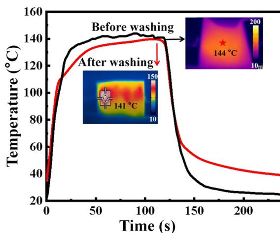
**Fig. S9** Electrical heating performance (temperature rise curve and IR image at saturated temperature) of M-textile-17.3 textile at 3V before and after machine washing for 100 minutes.
