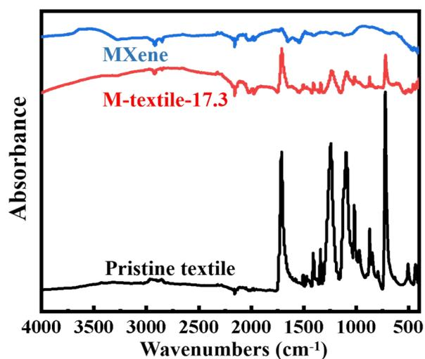
**Fig. S4** ATR-IR spectra of the  $\text{Ti}_3\text{C}_2\text{T}_x$ , pristine textile, M-textile with different MXene content, respectively.
