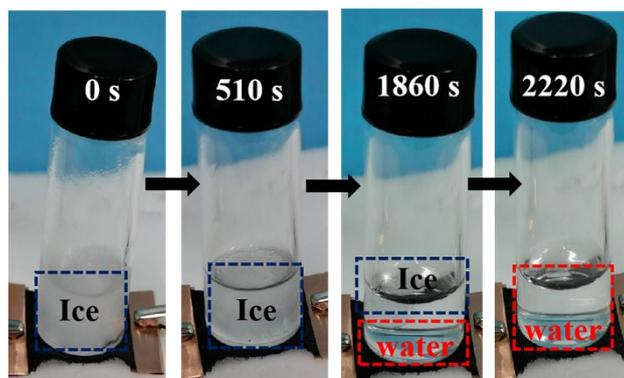
**Fig. S11** Digital image of deicing process without applying voltage.
