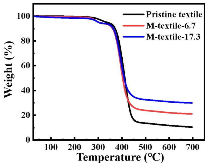
**Fig. S19** TG curves of pristine textile and M-textile with different MXene content, respectively.
