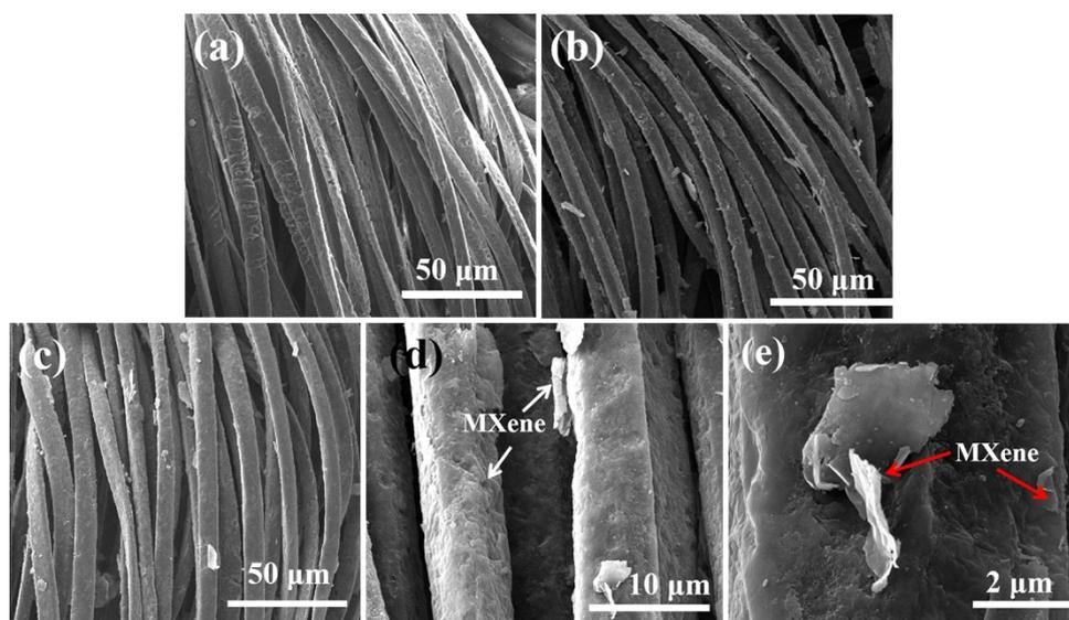
**Fig. S3** SEM images of a) pristine textile, b) M-textile-17.3, c), d) and e) M-textile-4.7 at low and high magnification, respectively.
