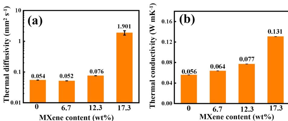
**Fig. S7** a) Thermal diffusivity and b) thermal conductivity of pristine textile and M-textile with different MXene content, respectively.
