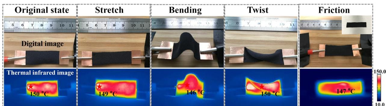
**Fig. S8** Joule heating performance of M-textile-17.3 in the state of stretch ( $\sim 120\%$ ), bending, twist or after one thousand time of friction on a paper.
