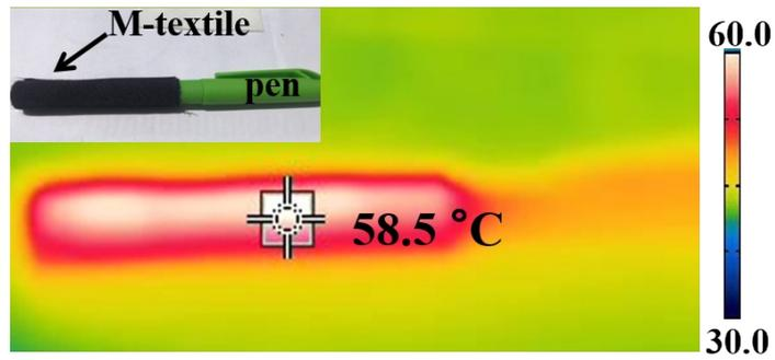
**Fig. S16** IR images of a pen wrapped with M-textile-17.3 irradiated by sunlight at 12 AM.
