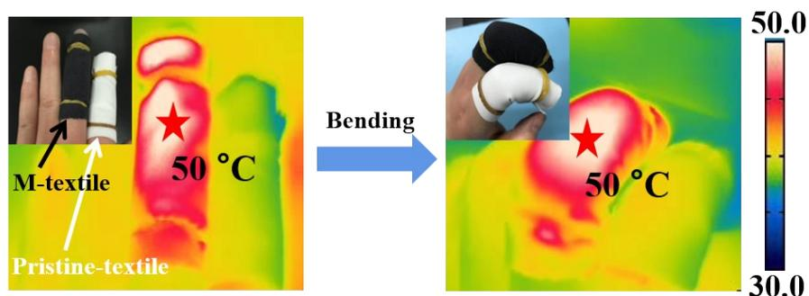
**Fig. S12** IR images of straight and bended figures wrapped with M-textile and pristine textile during FIR light irradiating at a distance of 20 cm.
