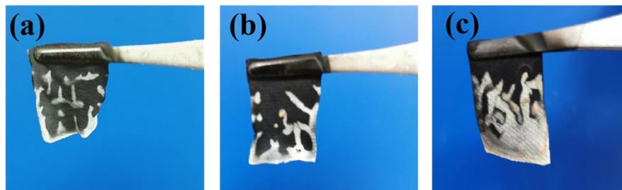
**Fig. S18** Digital images of textiles after burning: a) M-textile-6.7, b) M-textile-12.3 and c) M-textile-17.3, respectively.
