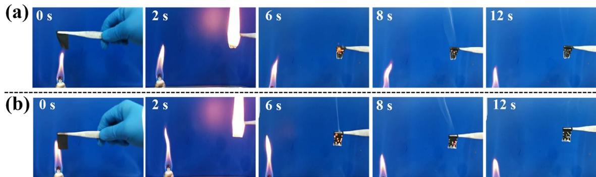
**Fig. S17** Digital images of the combustion process at different time of a) M-textile-6.7 and b) M-textile-12.3.
