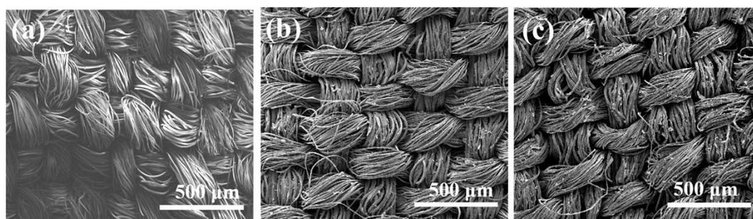
**Fig. S6** SEM images of a) pristine textile, b) M-textile-4.7, and c) M-textile-17.3 at high magnification.
