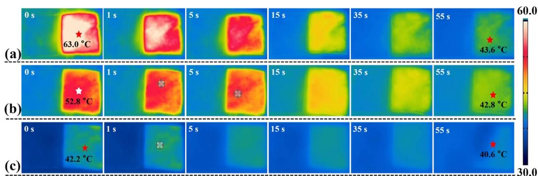
**Fig. S13** IR images of the M-textile-17.3 after shading the sunlight at different time: a) 12 AM, b) 3 PM and c) 5 PM (May 2, Zhengzhou, China).
