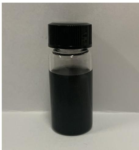
**Fig. S6.** Photograph of rGO/PPy-2-based ink. The rGO/PPy sheets were uniformly dispersed in ethanol.
