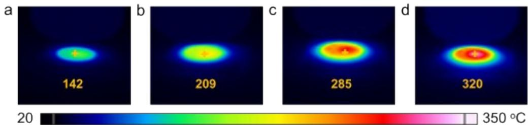
**Fig. S3.** IR thermal images of the rGO films on a PDMS substrate at different power densities of 0.8 (a), 1.5 (b), 2.2 (c), and 2.6 W cm<sup>-2</sup> (d), respectively.
