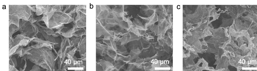
**Fig. S1.** SEM images of rGOF (a), rGO/PPyF-1 (b), and rGO/PPyF-2 (c).
