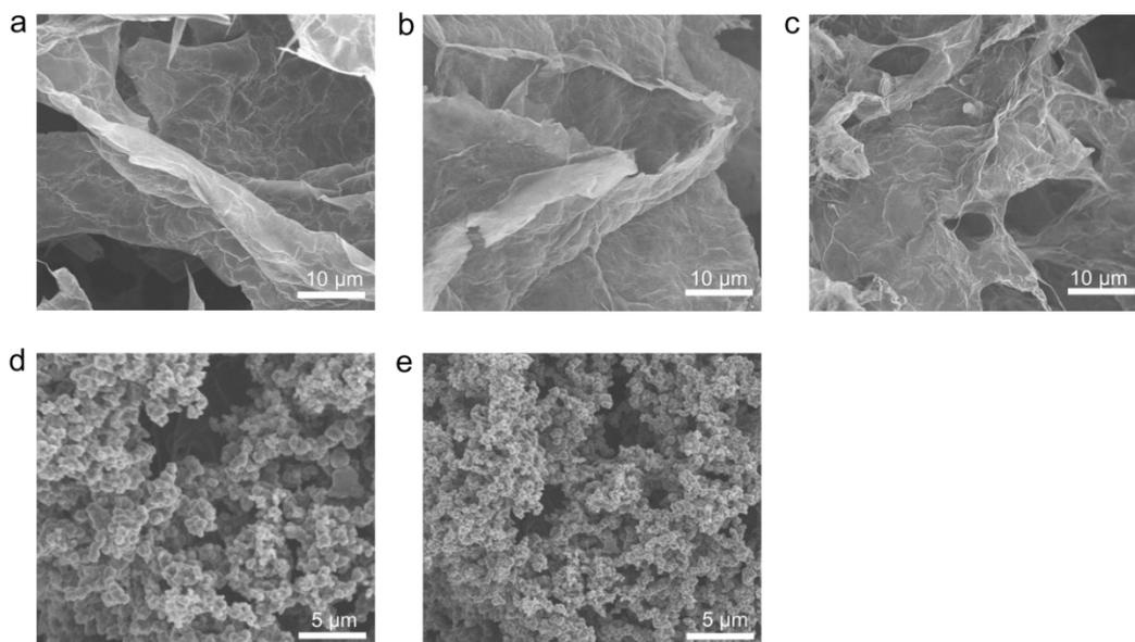
**Fig. S5.** (a-c) SEM images of the rGOF (a), rGO/PPyF-1 (b), and rGO/PPyF-2 (c) after a laser irradiation. (d,e) SEM images of the PPy powders before (d) and after (e) a laser irradiation.
