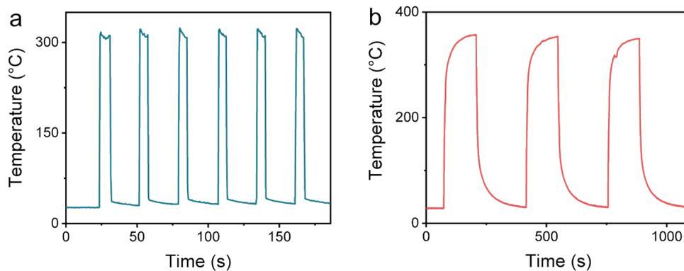
**Fig. S4.** On-off cycle response under a laser power density of 1.7 W cm<sup>-2</sup> for rGOF (a), and PPy (b).
