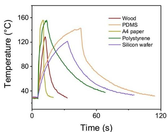
**Fig. S8.** Time-temperature curves of rGO/PPy-2-based films on the substrates of wood, PDMS, A4 paper, polystyrene, silicon wafer with the 808 nm NIR irradiation at the power density of  $0.8 \text{ W cm}^{-2}$ .
