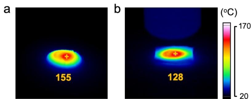
**Fig. S7.** IR thermal images of the rGO/PPy films on the substrates of A4 paper (a), and wood (b) with the 808 nm NIR irradiation at the power density of  $0.8 \text{ W cm}^{-2}$
