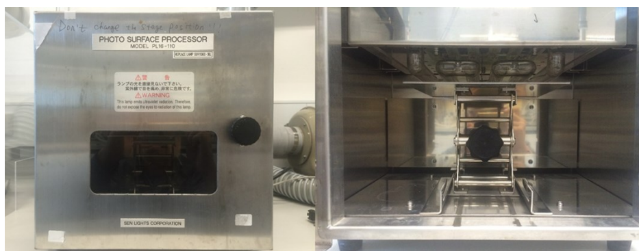
Fig. S1 Apparatus for UV/Ozone treatment.
