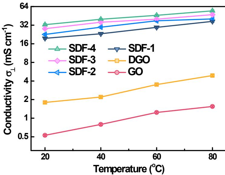
**Fig. S22.** Temperature-dependent vertical proton conductivities of the membranes under 100% RH.
