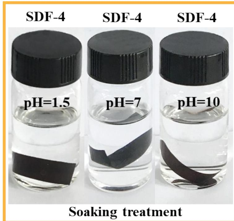
**Fig. S18.** Photos of the stability of SDF-4 membrane in different pH aqueous solutions for 14 d.
