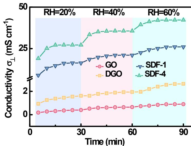
**Fig. S29.** Time-dependent vertical proton conductivities of the membranes at 80 °C.
