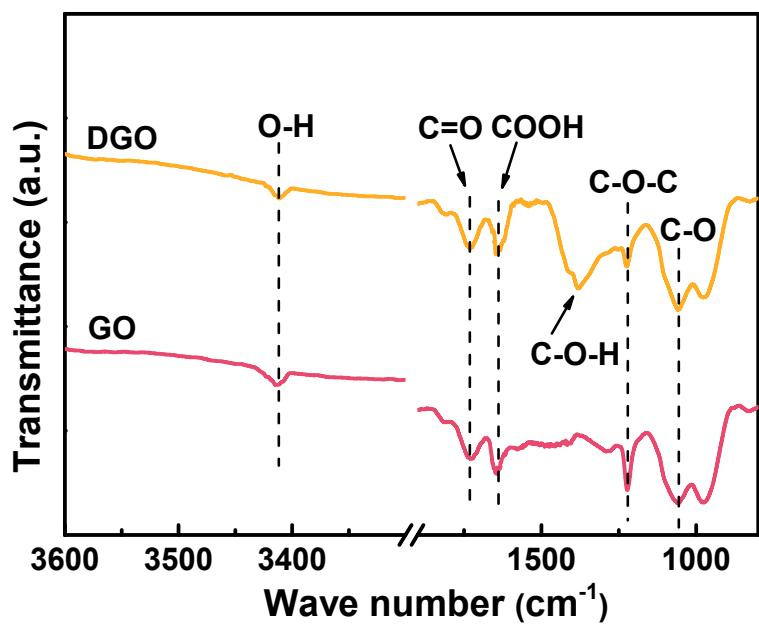
**Fig. S6.** FTIR spectra of GO and DGO nanosheets.
