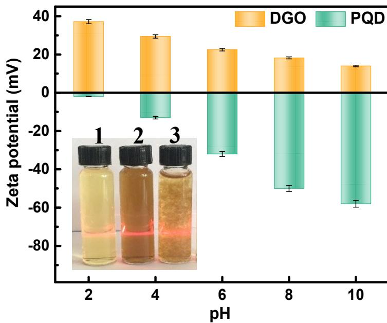
**Fig. S16.** Zeta potential of the DGO aqueous solution ( $1 \text{ g L}^{-1}$ ) and the PQD aqueous solution ( $1 \text{ g L}^{-1}$ ) with pH of 2-10 (insets are the photographs of PQD solution (1), DGO solution (2), and the mixed solution of PQD and DGO (3)).
