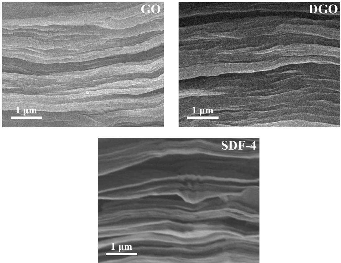
**Fig. S8.** Cross-sectional SEM images of GO, DGO, and SDF-4 membranes.
