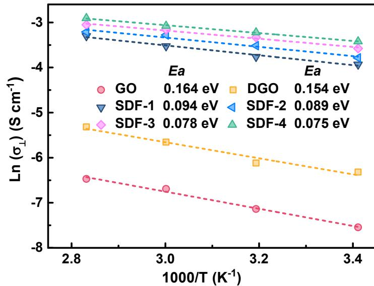
**Fig. S23.** Arrhenius plots of vertical conductivity under 100% RH and the related activation energy values.
