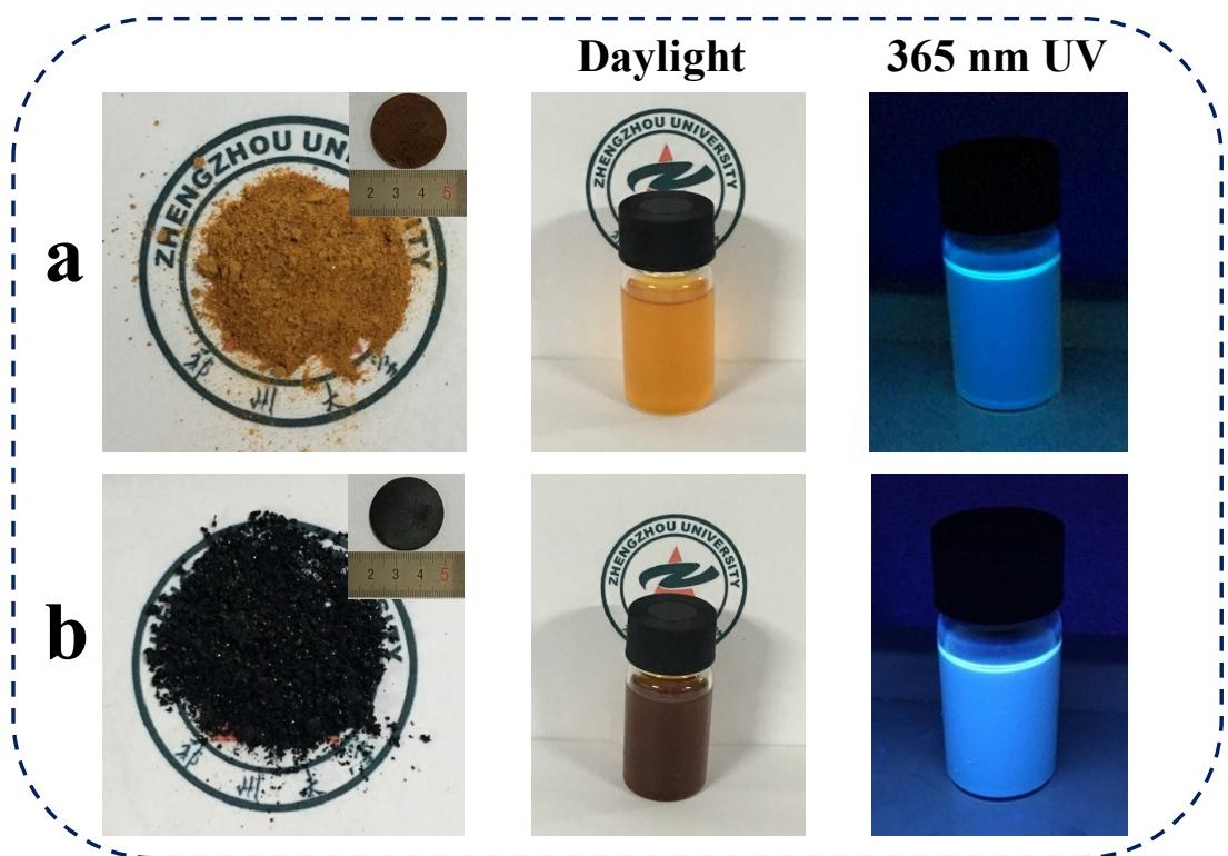
**Fig. S24.** Powders, tableting, and fluorescence effect of solution under daylight and 365 nm UV of a) PQD and b) C-PQD.
