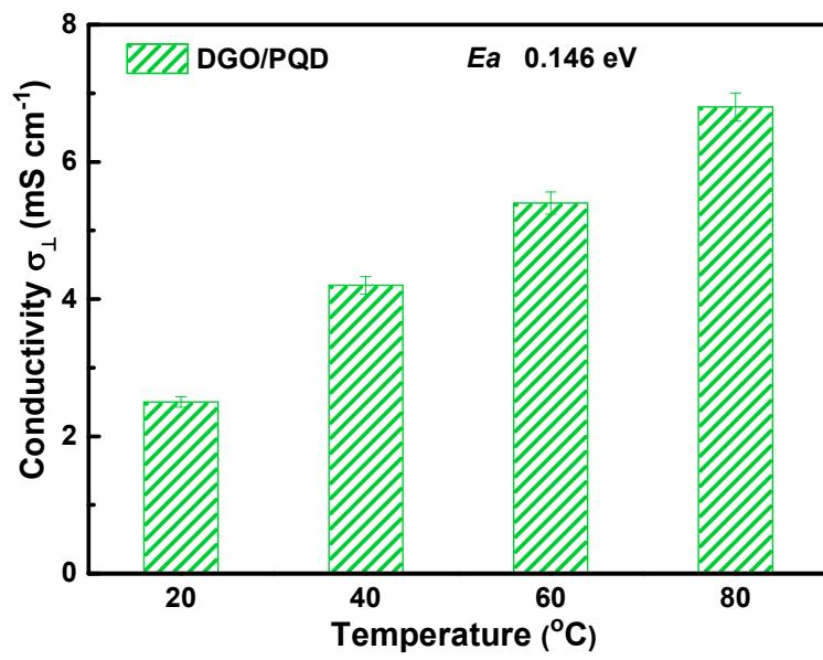
**Fig. S26.** Temperature-dependent proton conductivities of DGO/PQD membrane under 100% RH.
