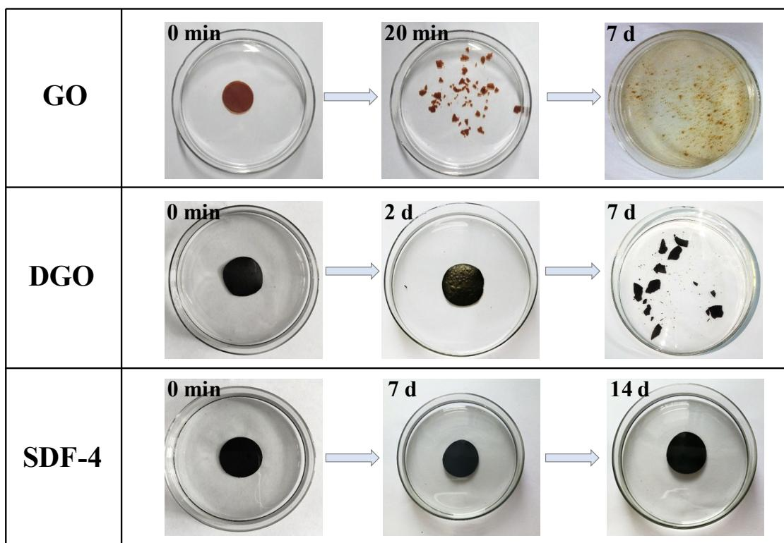
**Fig. S15.** Photos of the stability of GO, DGO, and SDF-4 membranes soaking in water at pH=7 for different time.
