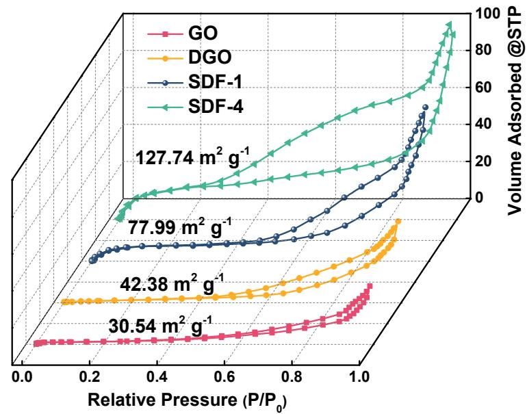
**Fig. S11.** Nitrogen adsorption/desorption isotherms and surface area of the membranes.
