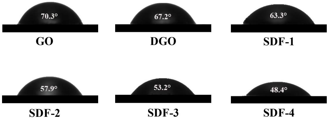
**Fig. S13.** Water contact angle of the membranes.
