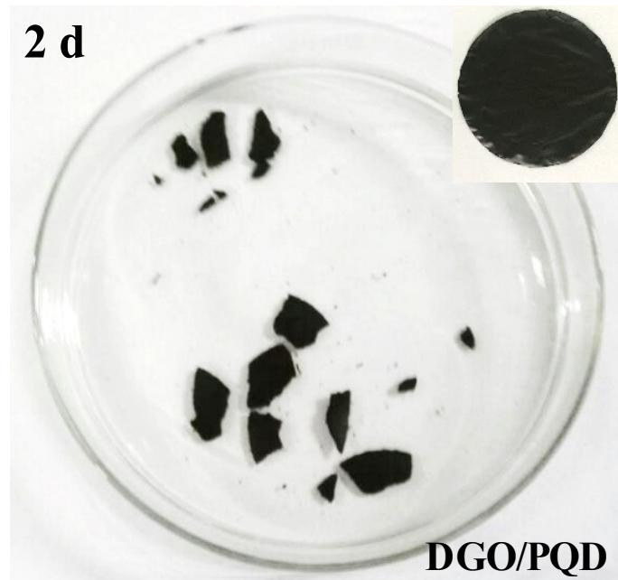
**Fig. S17.** Photo of the stability of DGO/PQD membrane soaking in water for 2 d.
