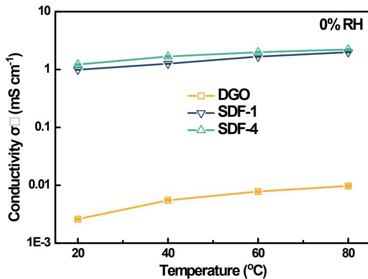
**Fig. S31.** Temperature-dependent vertical conductivities of DGO, SDF-1, and SDF-4 membranes under anhydrous conditions.
