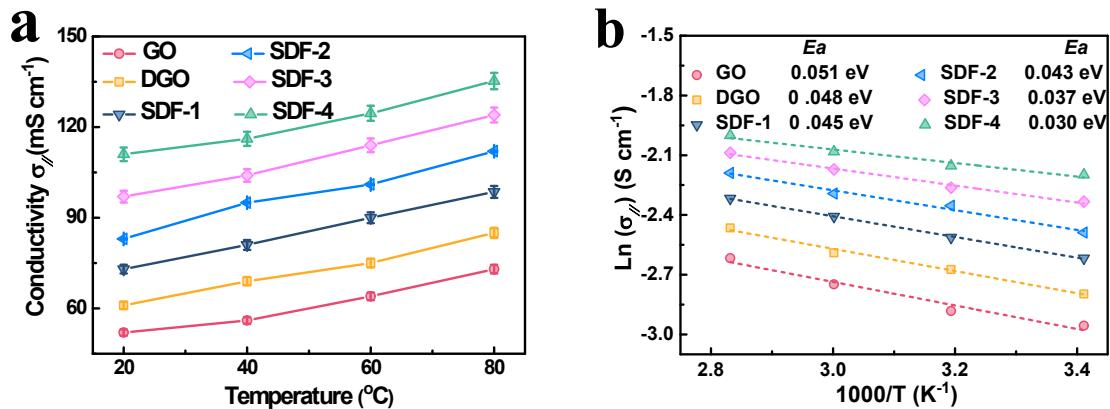
**Fig. S32.** a) Temperature-dependent horizontal conductivities of the membranes under 100% RH. b) Arrhenius plots of horizontal conductivities under 100% RH and the related activation energy values.
