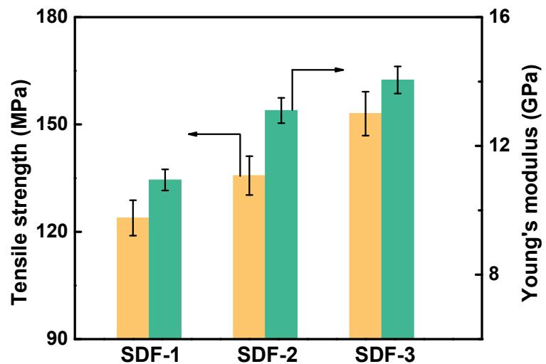
**Fig. S20.** Tensile strength and elastic modulus of SDF-1, SDF-2, and SDF-3 membranes.
