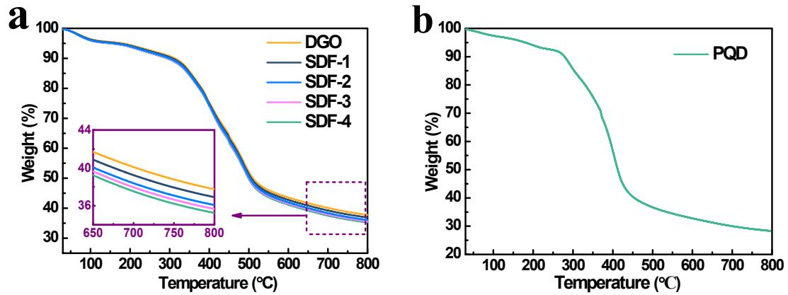
Fig. S12. TGA curves of a) membranes and b) PQD.
