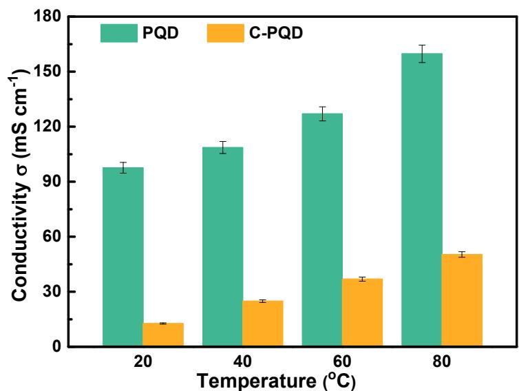
**Fig. S25.** Temperature-dependent proton conductivities of PQD and C-PQD under 100% RH.
