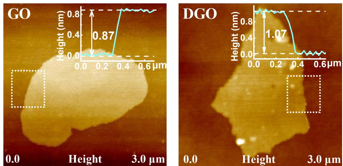
**Fig. S3.** AFM images and the corresponding height profiles of GO and DGO nanosheets.
