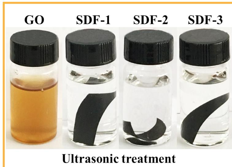
**Fig. S14.** Photos of the stability of GO, SDF-1, SDF-2, and SDF-3 membranes under ultrasonic treatment for 4 h.
