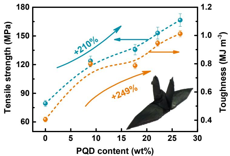
**Fig. S21.** The mechanical properties of the membranes (inset is a paper cranes folded with SDF-4 membrane).
