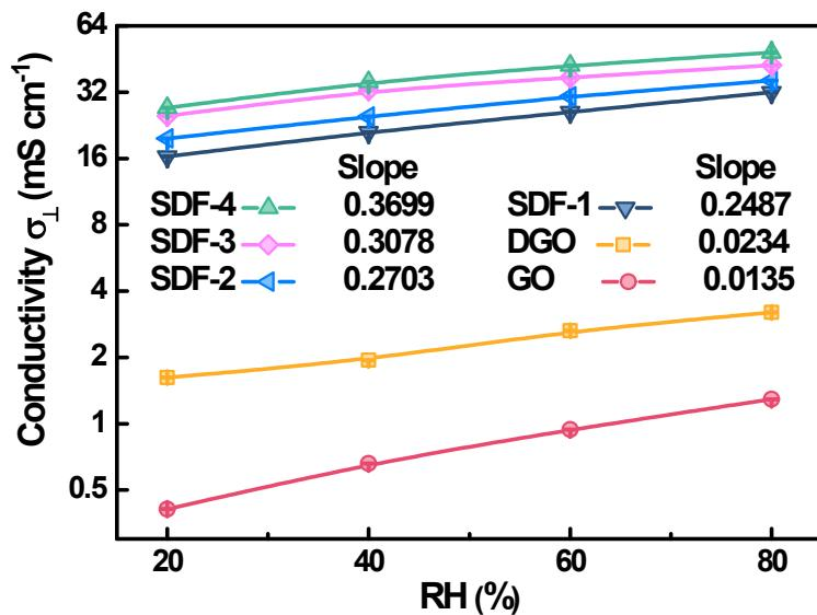
**Fig. S27.** Humidity-dependent vertical proton conductivities of the membranes at 80 °C.
