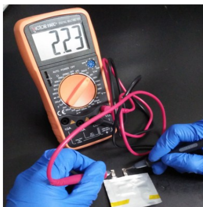
Fig. S16 Open circuit voltage of the assembled solid-state soft-package lithium metal battery at room temperature.
