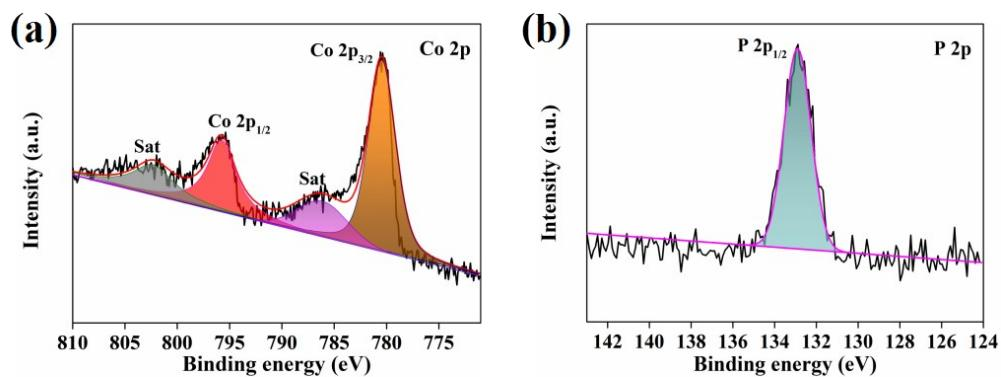
**Fig. S3** High resolution XPS spectra of (a) Co 2p, (b) P 2p from CPB.
