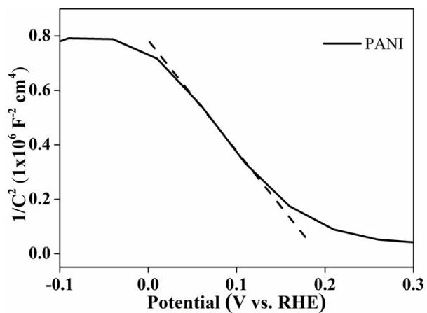
**Fig. S6** Mott-Schottky plots of PANI at a frequency of 1000 Hz and an amplitude of 10 mV.
