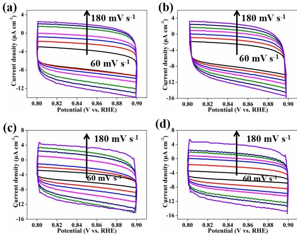
**Fig. S9** CV curves measured in a non-Faradaic region of 0.8-0.9 V at various scan rates for (a) PANI/BiVO<sub>4</sub>. (b) PANI/BiVO<sub>4</sub>-NIR. (c) CPB and (d) CPB-NIR photoanode with a geometric area of 1  $\text{cm}^2$ , respectively.
