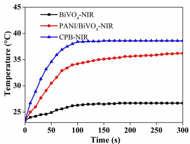
**Fig. S4** Temperature-time plots of BiVO<sub>4</sub>, PANI/BiVO<sub>4</sub> and CPB under AM 1.5G illumination with NIR light.
