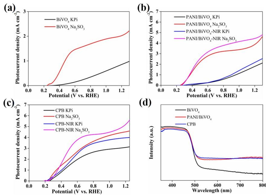
**Fig. S10** (a-c) LSV curves measured with 0.5 M KPi solution and 1M Na<sub>2</sub>SO<sub>3</sub> solution of BiVO<sub>4</sub>, PANI/BiVO<sub>4</sub> and CPB photoanodes at 1.23 V<sub>RHE</sub> with or without NIR laser and (d) UV-Vis absorptance spectra of BiVO<sub>4</sub>, PANI/BiVO<sub>4</sub> and CPB photoanodes.
