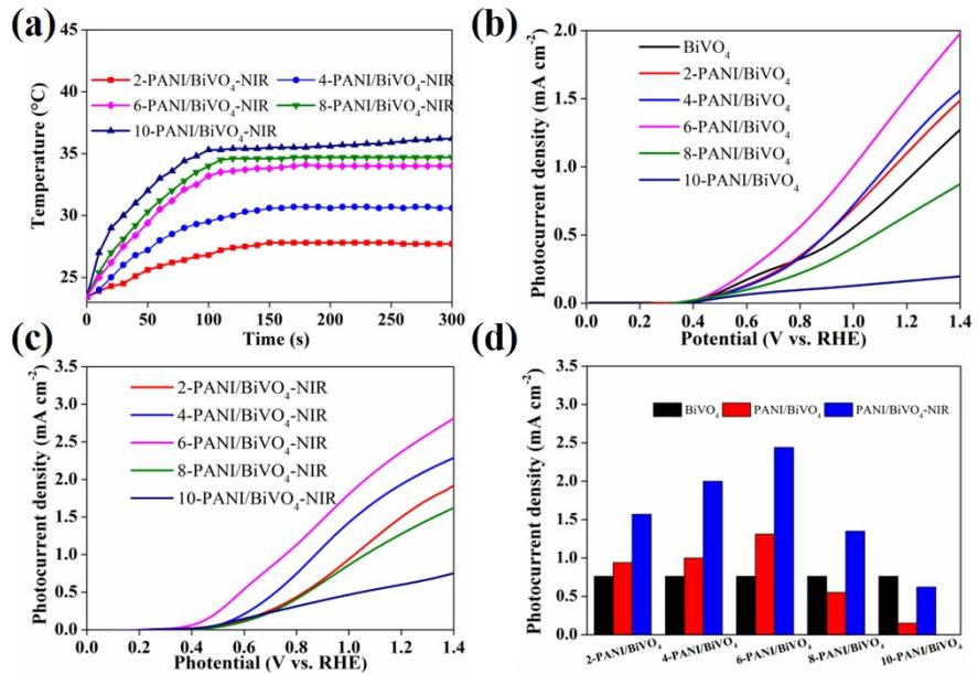
**Fig. S2** (a) Temperature-time plots under different concentrations of PANI/BiVO<sub>4</sub> photoanode with NIR. (b) LSV curves of PANI loaded with different concentrations. (c) LSV curves of NIR irradiated by PANI with different concentration. (d) Histogram of PANI loaded with different concentrations under AM 1.5G illumination with or without NIR laser.
