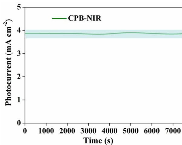
**Fig. S5** Stability of CPB-NIR at  $1.23 \text{ V}_{\text{RHE}}$  under illumination for 7500 s in 0.5 M borate buffer (pH 7).
