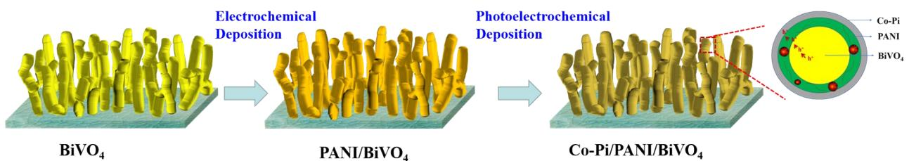
**Scheme S1** Schematic illustration of the fabrication of Co-Pi/PANI/ $\text{BiVO}_4$  (CPB) composite photoanodes.
