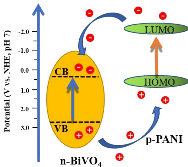
**Fig. S8** Proposed band diagram and mechanism of charge separation for PANI/BiVO<sub>4</sub> heterojunction photoanode.
