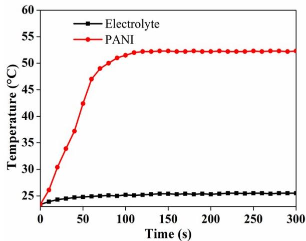
**Fig. S1** Temperature-time plots of PANI and electrolyte solution.
