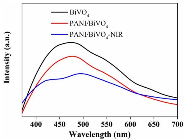
**Fig. S7** Photoluminescent spectra of  $\text{BiVO}_4$ ,  $\text{PANI}/\text{BiVO}_4$ ,  $\text{PANI}/\text{BiVO}_4$ -NIR photoanodes at the excitation wavelength of 325 nm.
