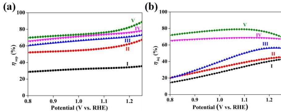
**Fig. S11** (a) Bulk ( $\eta_{\text{sep}}$ ) charge separation of BiVO<sub>4</sub>, PANI/BiVO<sub>4</sub>, PANI/BiVO<sub>4</sub>-NIR, CPB and CPB-NIR photoanodes. (b) Surface ( $\eta_{\text{inj}}$ ) charge separation of BiVO<sub>4</sub>, PANI/BiVO<sub>4</sub>, PANI/BiVO<sub>4</sub>-NIR, CPB and CPB-NIR photoanodes. I, II, III, IV, V represent BiVO<sub>4</sub>, PANI/BiVO<sub>4</sub>, PANI/BiVO<sub>4</sub>-NIR, CPB, CPB-NIR, respectively.
