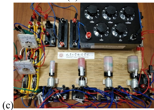
Figure S10 (a): Circuit diagram of the home-made bending machine; (b): illustration of the bending process; (c)~(d): photographs of the machine with and without connecting the circuit.
