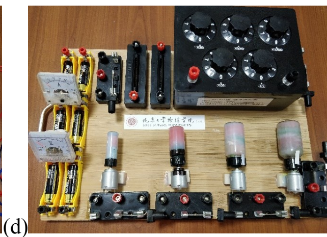
Figure S10 (a): Circuit diagram of the home-made bending machine; (b): illustration of the bending process; (c)~(d): photographs of the machine with and without connecting the circuit.
