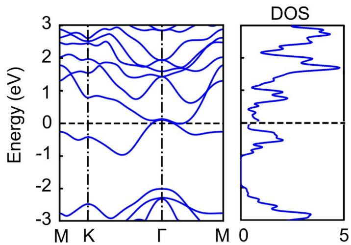
**Fig. S5.** The band structure and total electron density of states for  $\text{Ti}_2\text{CO}/\text{WS}_2$  heterostructure by using HSE06 method.
