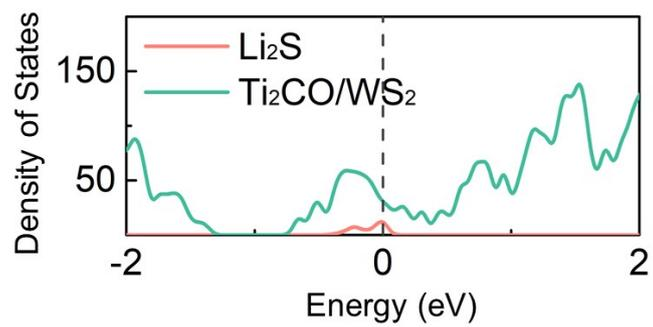
**Fig. S6.** The projected DOS of  $\text{Li}_2\text{S}$  and  $\text{Ti}_2\text{CO}/\text{WS}_2$  in  $\text{Li}_2\text{S}-\text{Ti}_2\text{CO}/\text{WS}_2$  system.
