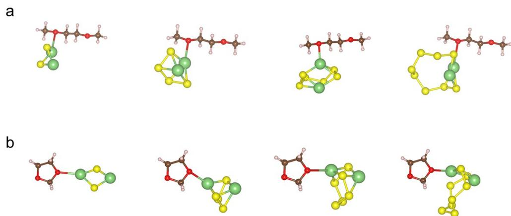
**Fig. S2.** Configurations of  $\text{Li}_2\text{S}_n$  ( $n=2,4,6,8$ ) bound with (a) DME and (b) DOL. The red, brown, white, yellow and green balls represent the oxygen, carbon, hydrogen, sulfur and lithium atom respectively.
