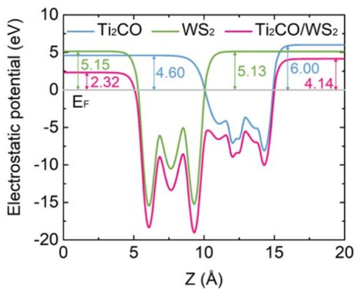
**Fig. S4.** The plane-averaged electrostatic potential of Ti<sub>2</sub>CO, WS<sub>2</sub> before contacting and Ti<sub>2</sub>CO/WS<sub>2</sub> after contacting.
