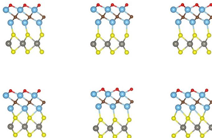
**Fig. S1.** The considered stacking patterns for the Ti<sub>2</sub>CO/WS<sub>2</sub> bilayer. The red, blue, brown, yellow and gray balls represent the oxygen, titanium, carbon, sulfur and tungsten atom respectively.
