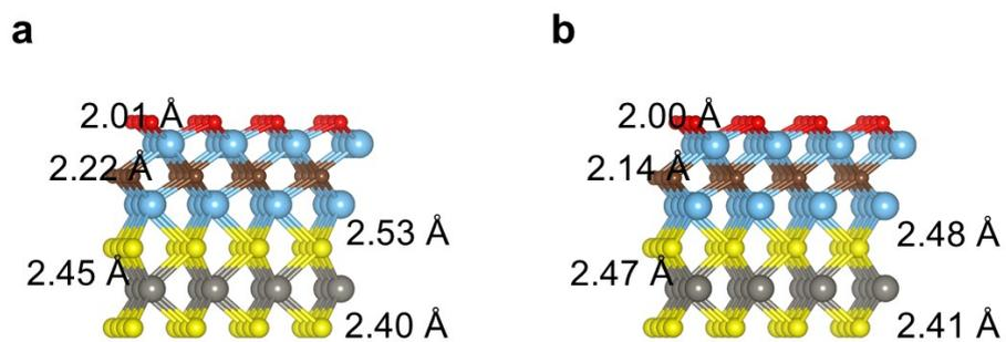
**Fig. S3.** The side views of the  $\text{Ti}_2\text{CO}/\text{WS}_2$  structure (a) before and (b) after AIMD runs for 5 ps. All atoms are displacing slightly near their equilibrium positions during the simulations and no structural reconstruction occurs at 298 K.
