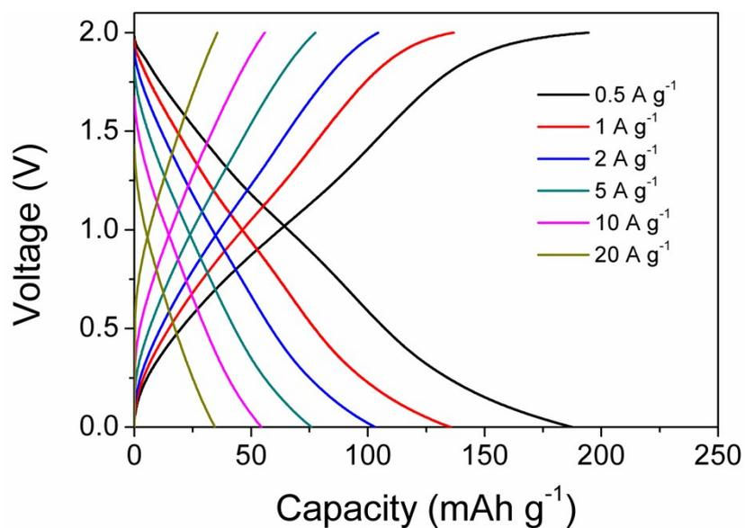
Fig. S4 The GCD curves at different current densities from 0.5 to 20 A g<sup>-1</sup> by testing the water-in-salt zinc-ion hybrid supercapacitor assembled with nonwoven cloth.
