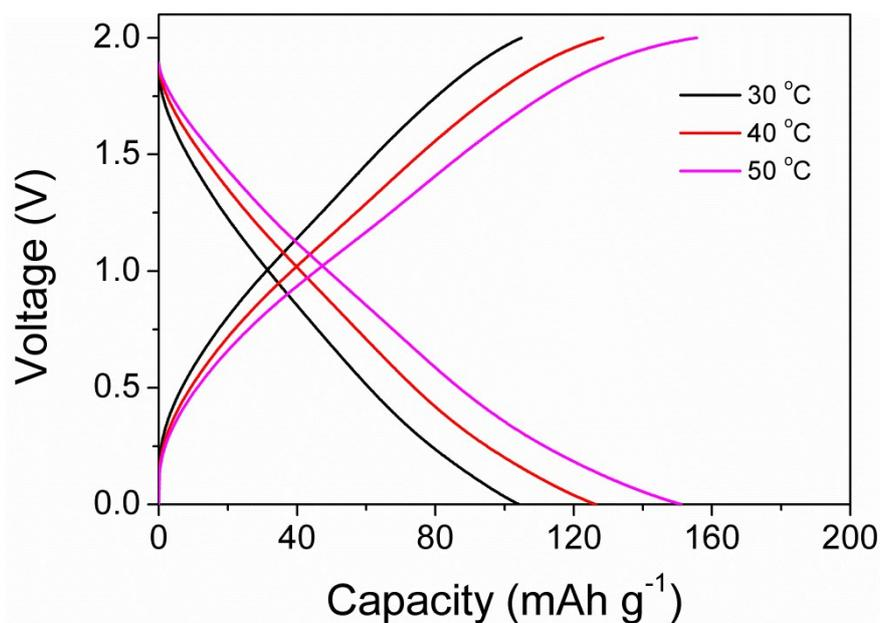
Fig. S10 GCD curves under the temperatures of 30, 40 and 50 °C at the current density of 5 A g<sup>-1</sup>.
