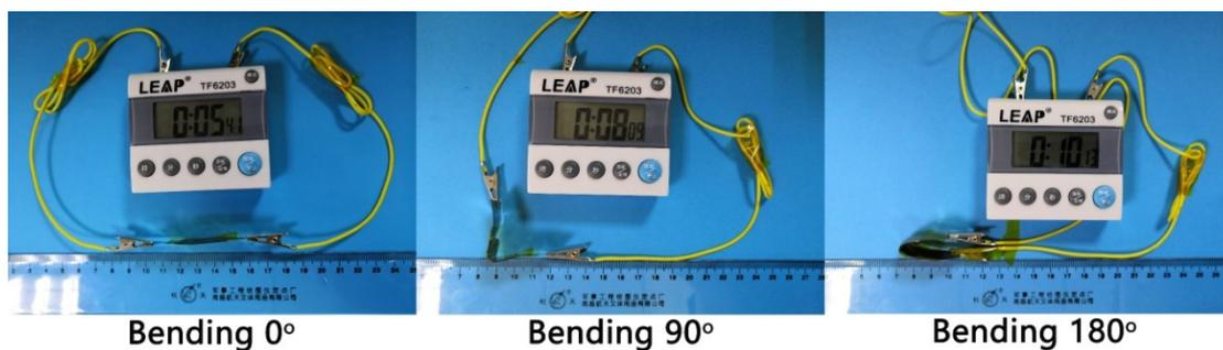
Fig. S9 The flexibility of zinc-ion hybrid supercapacitor assembled by the cellulose hydrogel electrolyte.
