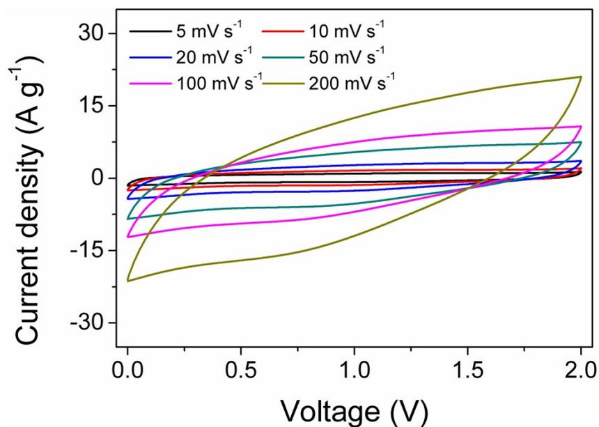
Fig. S6 The CV curves at different scan rates under a low temperature of  $-20\text{ }^{\circ}\text{C}$  by testing zinc-ion hybrid supercapacitor assembled with cellulose hydrogel electrolyte.
