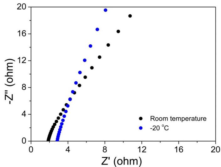
Fig. S2 The nyquist plot tested by sandwiching the cellulose hydrogel between two stainless steel sheets. The size of hydrogel is  $0.2 \times 1 \times 1.5 \text{ cm}^3$  (thickness $\times$ width $\times$ length)
