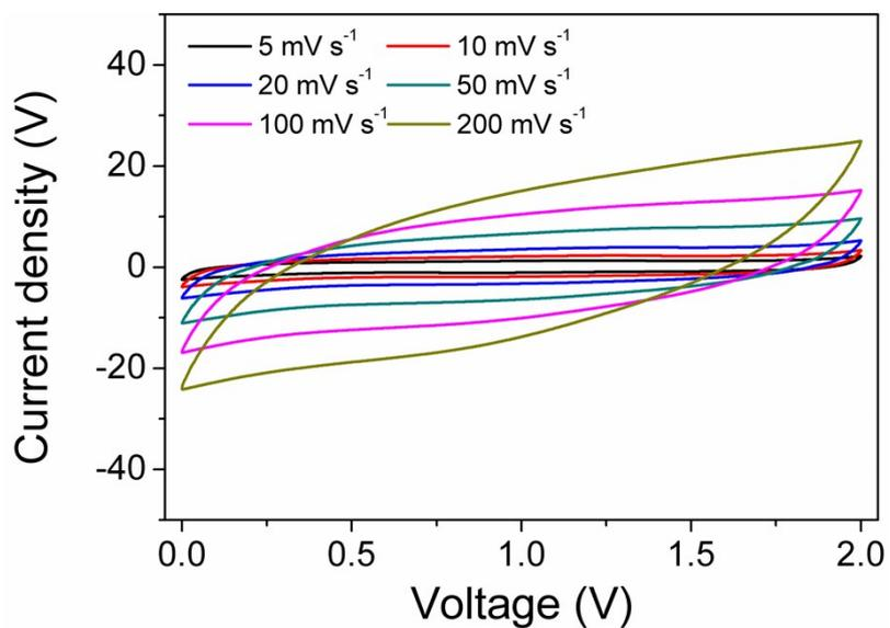
Fig. S3 The CV curves at different scan rates from 5 to 200  $\text{mV s}^{-1}$  by testing the water-in-salt zinc-ion hybrid supercapacitor assembled with nonwoven cloth.
