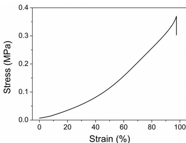
Fig. S1 Tensile stress–strain curve of the cellulose hydrogel.
