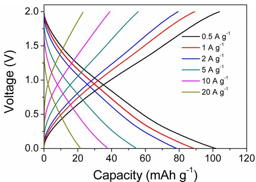
Fig. S7 The GCD curves at different current densities under a low temperature of  $-20\text{ }^{\circ}\text{C}$  by testing zinc-ion hybrid supercapacitor assembled with cellulose hydrogel electrolyte. The coulombic efficiency is in the range of 94.0 - 99.8% at  $-20\text{ }^{\circ}\text{C}$ .
