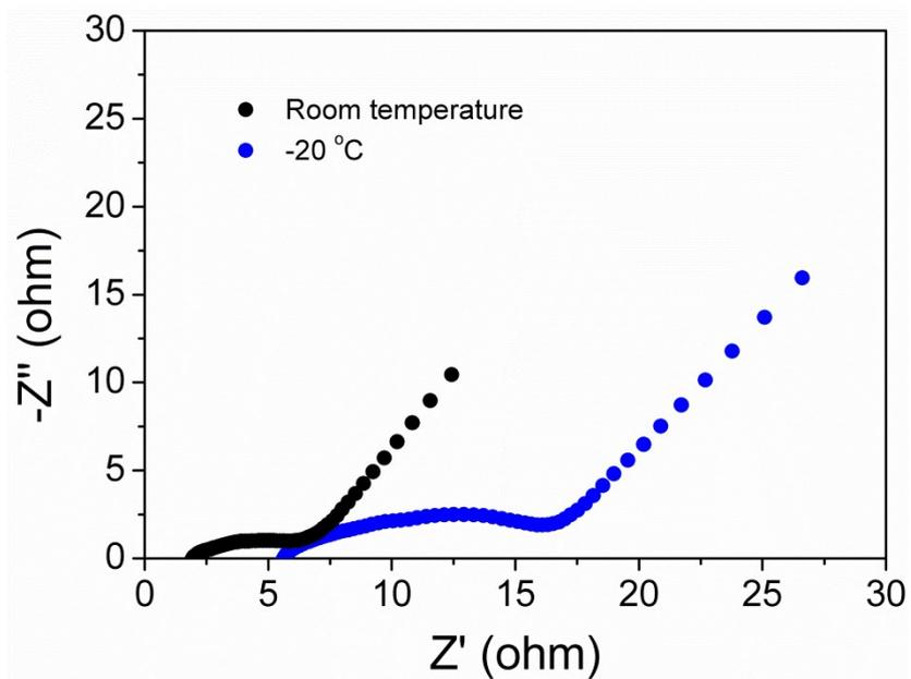
Fig. S8 The nyquist plots at the room temperature and  $-20\text{ }^{\circ}\text{C}$  by testing zinc-ion hybrid supercapacitor assembled with cellulose hydrogel electrolyte.
