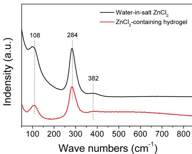
Fig. S5 Raman spectra of ZnCl<sub>2</sub> solution (1.75 g/g ZnCl<sub>2</sub>/H<sub>2</sub>O) and the cellulose hydrogel at the same ZnCl<sub>2</sub> concentration.
