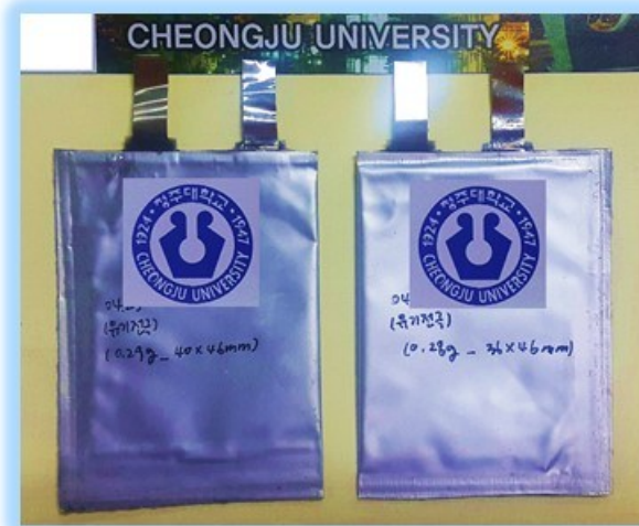
Figure S9. Photo image of the assembled organic sodium full-cell.
