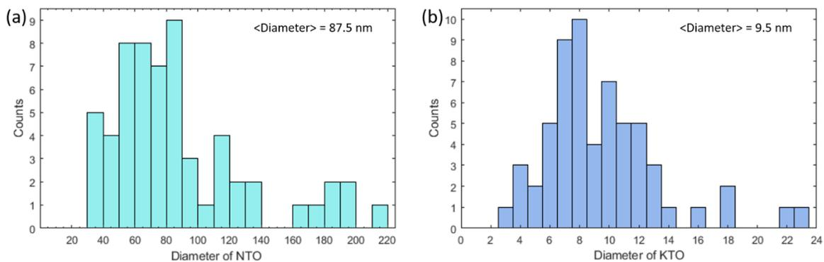
**Figure S10.** Statistic diameter distributions of (a) NTO nanobelts and (b) KTO nanowires, taken from 60 nanosheets or nanowires, respectively.
