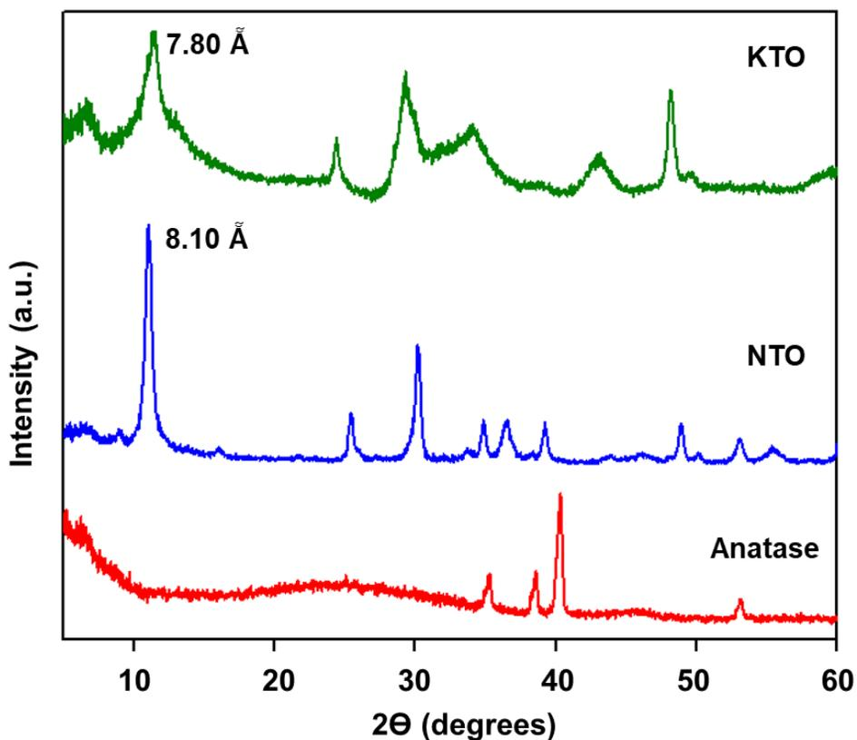
**Figure S5.** XRD patterns of the layered titanates after hydrothermal treatment at 220 °C for 24 h. Characteristic XRD patterns exhibit the layered structure of the NTO and KTO samples. However, anatase is obtained (red line) instead of the layered LTO sample.
