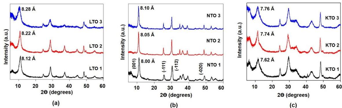
**Figure S8. XRD patterns of layered titanates.** Characteristic XRD patterns of the Li, Na and K based layered titanates with the prominent peaks indexed, and demonstrating the typical layered structure. Also, the variation in interlayer spacing can be seen, which can be attributed to varying amounts of interlayer water.
