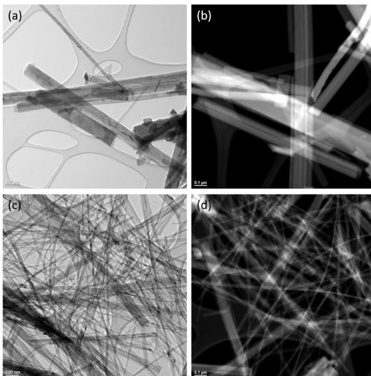
**Figure S9.** (a) Bright-field TEM and (b) annular dark field scanning TEM (ADF-STEM) imaging of NTO nanobelts. (c) Bright-field TEM and (d) ADF-STEM imaging of KTO nanowires.
