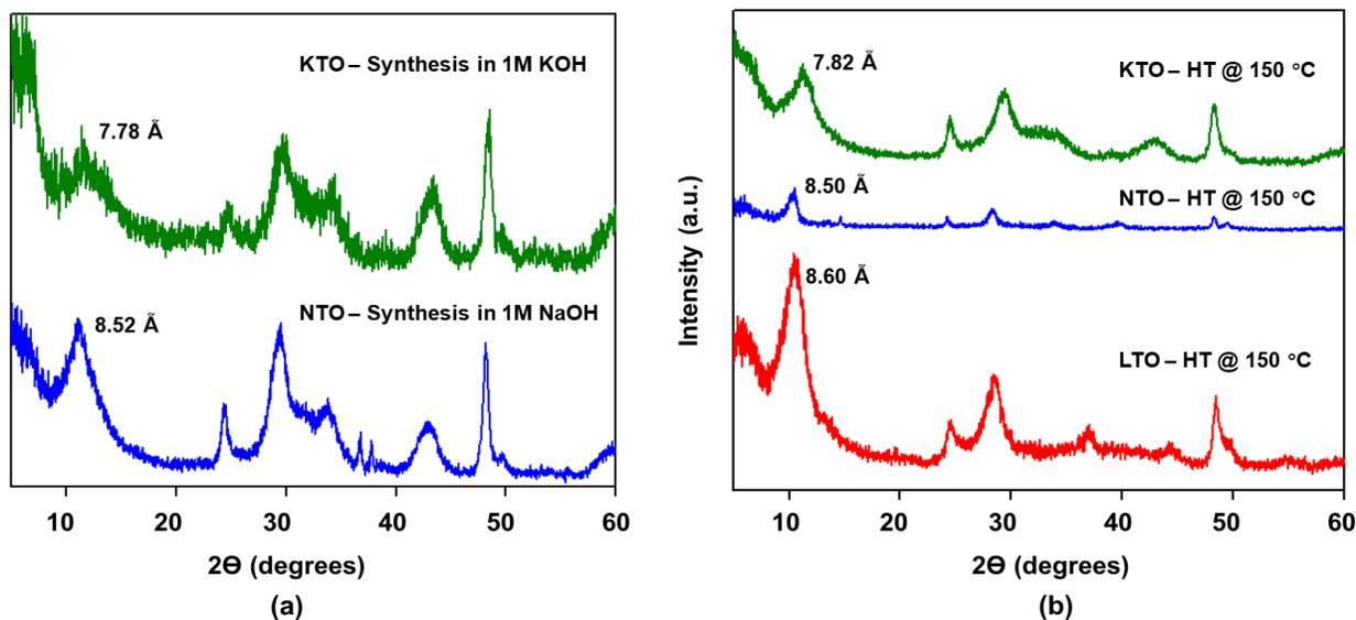
**Figure S6. Adaptation of the synthesis conditions found for the LTO sample to the preparation of the NTO and KTO phases.** (a) XRD patterns indicating the weak lamellar ordering and low crystallinity for NTO and KTO samples synthesized with a starting 1M concentration of the corresponding base, (b) low crystallinity observed in the XRD patterns of the NTO and KTO samples synthesized at HT conditions of 150 °C, as opposed to the highly crystalline LTO sample.
