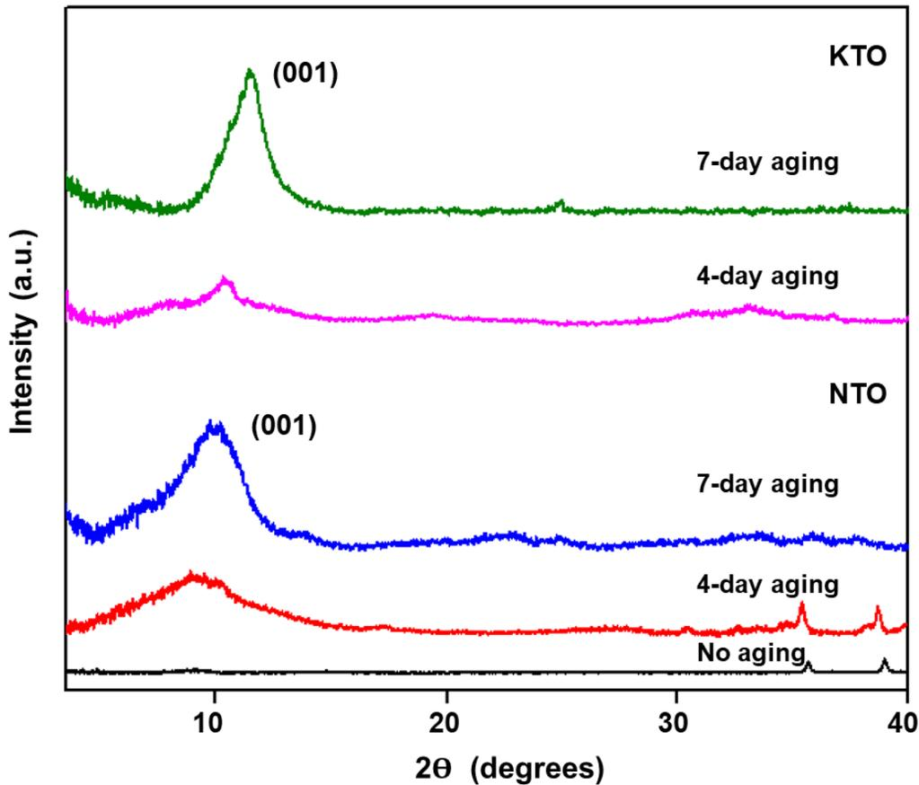
**Figure S3. The role of aging in the development of lamellar ordering.** XRD patterns of the NTO and KTO samples demonstrating the gradual evolution of the lamellar ordering, as the (001) peak grows in intensity with longer aging time.
