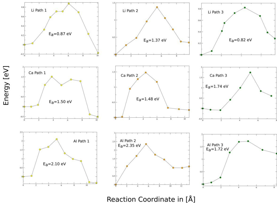
Figure S3: Minimum energy paths (MEP) demonstrating activation barriers for Li, Ca and Al migrating along pathways 1, 2 and 3, yellow, orange and green colours, respectively. Activation barriers are displayed for each case as  $E_a$  in eV.
