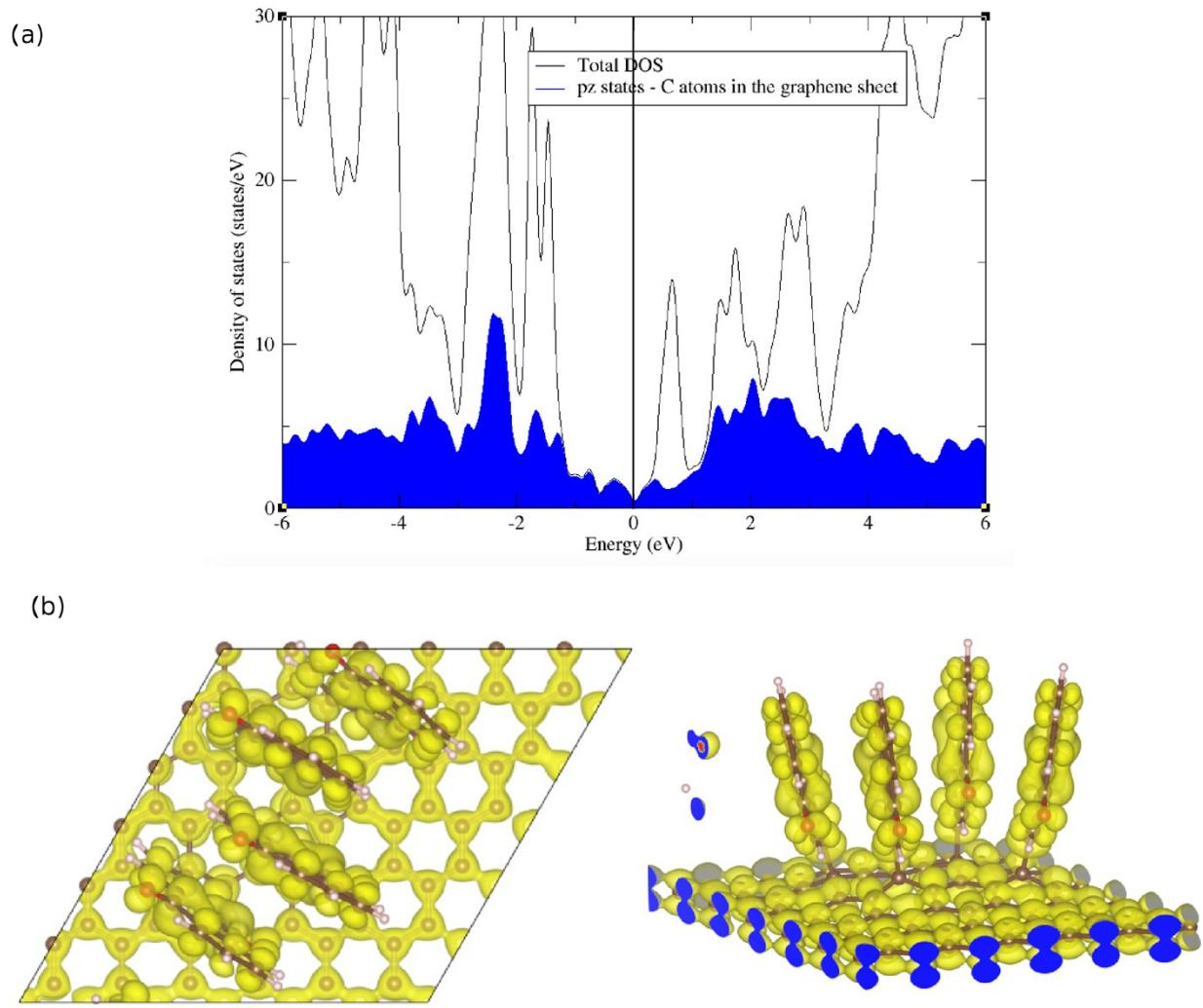
Figure S2: (a) Total and partial density of states (DOS and pDOS) of  $\text{AQ}_4\text{C}_{72}$ . Field colored blue is the summed density of states of the  $2p_z$  AOs of the carbons in the sheet (Fermi energy was set to zero). (b) Top and side view of the partial charge density for states close to the Fermi level (isosurface value is  $0.008 \text{ e}/\text{\AA}^3$ ).
