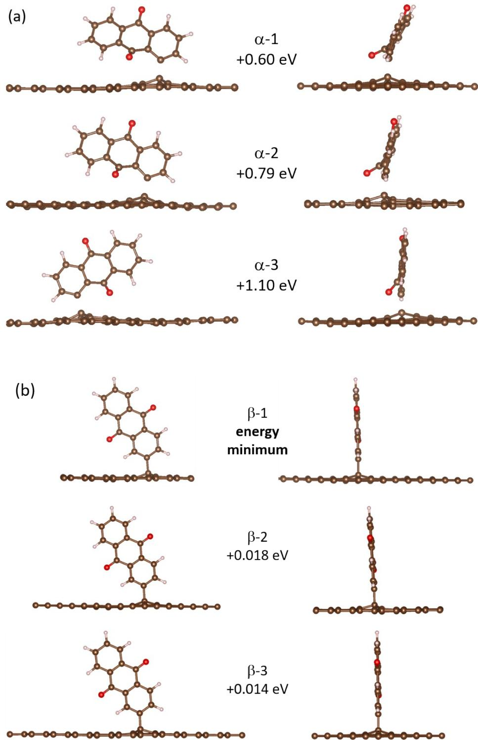
Figure S1. Optimized geometries and relative energies of the functionalized graphene with the anthraquinone residue attached at alpha (a.) and beta (b.) position. The connecting bond in a. is longer than 1.6 Å and therefore is not visualized. A PAW energy cut-off of 350 eV were used for the optimizations.
