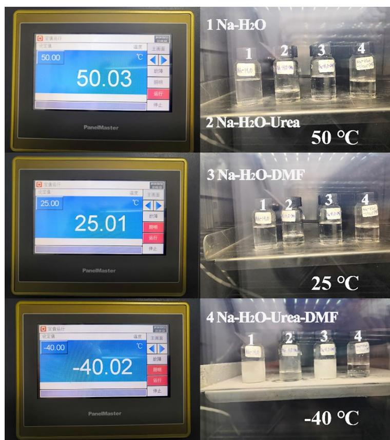
**Figure S3.** The digital photograph of state of different electrolytes at 50°C, 25°C and -40°C.
