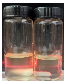
Fig. S4. Tyndall effect. (left)The solution added 1g PEG and (right) initial PAN solution.
