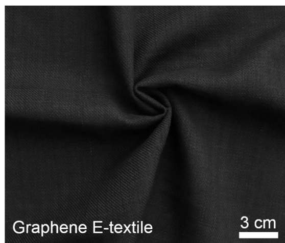
Fig. S13 Optical image of graphene E-textile, the same flexibility as original textiles.
