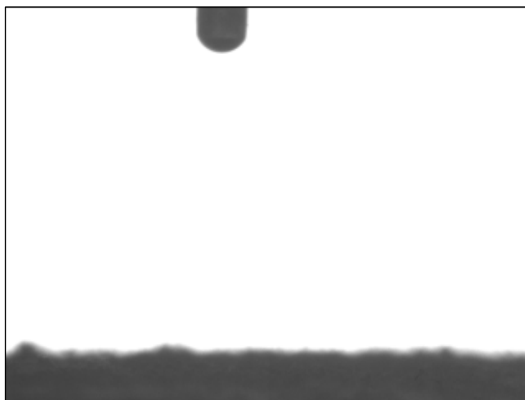
Fig. 14 Measurement of water CA of the shell of the silicone/MWCNTs evaporator after being soaked in 3.5 wt% NaCl solution for 30 d.
