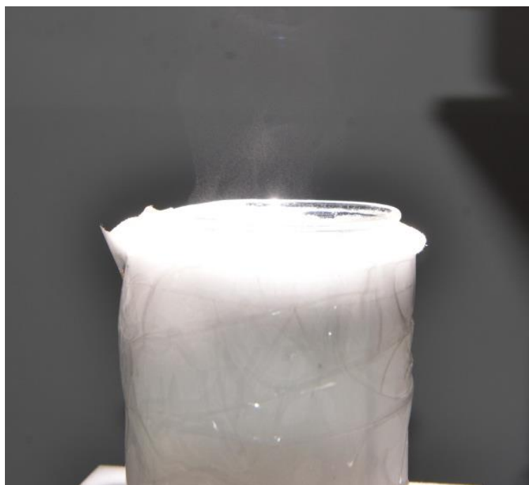
Fig. S7 Photograph of water vapor generated by the silicone/MWCNTs evaporator under 2 sun.
