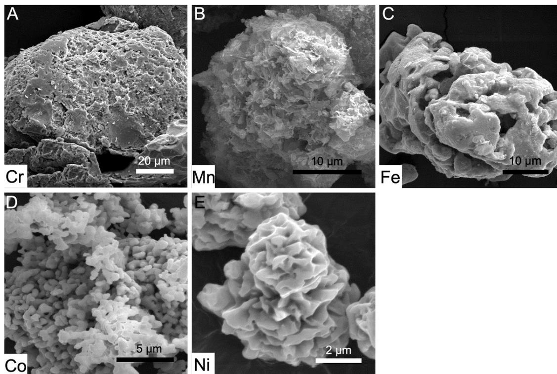
**Figure S6.** SEM images of porous Cr, Mn, Fe, Co and Ni, respectively.
