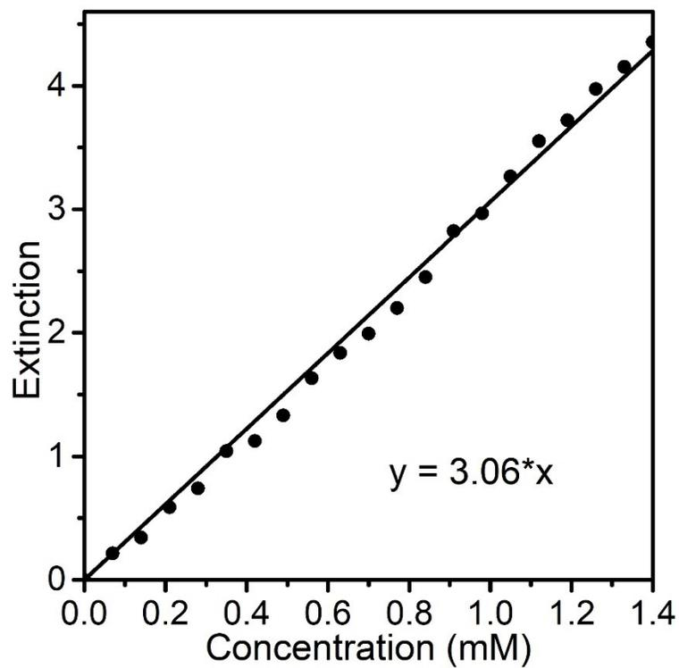
**Figure S5.** The extinction at 400 nm of a series of p-nitrophenol solution with distinct concentrations.
