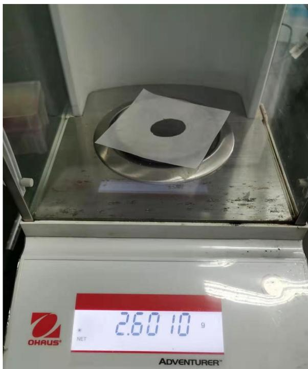
**Figure S2.** Large-scale production of CMFCN-4 powders obtained by etching 20 g of CMFCN-0.
