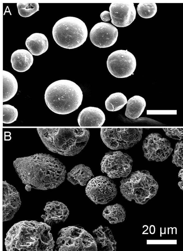
**Figure S1.** (A, B) SEM images of CMFCN-0 and CMFCN-4, respectively. All bars represent 20  $\mu\text{m}$ .
