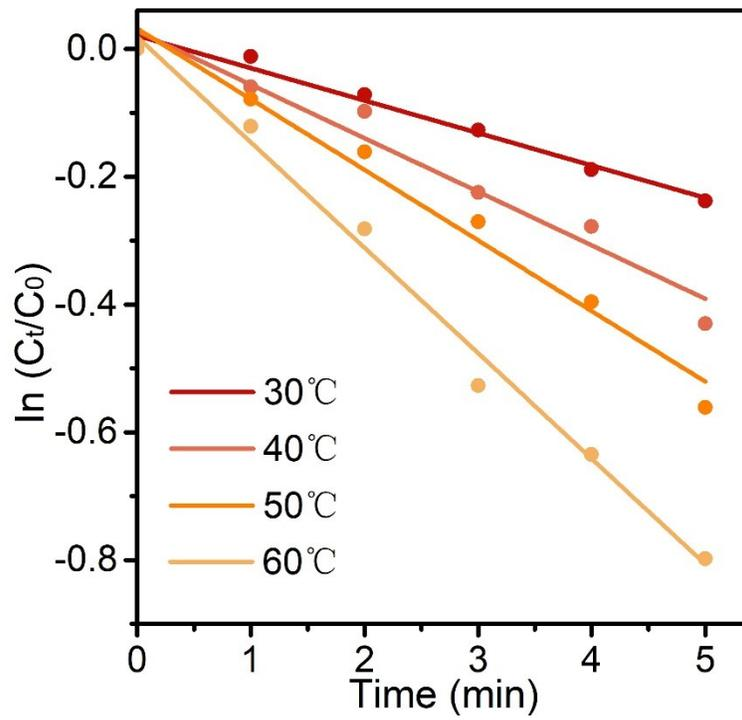
**Figure S8.** Plots of  $\ln (C_t/C_0)$  versus time catalyzed by CMFCN-4 at different temperatures.
