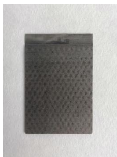
Figure S5. The photo profile of the Ni(OH) 2 electrode (3 * 4 cm 2 )
