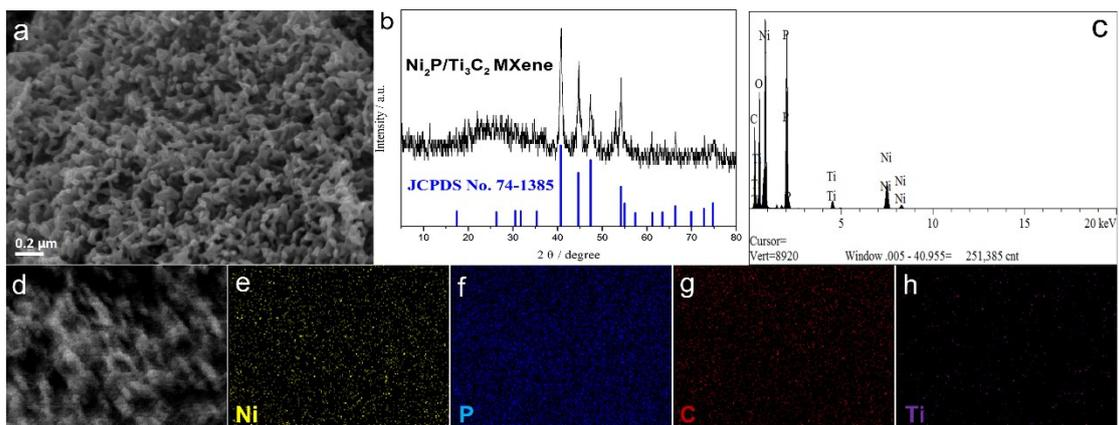
**Figure S19.** (a) SEM image, (b) XRD patterns, (c) EDX spectrum, and (d-h) Elemental mapping of Ni<sub>2</sub>P/Ti<sub>3</sub>C<sub>2</sub> MXene.
