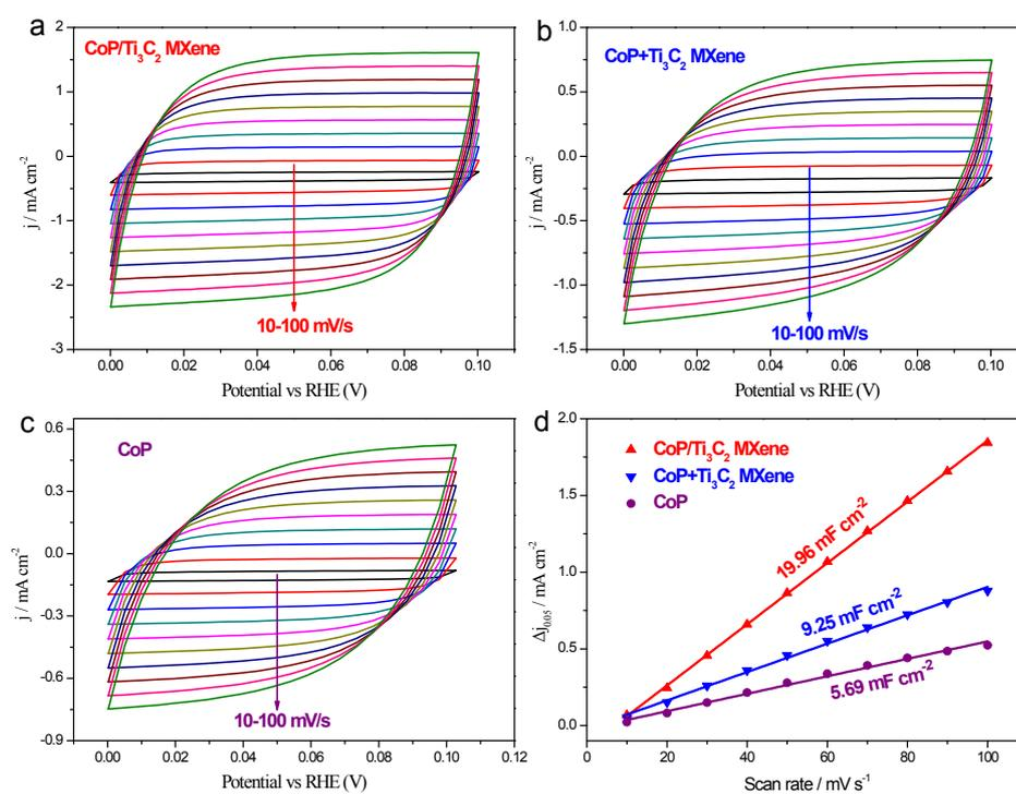
**Figure S5.** Cyclic voltammograms (CV) curves of (a) CoP/Ti<sub>3</sub>C<sub>2</sub> MXene, (b) CoP+Ti<sub>3</sub>C<sub>2</sub> MXene, and (c) MXene-free CoP in the region of 0-0.10 V in 1.0 M KOH at various scan rates. (d) Plots of current density differences ( $\Delta j$ ) against scan rates of the three catalysts at 0.05 V, where  $\Delta j$  is the difference between anodic and cathodic current densities in CV curves at different scan rates.
