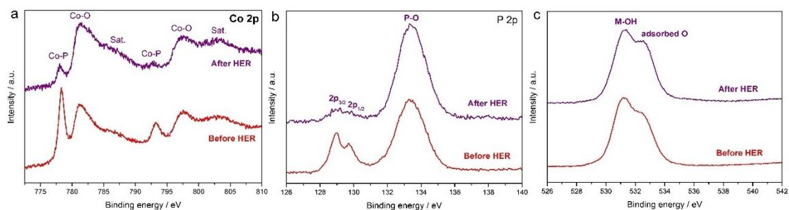
**Figure S13.** XPS spectra of (a) Co 2p, (b) P 2p, and (c) O 1s of the CoP/Ti<sub>3</sub>C<sub>2</sub> MXene before and after HER test in 1.0 M KOH.
