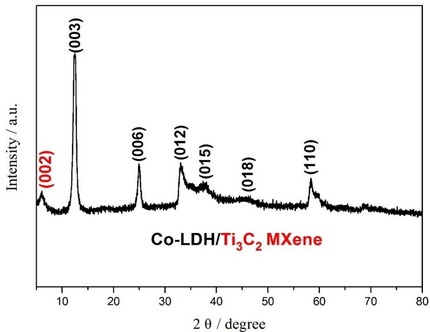
**Figure S1.** XRD patterns of Co-LDH/Ti<sub>3</sub>C<sub>2</sub> MXene.
