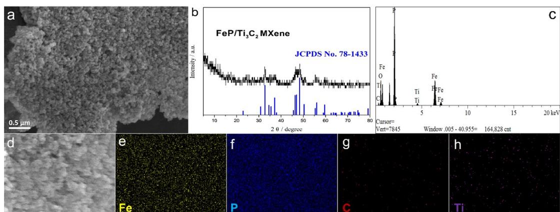
**Figure S20.** (a) SEM image, (b) XRD patterns, (c) EDX spectrum, and (d-h) Elemental mapping of FeP/Ti<sub>3</sub>C<sub>2</sub> MXene.
