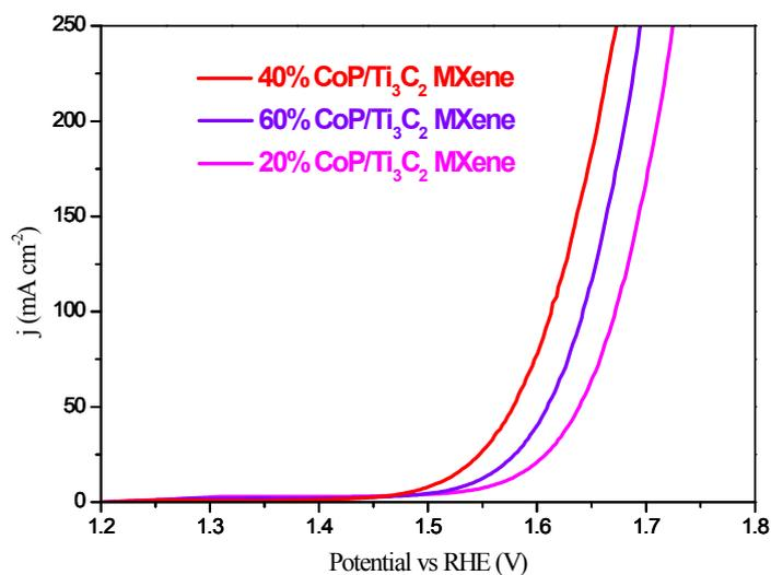
**Figure S7.** OER polarization curves of CoP/Ti<sub>3</sub>C<sub>2</sub> MXene catalysts with varied CoP content measured in 1.0 M KOH.
