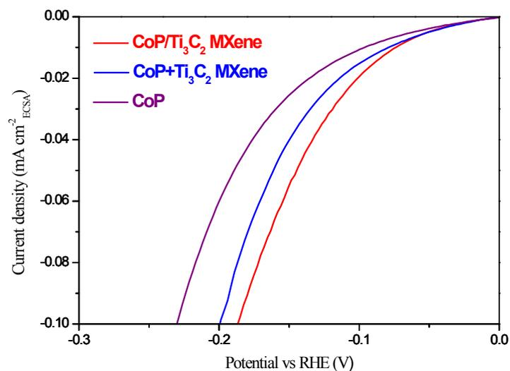
**Figure S6.** The LSV curves of samples normalized to the ECSA.
