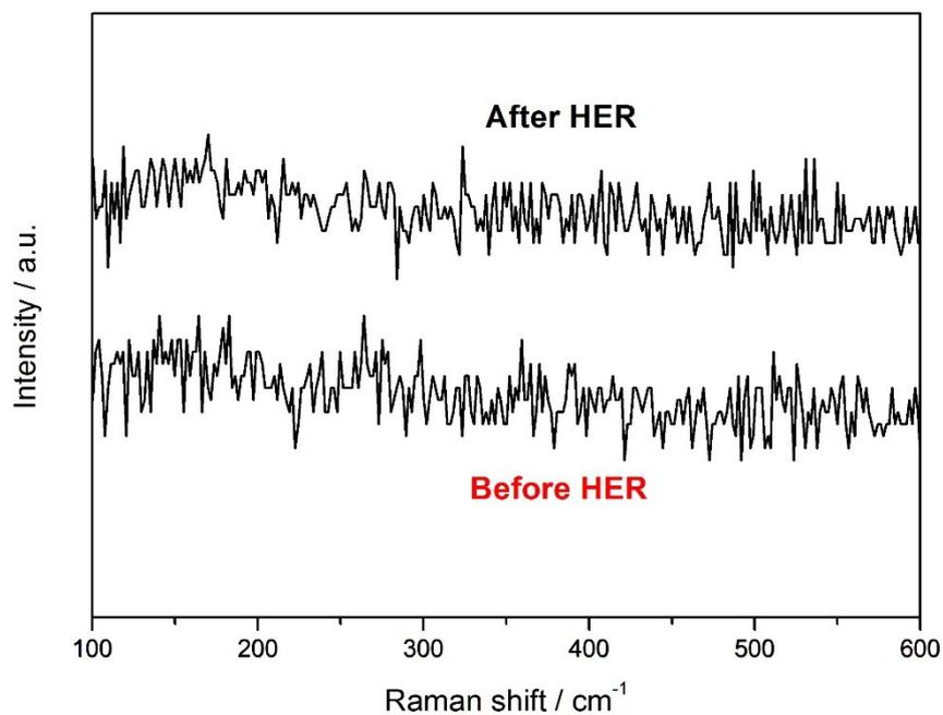
**Figure S16.** Raman spectrum of CoP/Ti<sub>3</sub>C<sub>2</sub> MXene before and after HER test in 1.0 M KOH.
