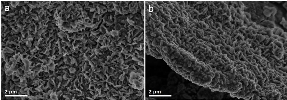
**Figure S18.** SEM images of CoP/Ti<sub>3</sub>C<sub>2</sub> MXene after (a) HER and (b) OER stability test.
