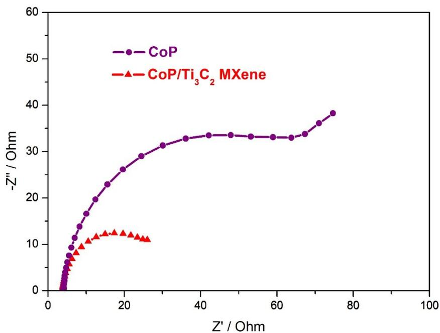
**Figure S8.** Nyquist plots of the CoP/Ti<sub>3</sub>C<sub>2</sub> MXene and MXene-free CoP for OER.
