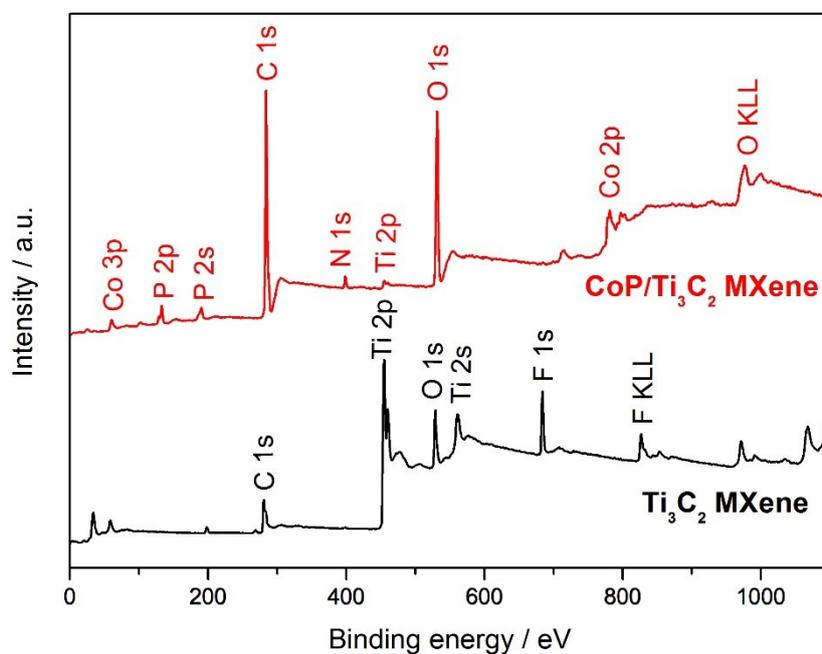
**Figure S2.** XPS survey spectra of CoP/Ti<sub>3</sub>C<sub>2</sub> MXene and Ti<sub>3</sub>C<sub>2</sub> MXene.
