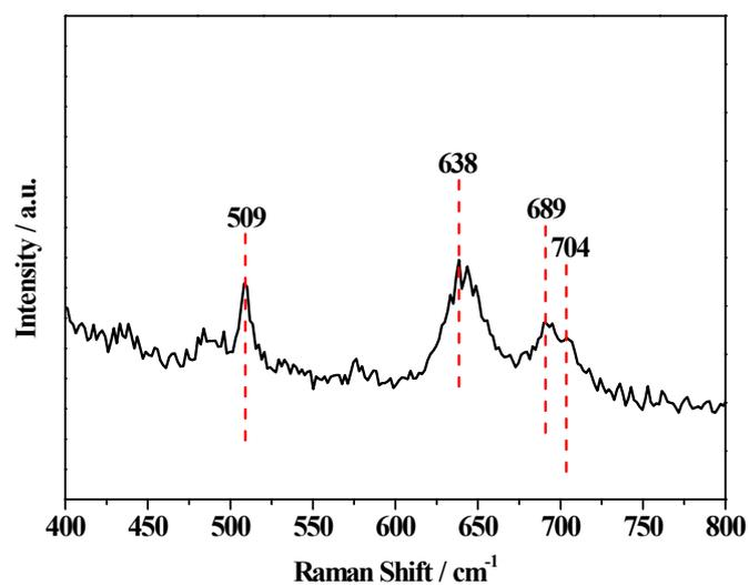
**Figure S12.** Raman spectra of CoP/Ti<sub>3</sub>C<sub>2</sub> MXene after OER test.
