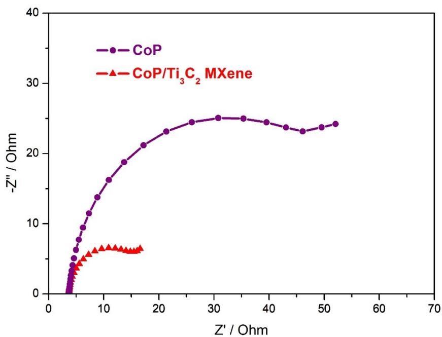
**Figure S4.** Nyquist plots of the CoP/Ti<sub>3</sub>C<sub>2</sub> MXene and MXene-free CoP for HER.
