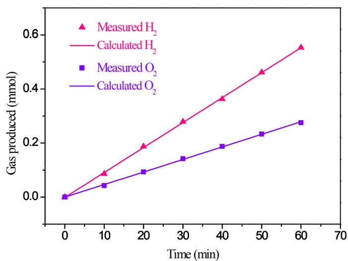
**Figure S17.** The amount of gas theoretically calculated and experimentally measured versus time for overall water splitting of CoP/Ti<sub>3</sub>C<sub>2</sub> MXene.
