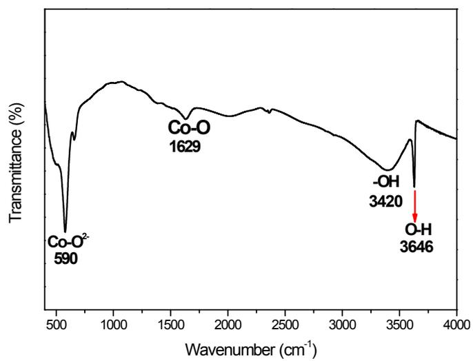
**Figure S11.** FTIR spectrum of CoP/Ti<sub>3</sub>C<sub>2</sub> MXene after OER test.
