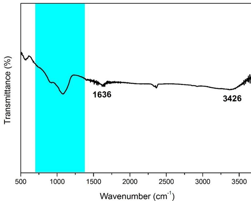
**Figure S15.** FTIR spectrum of CoP/Ti<sub>3</sub>C<sub>2</sub> MXene after HER test in 1.0 M KOH.
