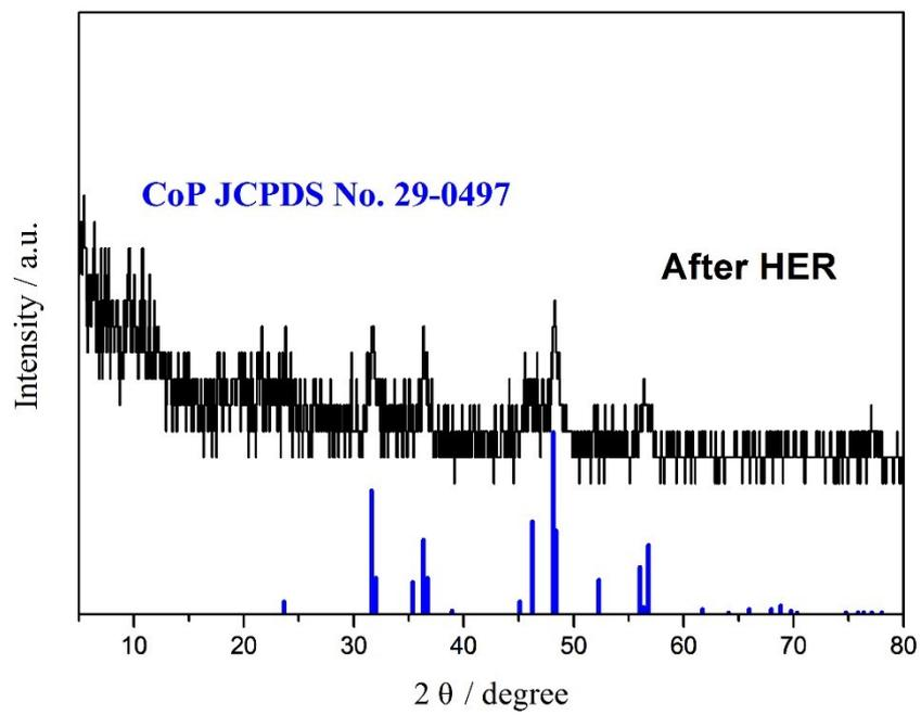
**Figure S14.** XRD patterns of CoP/Ti<sub>3</sub>C<sub>2</sub> MXene after HER test in 1.0 M KOH.
