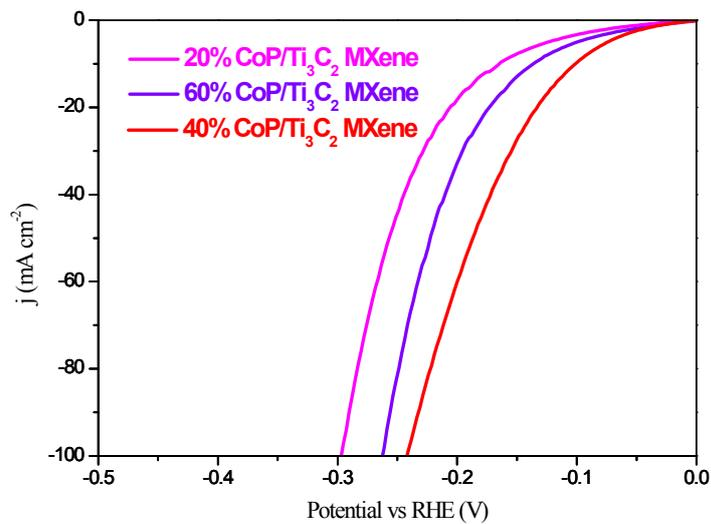
**Figure S3.** HER polarization curves of CoP/Ti<sub>3</sub>C<sub>2</sub> MXene catalysts with varied CoP content measured in 1.0 M KOH.
