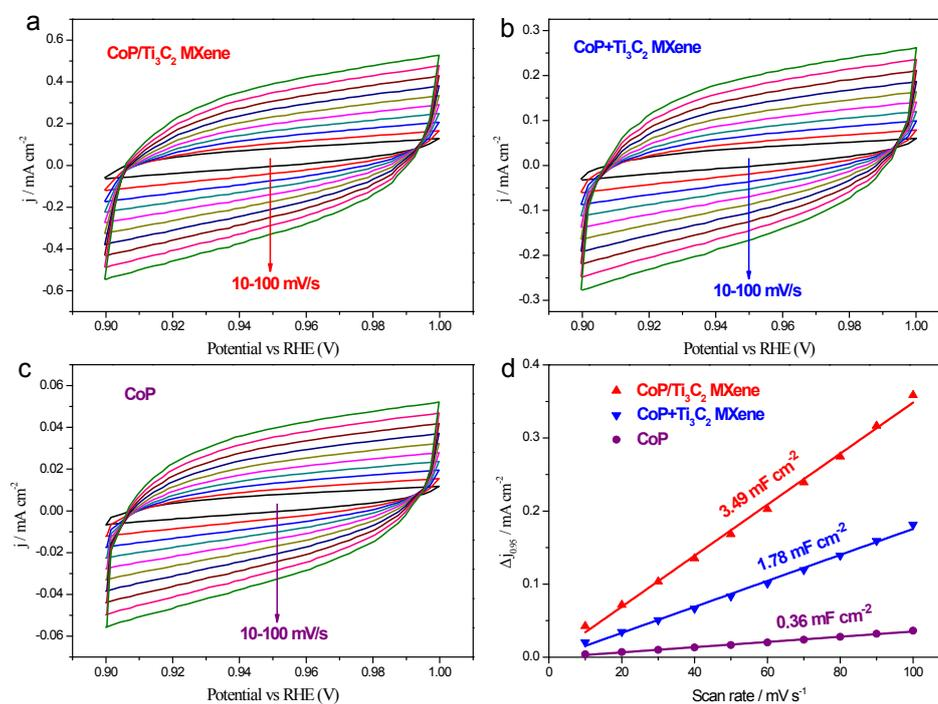
**Figure S9.** Cyclic voltammograms (CV) curves of (a) CoP/Ti<sub>3</sub>C<sub>2</sub> MXene, (b) CoP+Ti<sub>3</sub>C<sub>2</sub> MXene, and (c) MXene-free CoP in the region of 0.9-1.0 V in 1.0 M KOH at various scan rates. (d) Plots of current density differences ( $\Delta j$ ) against scan rates of the three catalysts at 0.95 V, where  $\Delta j$  is the difference between anodic and cathodic current densities in CV curves at different scan rates.
