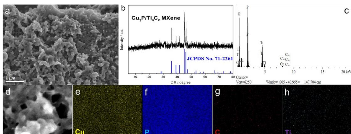
**Figure S21.** (a) SEM image, (b) XRD patterns, (c) EDX spectrum, and (d-h) Elemental mapping of Cu<sub>3</sub>P/Ti<sub>3</sub>C<sub>2</sub> MXene.
