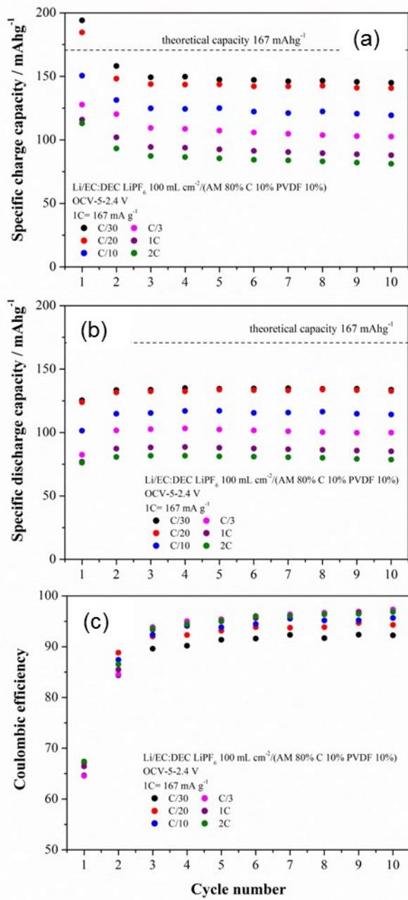
**Figure S5.** (a) Charge and (b) discharge specific capacity for the LCFMP@C electrodes at various current rates and (c) the corresponding Coulombic efficiencies. The specific capacity are normalized by the mass of the active material in the electrode, also including the ~7% of the carbon coating.
