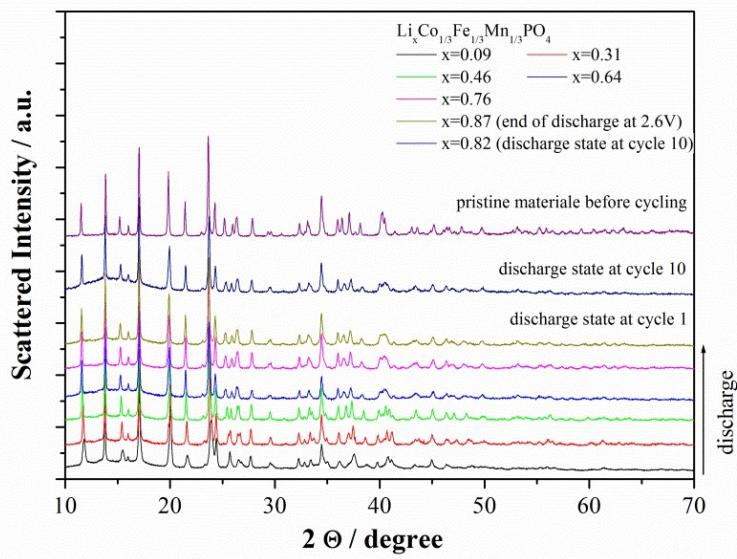
**Figure S8.** Evolution of the XRD patterns recorded on post mortem samples recuperated from lithium cells at various stages of discharge
