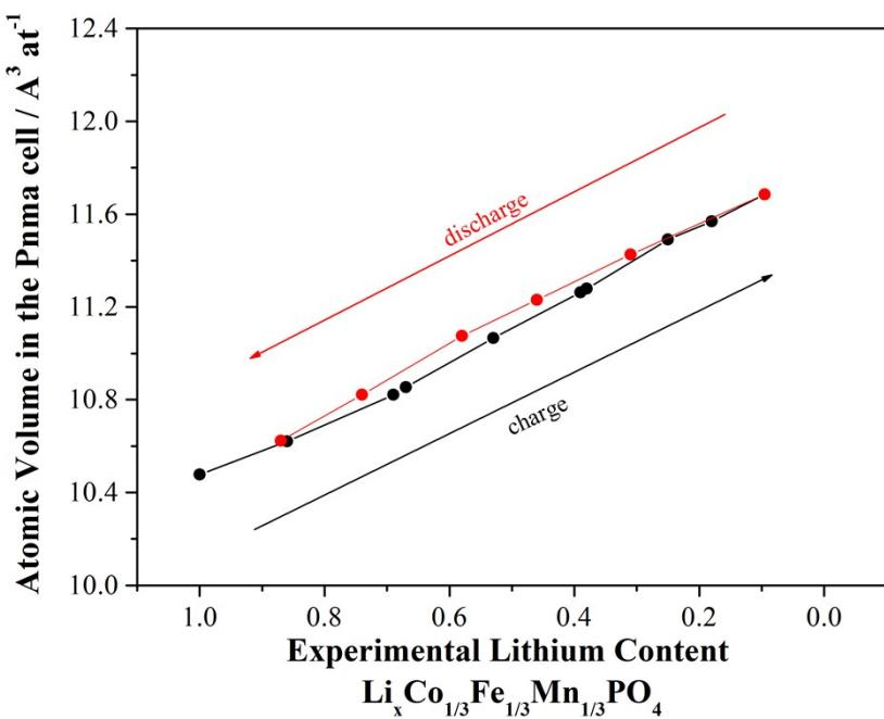
**Figure S24.** Evolution of the atomic volume in the Pnma orthorhombic cell upon electrochemical lithium extraction/insertion by Rietveld Refinement of the synchrotron XRD.
