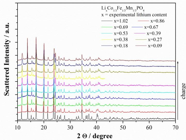
**Figure S7.** Evolution of the XRD patterns recorded on post mortem samples recuperated from lithium cells at various stages of charge
