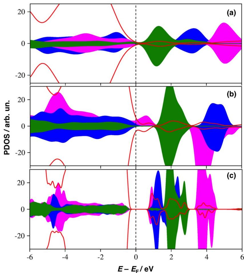
**Figure S6.** DFT+U computed Spin- angular-momentum and atom-projected density of states (PDOS) for LCFMP showing a sequential emptying of the electronic states after (a) 33%, (b) 66% and (c) 100% de-lithiation:  $E_F$  refers to the Fermi Energy; color legend: Co 3d (solid blue), Fe 3d (solid green), Mn 3d (solid magenta), O 2p (red line).
