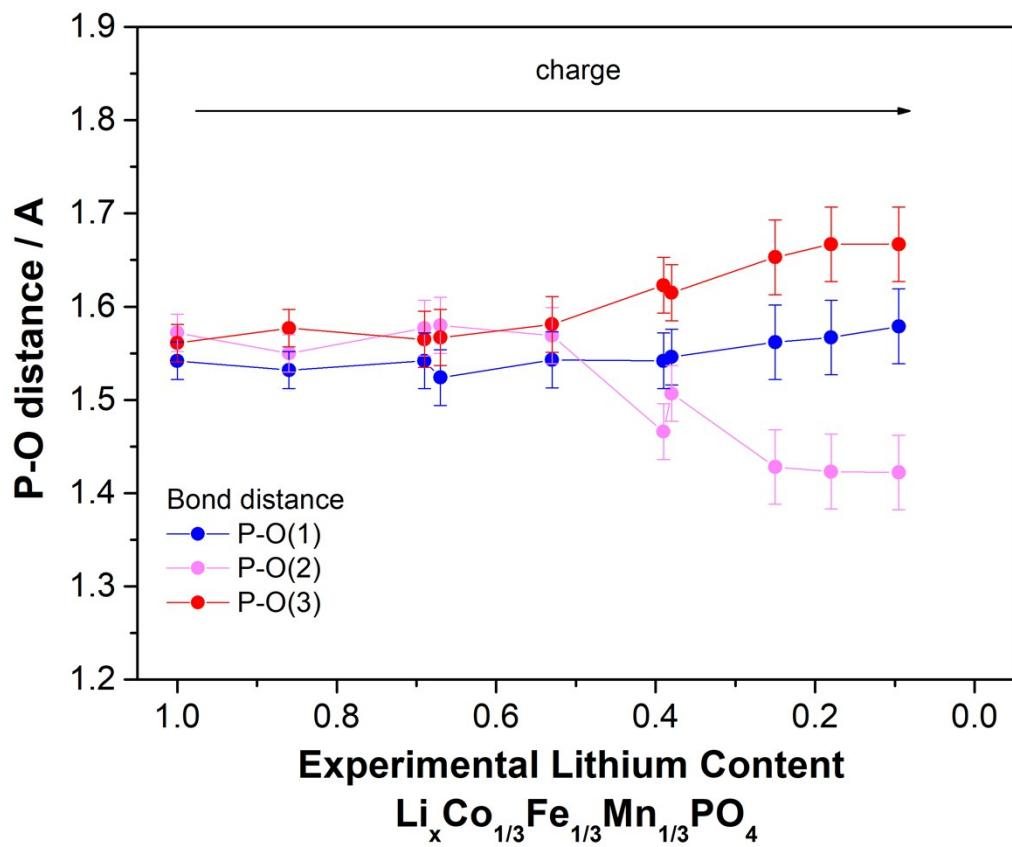
**Figure S28.** Experimental P-O bond distances at various lithium content in the LCFMP olivine lattice derived by the Rietveld Refinement performed on the XRD data
