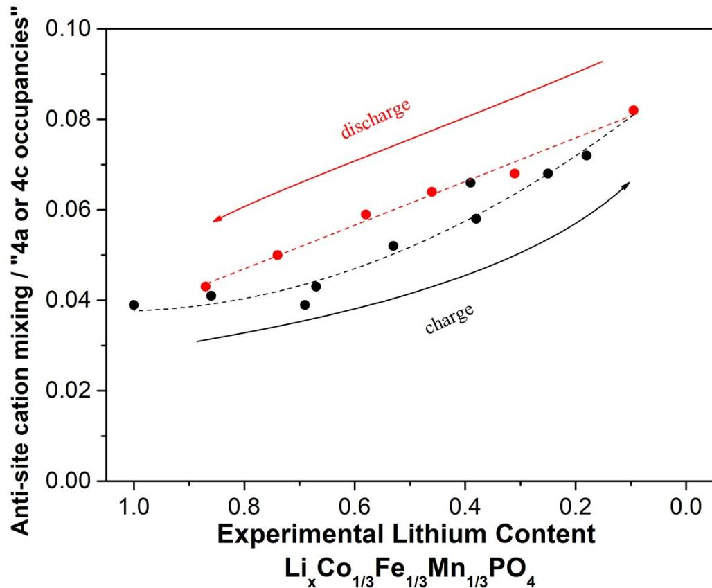
**Figure S27.** Evolution of 4a/4c anti-site defects upon electrochemical lithium extraction/insertion by Rietveld Refinement of the synchrotron XRD.
