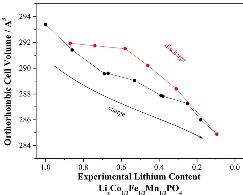
**Figure S25.** Evolution of Pnma orthorhombic cell volume upon electrochemical lithium extraction/insertion by Rietveld Refinement of the synchrotron XRD.
