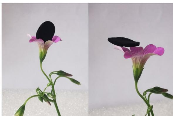
Fig. S4 Optical photograph of the ultralight N-PCNF aerogel standing on a flower
