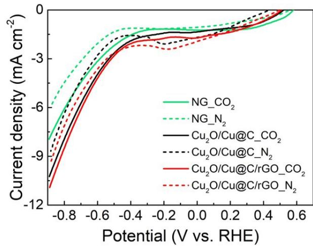
**Figure S6** LSV curves for NG, Cu<sub>2</sub>O/Cu@C, and Cu<sub>2</sub>O/Cu@C/rGO in N<sub>2</sub>- and CO<sub>2</sub>-saturated 0.1 M KHCO<sub>3</sub> electrolyte.
