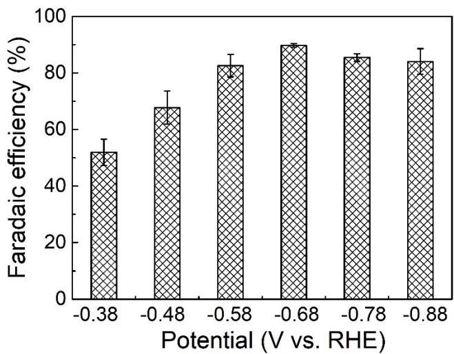
Figure S8 Faradaic efficiency for hydrogen of NG.
