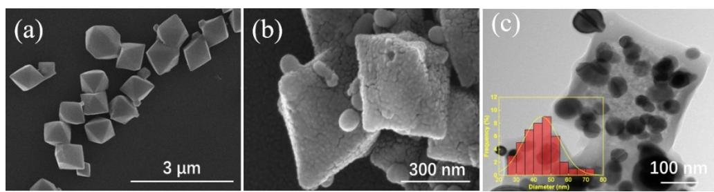
**Figure S2** SEM image of Cu\_btc particles (a), SEM (b) and TEM images (c) after Cu\_btc carbonization, insertion presented the size distribution of metallic nanoparticle.
