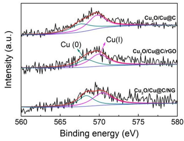
**Figure S4** Cu LMM Auger spectra of  $\text{Cu}_2\text{O}/\text{Cu}@\text{C}$ ,  $\text{Cu}_2\text{O}/\text{Cu}@\text{C/rGO}$ , and  $\text{Cu}_2\text{O}/\text{Cu}@\text{C/NG}$ .
