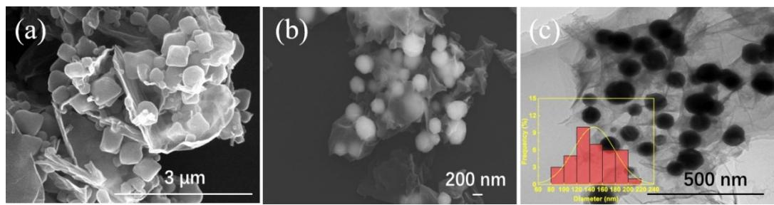
**Figure S3** SEM image of Cu\_btc/rGO composites (a), SEM (b) and TEM images (c) after Cu\_btc/rGO carbonization, insertion presented the size distribution of metallic nanoparticle.
