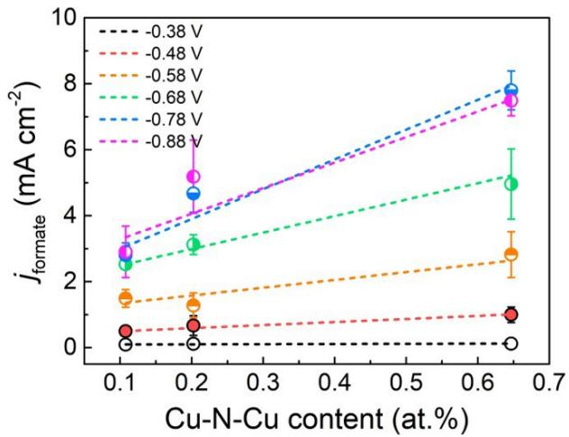
**Figure S11** The linear fitting between Cu-N-Cu content and partial current density of formate obtained by  $\text{Cu}_2\text{O}/\text{Cu@C}$ ,  $\text{Cu}_2\text{O}/\text{Cu@C/rGO}$  and  $\text{Cu}_2\text{O}/\text{Cu@C/NG}$ .
