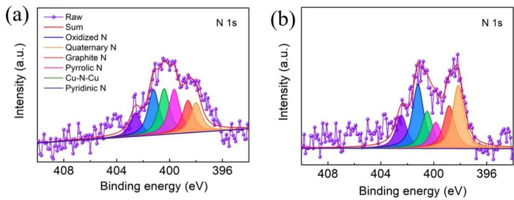
**Figure S5** Higher resolution of XPS N 1s of  $\text{Cu}_2\text{O}/\text{Cu}@\text{C}$  (a) and  $\text{Cu}_2\text{O}/\text{Cu}@\text{C}/\text{rGO}$  (b).
