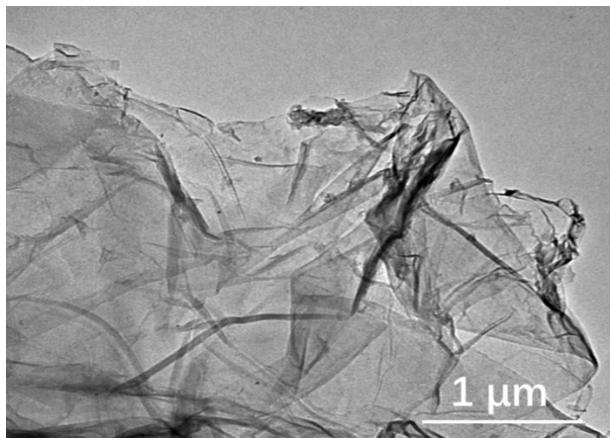
Figure S1 TEM N-doped reduced graphene oxide.
