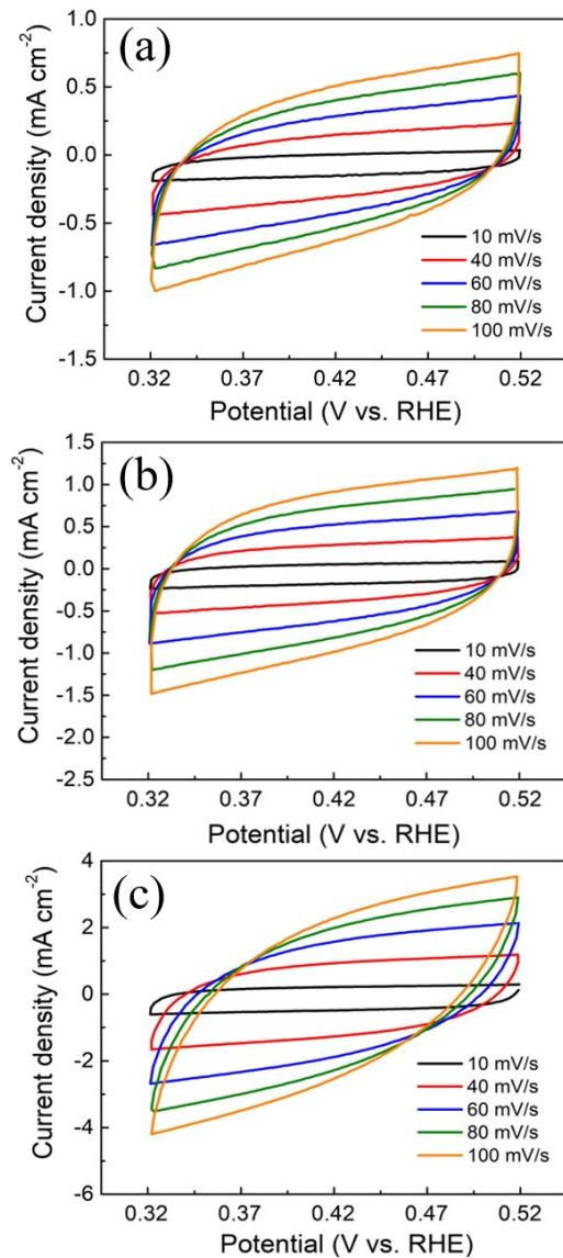
**Figure S10** Cyclic voltammograms at scan rate range from 10 to 100  $\text{mV s}^{-1}$  for  $\text{Cu}_2\text{O}/\text{Cu@C}$  (a),  $\text{Cu}_2\text{O}/\text{Cu@C/rGO}$  (b), and  $\text{Cu}_2\text{O}/\text{Cu@C/NG}$  (c), respectively.
