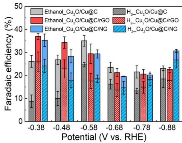
**Figure S7** Faradaic efficiency for hydrogen and ethanol of Cu<sub>2</sub>O/Cu@C, Cu<sub>2</sub>O/Cu@C/rGO, and Cu<sub>2</sub>O/Cu@C/NG.
