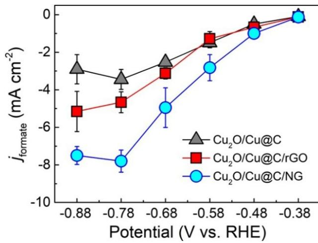
**Figure S9** Partial current density of formate for Cu<sub>2</sub>O/Cu@C, Cu<sub>2</sub>O/Cu@C/rGO, and Cu<sub>2</sub>O/Cu@C/NG.
