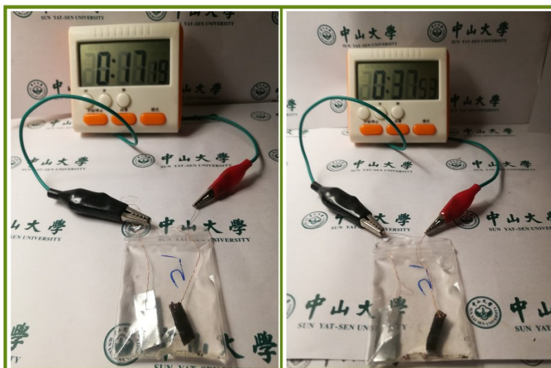
Fig. S6. The photograph of a timer lightened by the soft-package battery.
