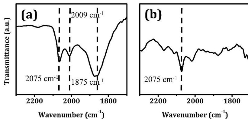
**Figure S5.** FTIR patterns obtained for (a) Rh/CaO/MgAl<sub>2</sub>O<sub>4</sub> and (b) Rh/TiO<sub>2</sub>/MgAl<sub>2</sub>O<sub>4</sub> after exposure to CO at room temperature after five 1073 K redox cycles with the final treatment being reduction.
