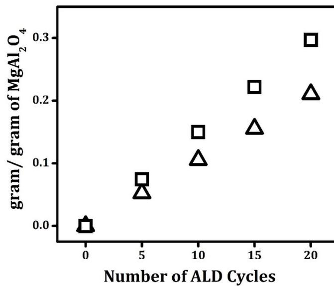
**Figure S1.** Growth curves for ALD films on a 120m<sup>2</sup>/g MgAl<sub>2</sub>O<sub>4</sub> support for (Δ) Sr-ALD process and (□) Ba-ALD process
