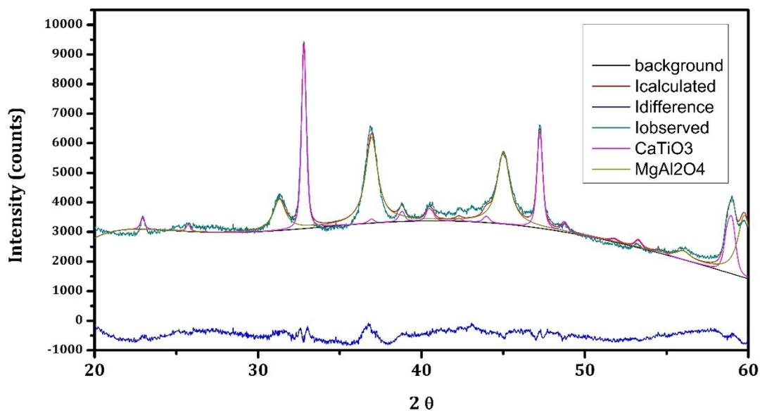
**Figure S3.** Rietveld refinement for the  $\text{CaTiO}_3/\text{MgAl}_2\text{O}_4$  samples.
