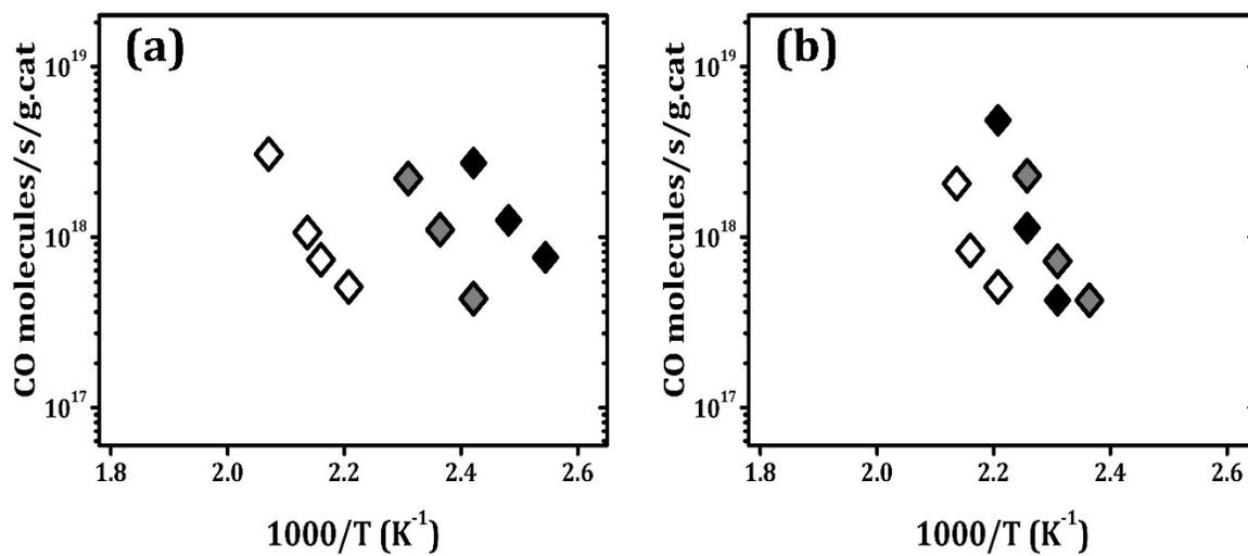
**Figure S7.** Steady-state, differential reaction rates for CO oxidation with 25 Torr of CO and 12.5 Torr O<sub>2</sub> for (a) Rh/CaO/MgAl<sub>2</sub>O<sub>4</sub> (b) Rh/TiO<sub>2</sub>/MgAl<sub>2</sub>O<sub>4</sub> as a function of reduction temperature. Reduction pretreatment temperature: (white) no reduction, (grey) 573K reduction and (black) 1073K reduction.
