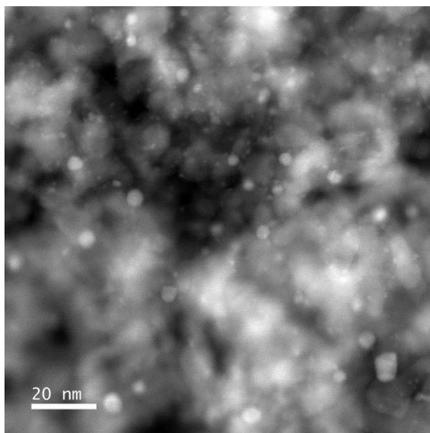
**Figure S4.** STEM result for Rh/MgAl<sub>2</sub>O<sub>4</sub>, after five 1073-K redox cycles, with the final step being reduction.
