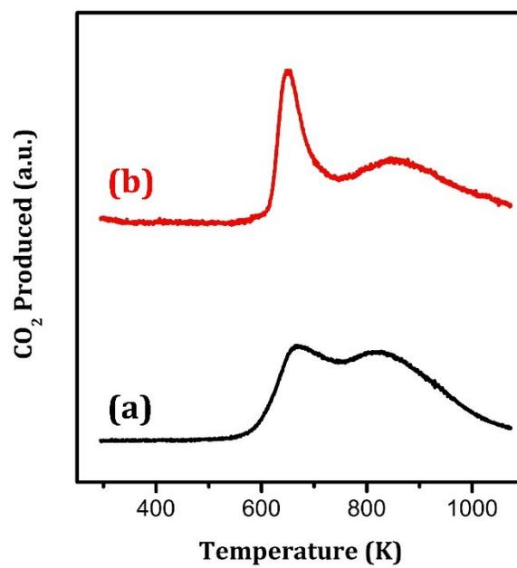
**Figure S8.** CO-TPR profile for (a)Rh/CaO/MgAl<sub>2</sub>O<sub>4</sub> and (b)Rh/TiO<sub>2</sub>/MgAl<sub>2</sub>O<sub>4</sub>
