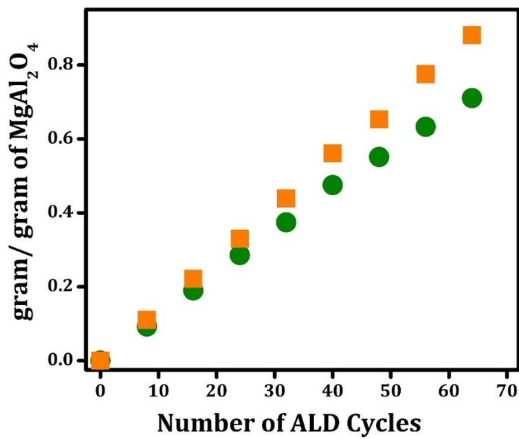
**Figure S2.** Growth curves for ALD films on a 120m<sup>2</sup>/g MgAl<sub>2</sub>O<sub>4</sub> support for (●) SrTiO<sub>3</sub>/MgAl<sub>2</sub>O<sub>4</sub> and (■) BaTiO<sub>3</sub>/MgAl<sub>2</sub>O<sub>4</sub> process.
