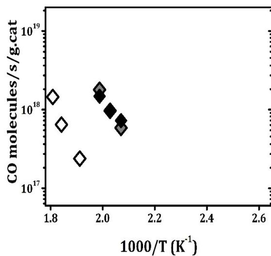
**Figure S6.** Steady-state, differential reaction rates for CO oxidation with 25 Torr of CO and 12.5 Torr O<sub>2</sub> for Rh/CaTiO<sub>3</sub>/MgAl<sub>2</sub>O<sub>4</sub> with extra Ca (Ca:Ti=1.1) as a function of reduction temperature. Reduction pretreatment temperature: (white) no reduction, (grey) 573 K reduction, and (black) 1073 K reduction.
