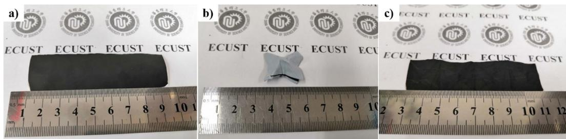
**Figure S12.** Digital images of SMF modified separators before folding (a), folding (b) and after folding (c), respectively.
