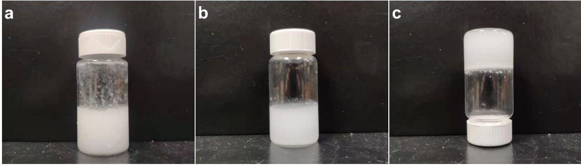
Figure S1. Photos of CNF and CNF-PAM solid-state electrolytes. (a) CNF dispersed in the solution of 1 M \text{Zn}(\text{CF}_3\text{SO}_3)_2 ; (b), (c) CNF-PAM prepared by the radical polymerization.
