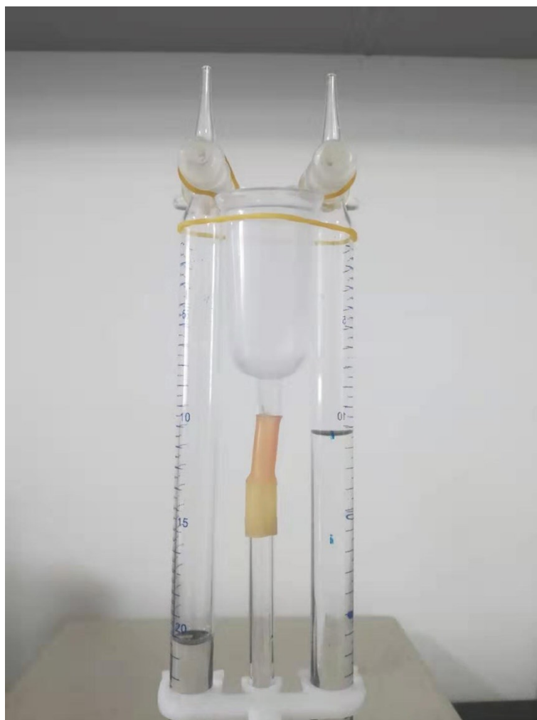
Fig. S22 The optical picture of the measured setup of the Hoffman apparatus.
