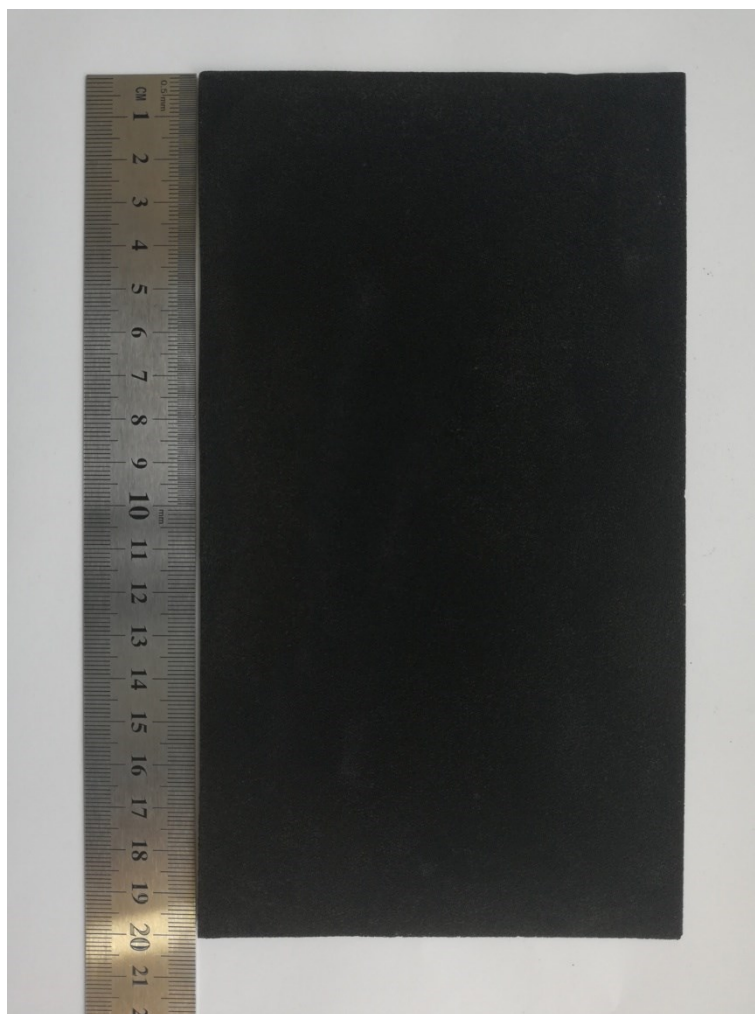
Fig. S2 Photo of the RuO 2 -NiO/NF with an area of 200 cm 2 .
