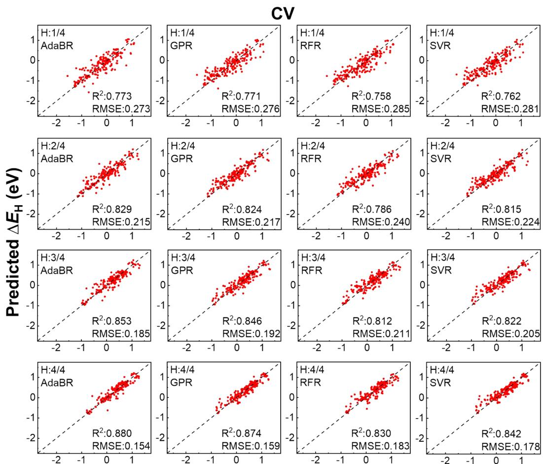
**Fig. S11.** Cross validation for several typical machine learning models for four H coverages without group-VIB  $M_nX_{n+1}O_2$  ( $M = Cr, Mo, W; n = 1, 2, 3$ ).
