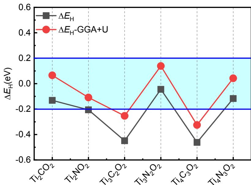
**Fig. S5.** Comparison of  $\Delta E_H$  calculated by GGA and GGA + U for Ti-monometallic MXenes. The corresponding  $U_{\text{eff}}$  values were set to 2.58 for the Ti element<sup>1</sup>.
