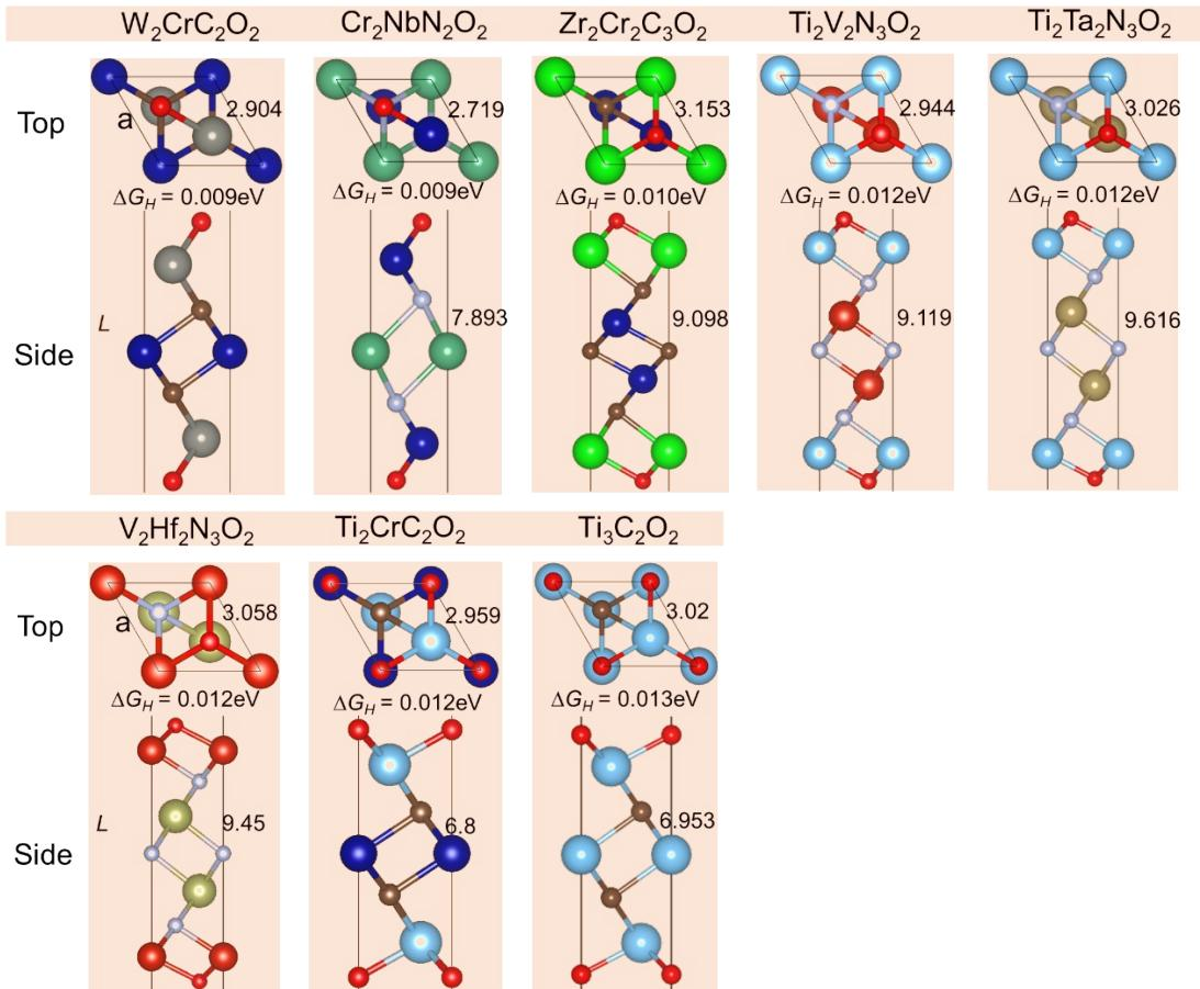
**Fig. S2.** The structure information of  $Ti_3C_2O_2$  and 22 MXenes OBAs with better catalytic activity than  $Ti_3C_2O_2$ . Lattice parameters are expressed in terms of  $a$ , and  $L$  in terms of layer thickness. The top and side views of all structures are listed in the order of  $\Delta G_H$ .
