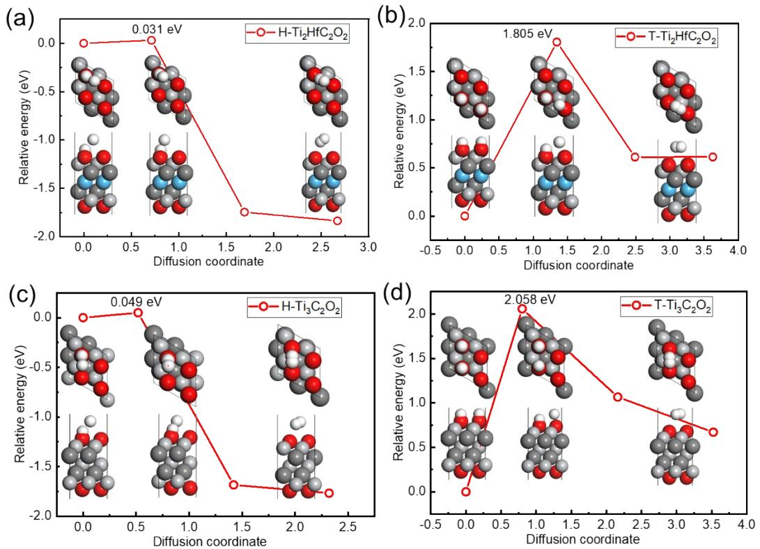
**Fig. S4.** The activation barriers of H on HfC<sub>2</sub>O<sub>2</sub> (a-b); Ti<sub>3</sub>C<sub>2</sub>O<sub>2</sub> (c-d). The “T-” represents the Tafel reaction while the “H-” typifies the Heyrovsky reaction. The inserted structure diagrams are the reaction of initial state (IS), the transition state (TS) and the final state (FS).
