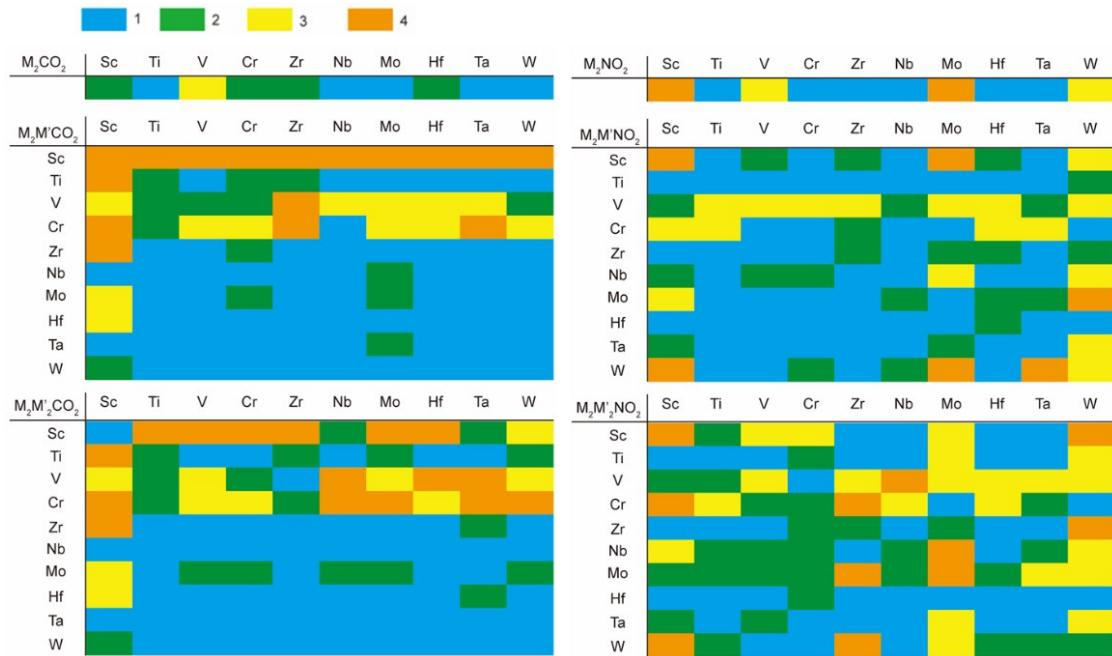
**Fig. S1.** Heat map showing the H equilibrium coverage for different MXenes. Under these conditions, the equilibrium coverage is defined as the coverage at which the free energy of hydrogen adsorption ( $\Delta G_H$ ) is closest to zero. 1, 2, 3, 4 denote the H coverage of 1/4, 2/4, 3/4 and 4/4, respectively.
