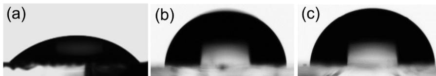
**Figure S16.** Water contact angles (CA) measured on various perovskite thin films: (a) uncoated, (b) 1 nm PPX-coated and (c) 5 nm PPX-coated perovskite thin films.
