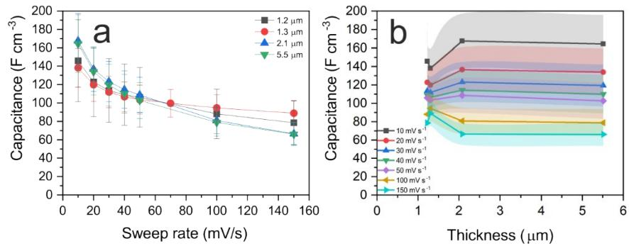
*Figure S8.* a) Volumetric capacitance vs sweep rate of GO-CNT-Ce-Mn-5152 for diverse thicknesses and b) volumetric capacitance vs thickness for different sweep rates.
