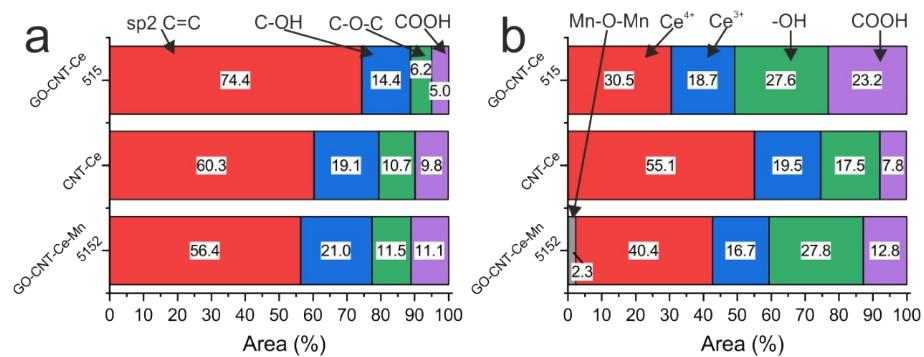
Figure S6. Integrated area of XPS a) C1s and b) O1s high resolution spectra.
