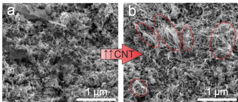
Figure S4. XHRSEM images at 100000x of a) GO-CNT-Ce-515, and b) GO-CNT-Ce-525. Regions with agglomerated CNTs are indicated.
