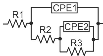
*Figure S9* Equivalent circuit for data fitting
