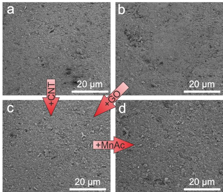
*Figure S1.* XHRSEM images at 5000x of a) GO-Ce, b) CNT-Ce, c) GO-CNT-Ce-515, and d) GO-CNT-Ce-Mn-5151.
