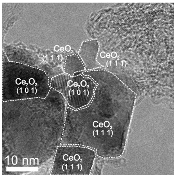
Figure S5. HRTEM of GO-CNT-Ce-515 with highlighted different crystalline regions.
