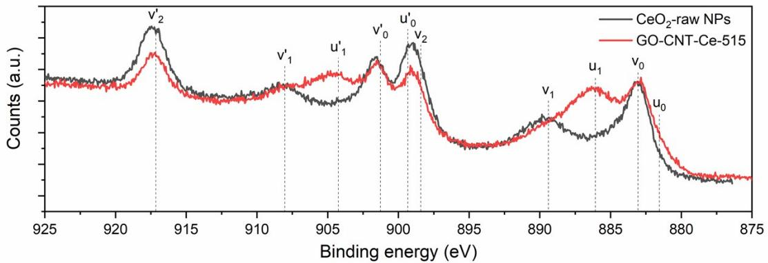
*Figure S7.* Ce 3d<sub>3/2</sub> and Ce 3d<sub>5/2</sub> high resolutions XPS of CeO<sub>2</sub>-raw nanoparticles and GO-CNT-Ce-515 for comparison.
