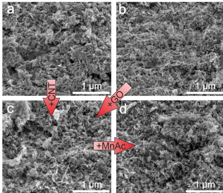
Figure S2. XHRSEM images at 100000x of a) GO-Ce, b) CNT-Ce, c) GO-CNT-Ce-515, and d) GO-CNT-Ce-Mn-5151.
