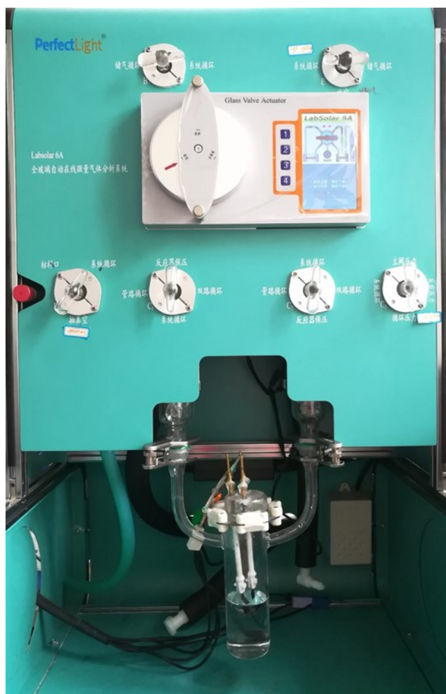
Fig. S16. Digital photographs of the setup of the water decomposition hydrogen production system
