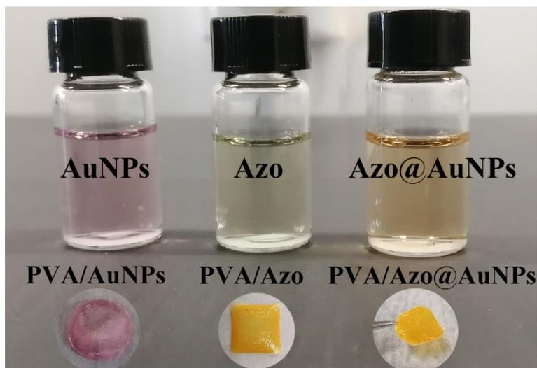
**Figure S7** Photos of AuNPs, tri-Azo and tri-Azo@AuNPs in DMF solution and corresponding PVA/AuNPs, PVA/Azo and PVA/Azo@AuNPs film.
