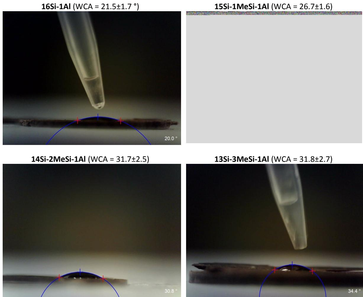
**Fig. 21S:** The results of water contact angle measurements for aluminosilicate samples with varying  $\text{CH}_3\text{Si}$  groups content. Average numbers based on 5-10 measurements and the best captured image for each sample.
