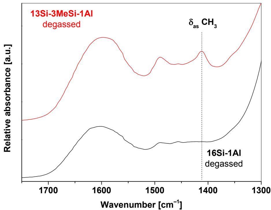
**Fig. 18S:** IR spectra of 16Si-1Al and 13Si-3MeSi-1Al after evacuation at 350 °C.
