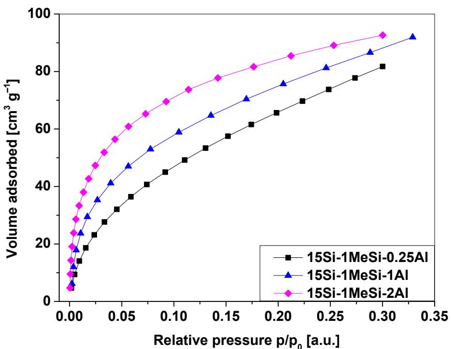
**Fig. 7S:** Water adsorption measurements performed at low  $p/p_0$  (< 0.3) on samples with different Si:Al ratio.
