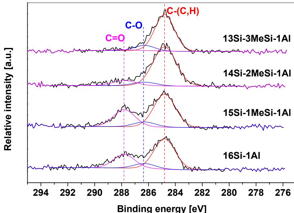
**Fig. 11S:** XPS spectra (C 1s) of NHSG prepared aluminosilicates with various MeSi groups content.
