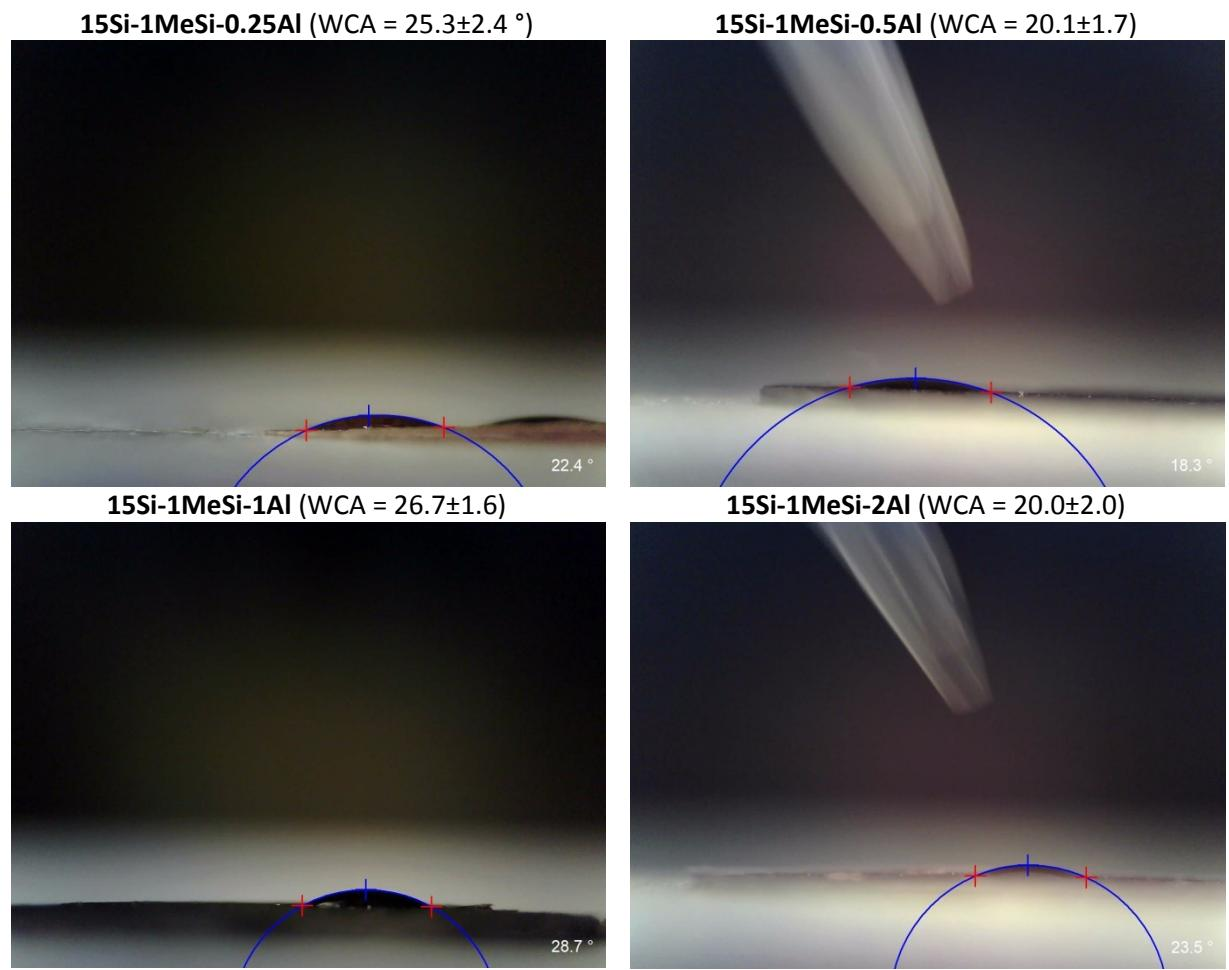
**Fig. 9S:** The results of water contact angle measurements for aluminosilicate samples with varying Si:Al ratio. Average numbers based on 5-10 measurements and the best captured image for each sample.
