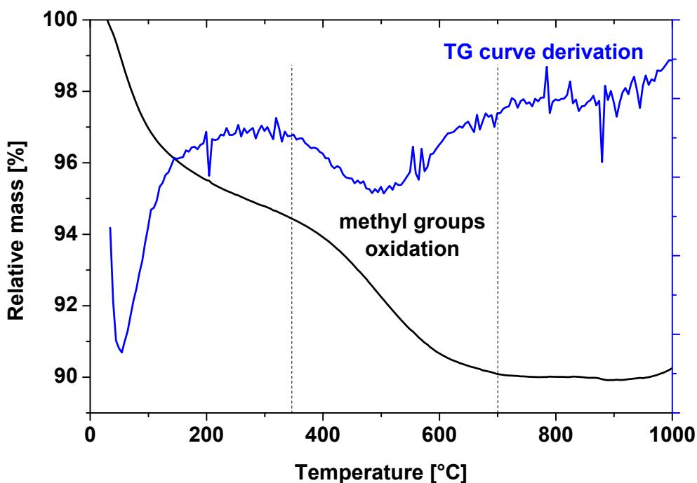
**Fig. 1S:** TG analysis of sample 15Si-1MeSi-1Al.
