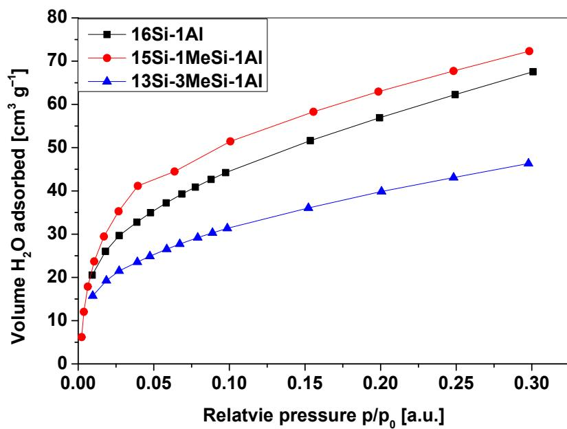
**Fig. 20S:** Water adsorption measurements performed at low  $p/p_0$  ( $< 0.3$ ) on samples with different MeSi groups loading.
