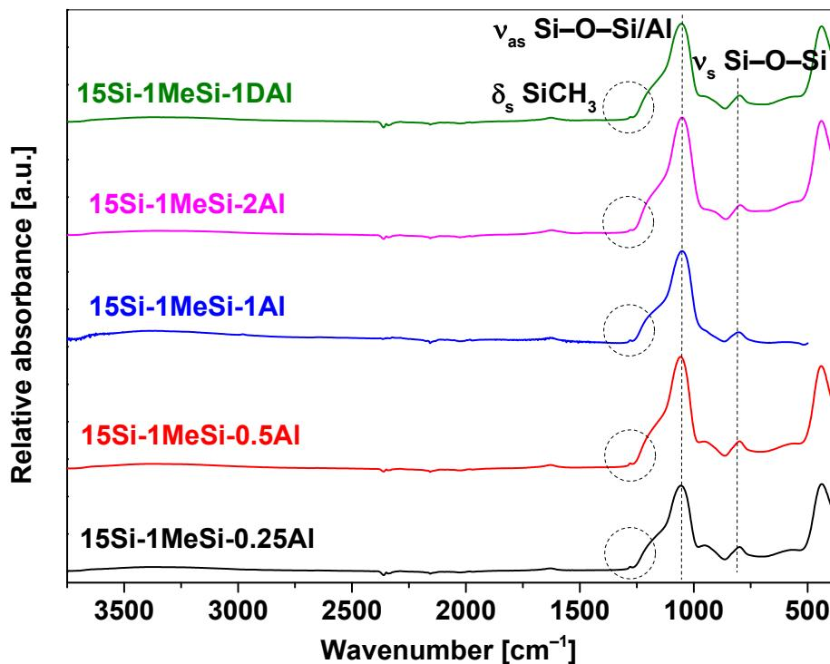
**Fig. 2S:** IR spectra of NHSG prepared samples with different Si/Al ratio and delayed Al addition.
