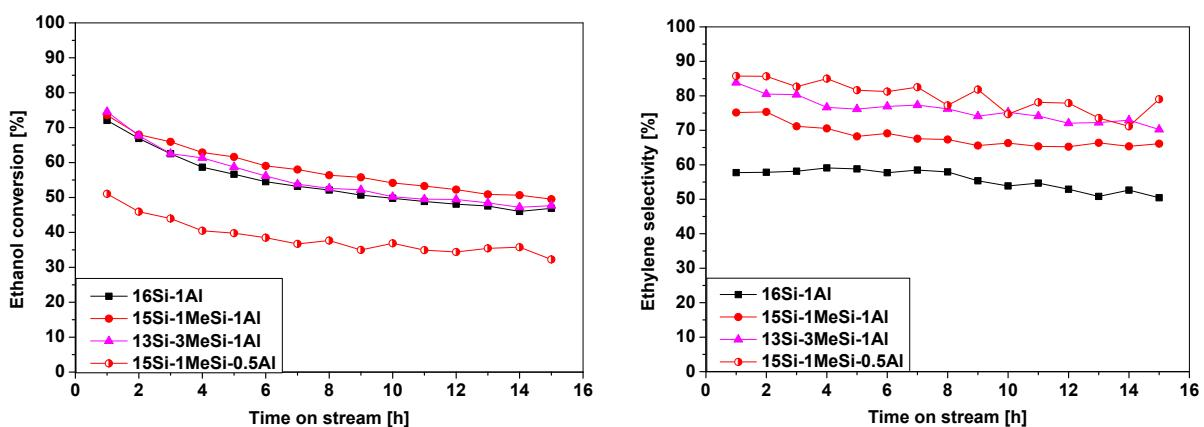
**Fig. 24S:** Conversion (left) and ethylene selectivity (right) at 240 °C over NHSG aluminosilicate catalysts during 15 h time on stream stability test.
