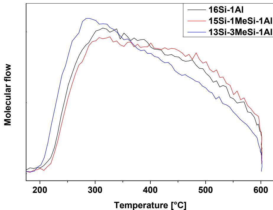
**Fig. 19S:** NH<sub>3</sub>-TPD curves of samples with different Si—CH<sub>3</sub> groups loading showing only subtle changes during methylation of NHSG prepared aluminosilicates.
