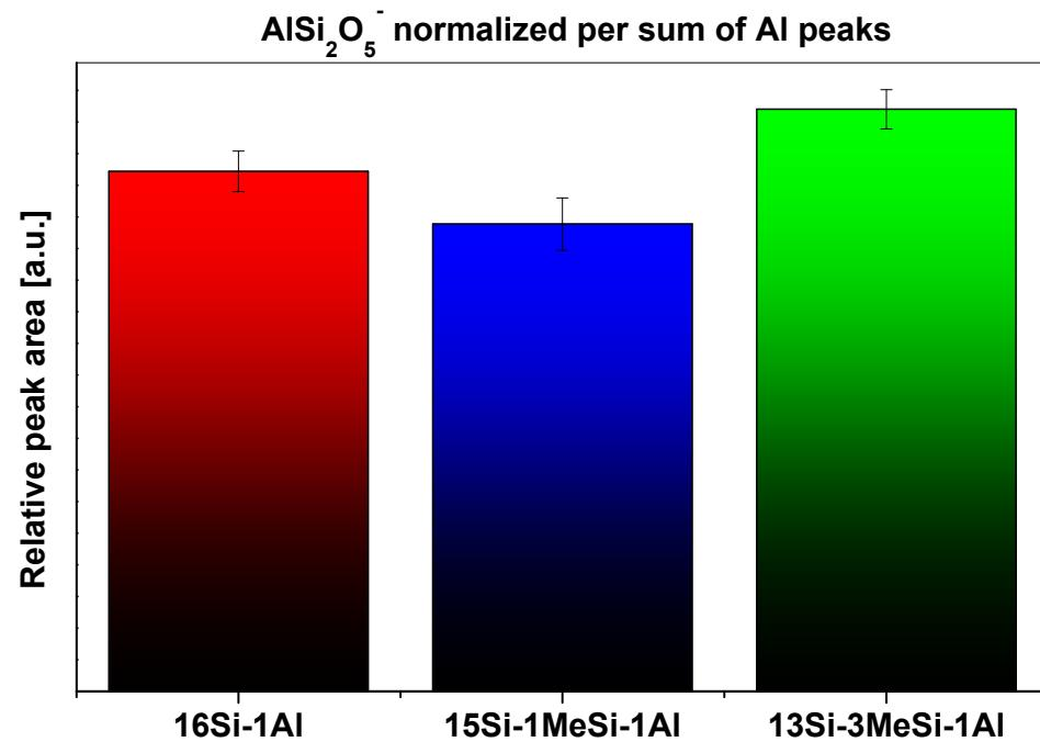
**Fig. 17S:** Comparison of samples with different Si—CH<sub>3</sub> groups loading in terms of relative peak areas of masses corresponding to AlSi<sub>2</sub>O<sub>5</sub><sup>-</sup> ions (mixed Al-Si clusters) in mass spectra obtained by ToF-SIMS.
