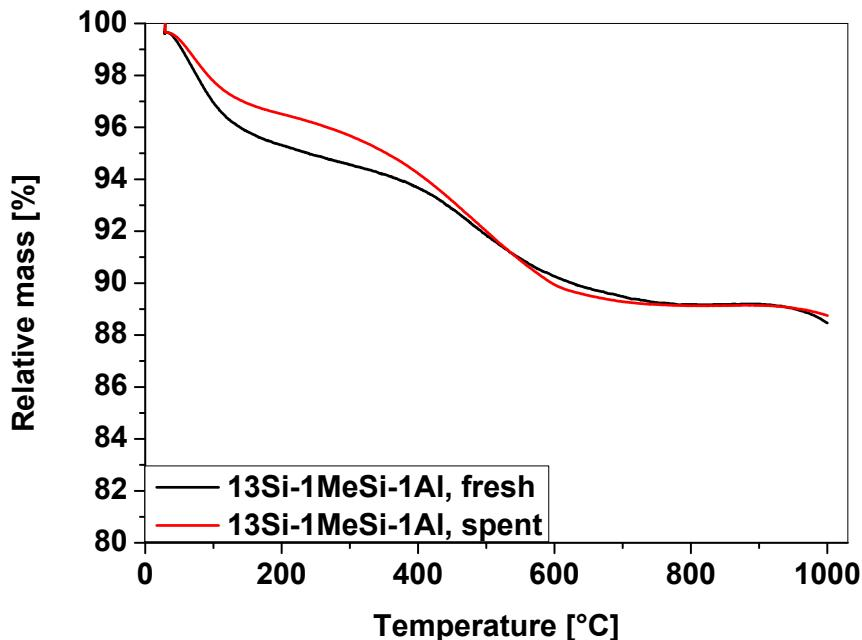
**Fig. 23S:** Comparison of TG analyses of spent and fresh 13Si-3Mesi-1Al catalyst.
