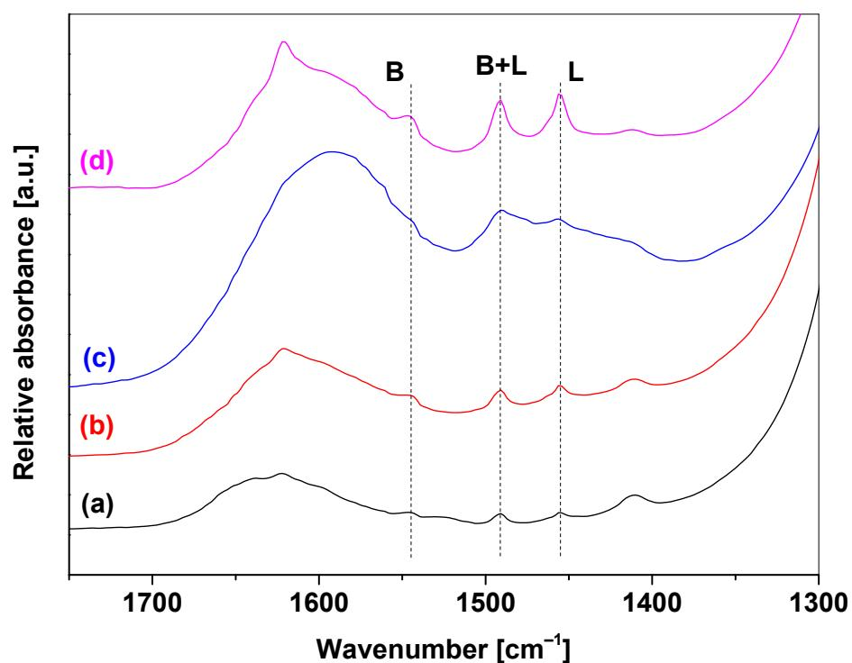
**Fig. 5S:** IR spectra of **15Si-1MeSi-0.25Al** (a), **15Si-1MeSi-0.5Al** (b), **15Si-1MeSi-2Al** (c), and **15Si-1MeSi-1DAI** (d) after evacuation at 350 °C, pyridine adsorption, and degassed at 150 °C.
