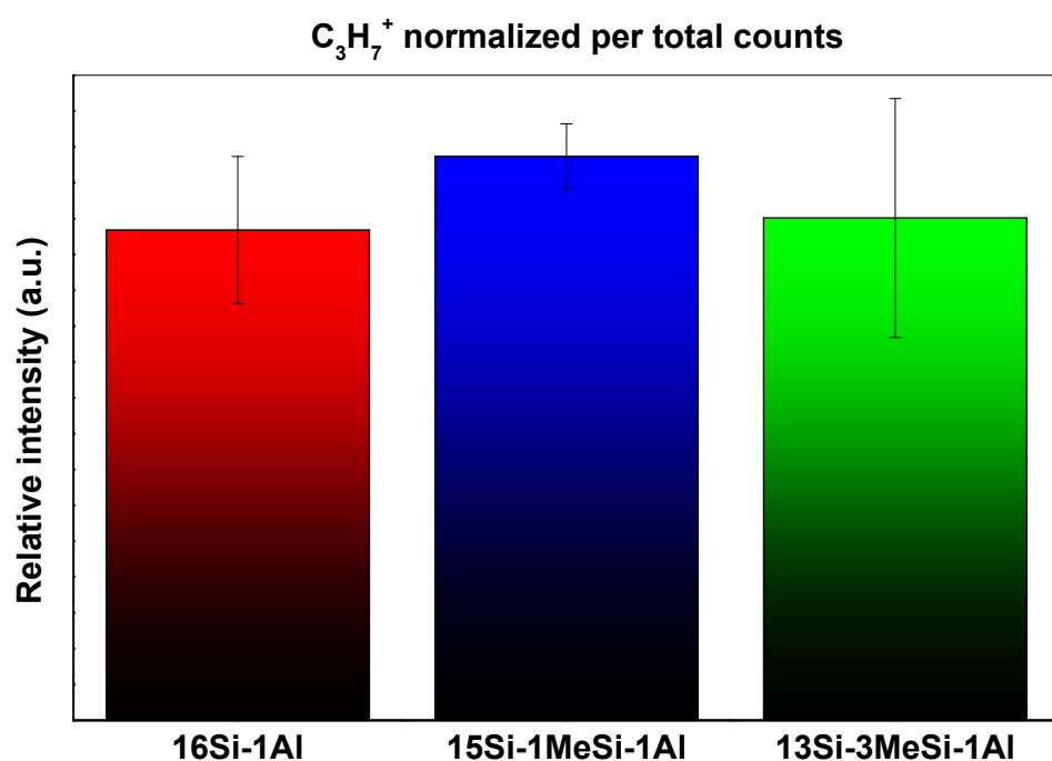
**Fig. 15S:** Comparison of samples with different Si— $\text{CH}_3$  groups loading in terms of relative peak areas of masses corresponding to  $\text{C}_3\text{H}_7^+$  ions in mass spectra obtained by ToF-SIMS.
