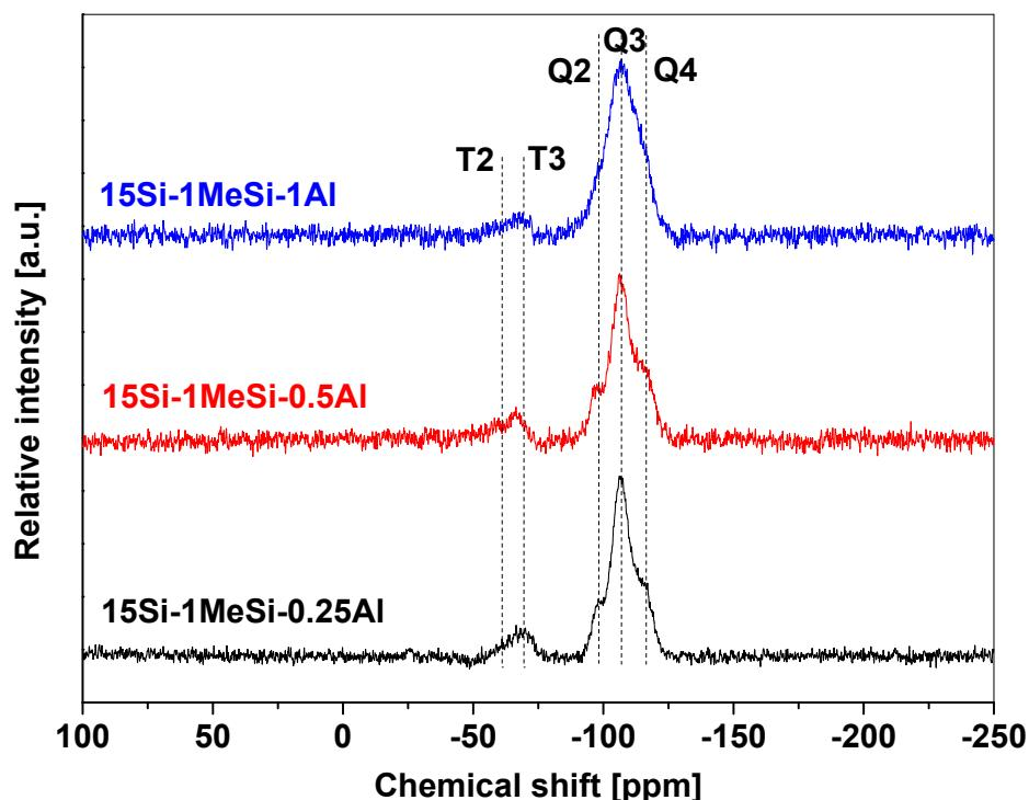
**Fig. 3S:** <sup>29</sup>Si CPMAS NMR spectra of NHSG prepared samples with different Si/Al loading.
