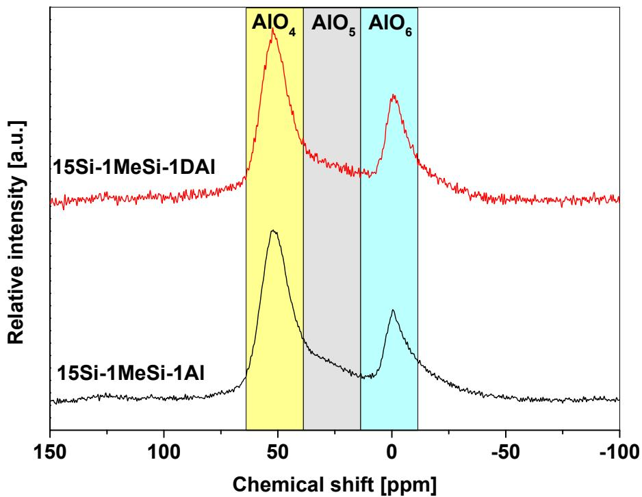
**Fig. 25S:**Comparison of  $^{27}\text{Al}$  MAS NMR spectra of **15Si-1MeSi-1Al** and **15Si-1MeSi-1DAI**.
