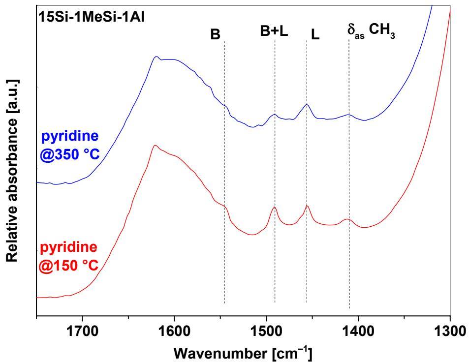
**Fig. 4S:** IR spectra of **15Si-1MeSi-1Al**, after pyridine adsorption and degassed at different temperatures.
