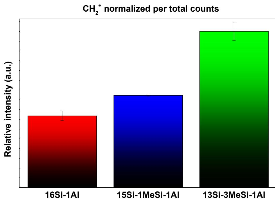
**Fig. 14S:** Comparison of samples with different Si— $\text{CH}_3$  groups loading in terms of relative peak areas of masses corresponding to  $\text{CH}_2^+$  ions in mass spectra obtained by ToF-SIMS.
