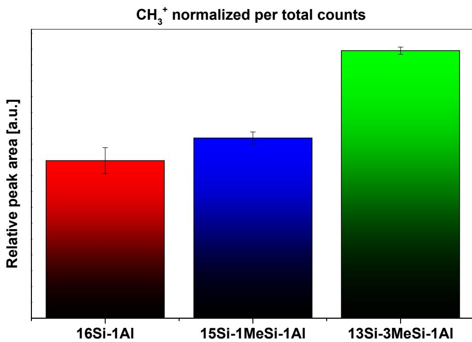
**Fig. 13S:** Comparison of samples with different Si—CH<sub>3</sub> groups loading in terms of relative peak areas of masses corresponding to CH<sub>3</sub><sup>+</sup> ions in mass spectra obtained by ToF-SIMS.
