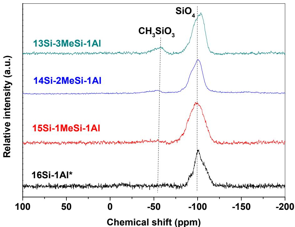
**Fig. 10S:**  $^{29}\text{Si}$  MAS NMR spectra of NHSG prepared samples with different Si— $\text{CH}_3$  groups loading. Asterisk denotes  $^{29}\text{Si}$  CPMAS NMR spectrum.
