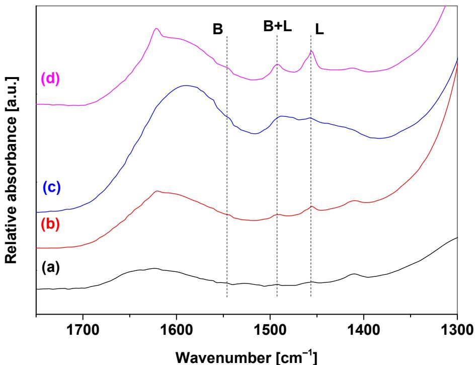
**Fig. 6S:** IR spectra of **15Si-1MeSi-0.25Al** (a), **15Si-1MeSi-0.5Al** (b), **15Si-1MeSi-2Al** (c), and **15Si-1MeSi-1DAI** (d) after evacuation at 350 °C, pyridine adsorption, and degassed at 350 °C.
