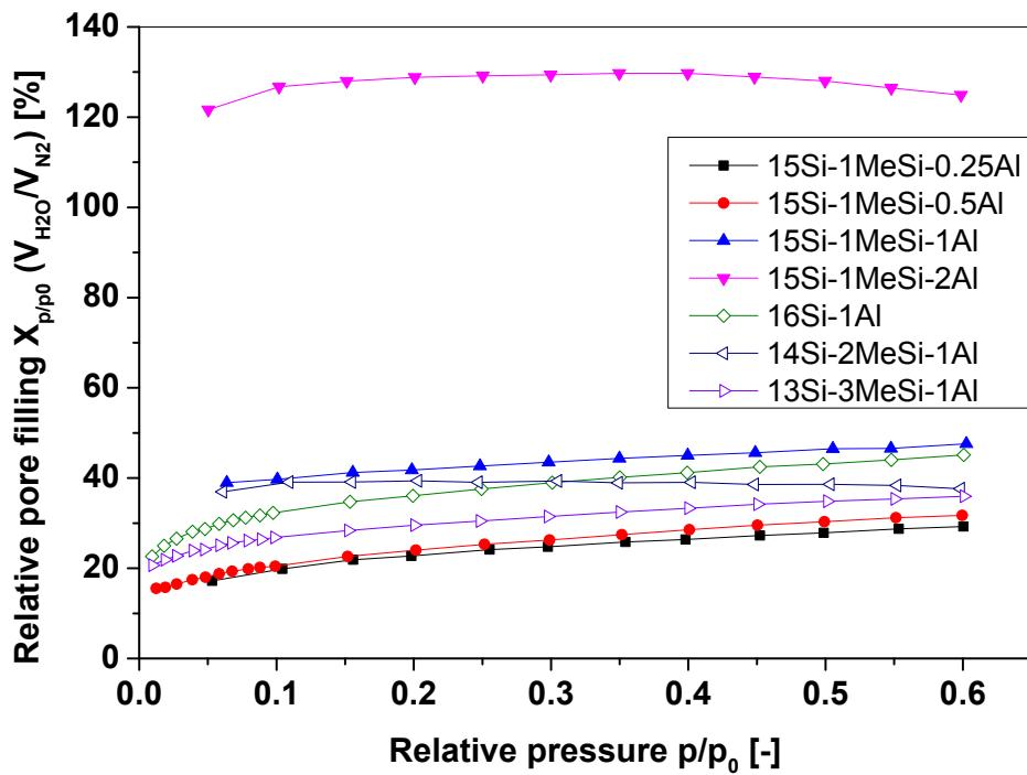
**Fig. 8S:** Volume of adsorbed H<sub>2</sub>O over the volume of adsorbed N<sub>2</sub> at given p/p<sub>0</sub> values (X<sub>p/p<sub>0</sub></sub>; both adsorbates being considered as in liquid phase).
