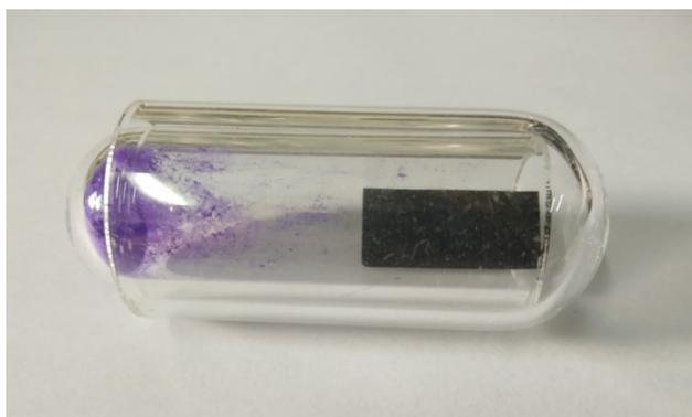
**Fig. S1.** The digital photograph for the quartz socket tube loaded with ZIF-67 and MoO<sub>3</sub>/CFP inside two sides.
