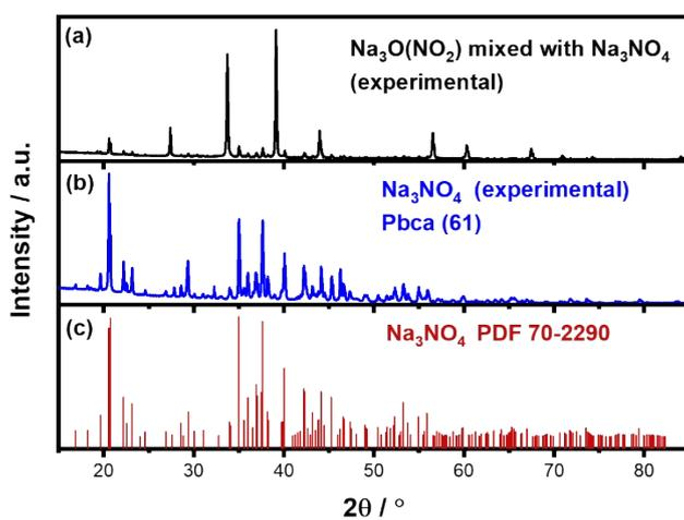
**Fig. S2** (a) Powder XRD pattern of  $\text{Na}_3\text{ONO}_2$  mixed with  $\text{Na}_3\text{NO}_4$ . (b) Powder XRD pattern of  $\text{Na}_3\text{NO}_4$ . (c) Powder diffraction file (PDF) of  $\text{Na}_3\text{NO}_4$ .
