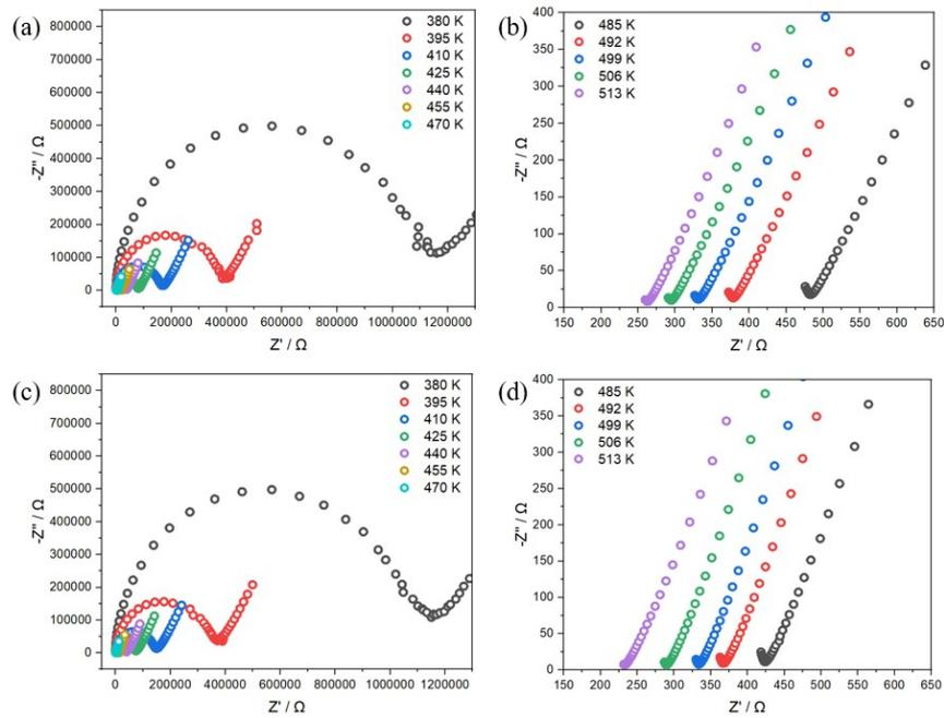
**Fig. S4** (a), (b) Nyquist curves of  $\text{Na}_3\text{ONO}_2$  during heating. (c), (d) Nyquist curves of  $\text{Na}_3\text{ONO}_2$  during cooling.
