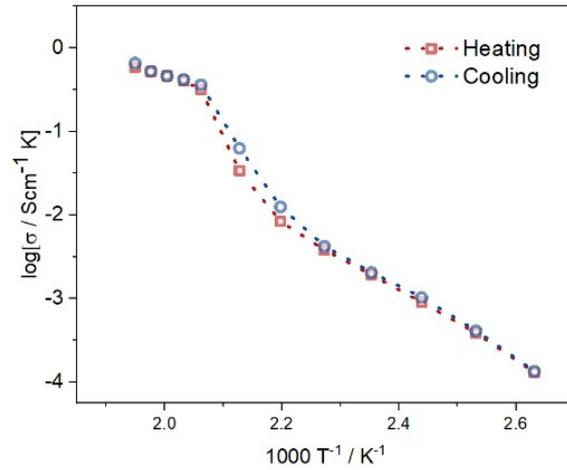
**Fig. S3** Arrhenius conductivity plot of  $\text{Na}_3\text{ONO}_2$  during heating and cooling.
