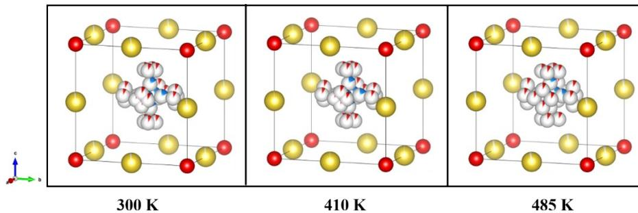
**Fig. S5** Crystal model of  $\text{Na}_3\text{ONO}_2$  after refinement based on neutron powder diffraction (NPD) at selected temperature.
