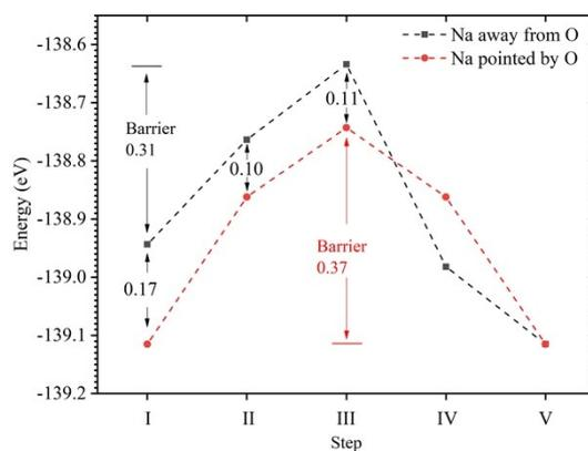
**Fig. S9** Calculated energy of each step for two models. Red line is the stable model where Na is pointed by O, while black line is a metastable model where  $\text{Na}^+$  is away from  $\text{O}^{2-}$  in its initial states.
