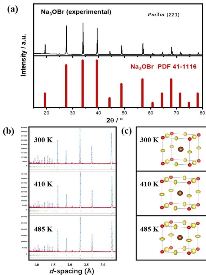
**Fig. S10** (a) Powder XRD pattern of  $\text{Na}_3\text{OBr}$  at room temperature. (b) Rietveld refinement of  $\text{Na}_3\text{OBr}$  based on NPD at 300 K, 410 K and 485 K. (c) Schematic crystal structure of  $\text{Na}_3\text{OBr}$  at 300 K, 410 K and 485 K with anisotropic thermal displacements.
