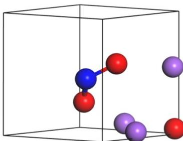
**Fig. S12** Structure of  $\text{Na}_3\text{ONO}_2$  after optimization, O in  $\text{NO}_2$  pointing to lattice Na.
