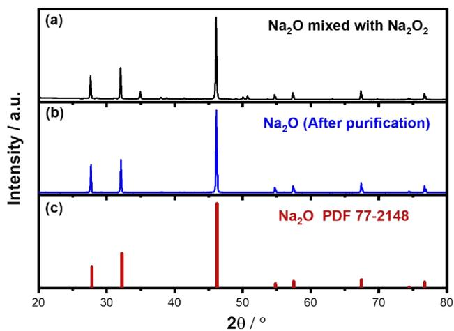
**Fig. S1** (a) Powder XRD pattern of  $\text{Na}_2\text{O}$  before purification. (b) Powder XRD pattern of  $\text{Na}_2\text{O}$  after purification. (c) Powder diffraction file (PDF) of  $\text{Na}_2\text{O}$ .
