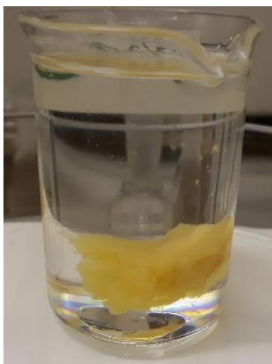
Figure S5: Insoluble fraction of PP-vitrimer (1 wt% Zn(acac) 2 and DGEBA/MA = 1.7) after swelling 24 hours in hot xylene (at 120 °C).
