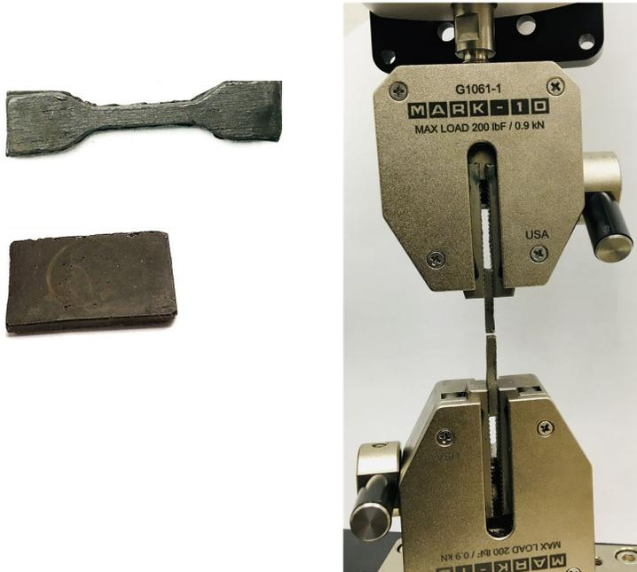
**Figure S9.** Digital images of **GS<sub>80</sub>** samples and the image of tensile strength tested dog bone shaped **GS<sub>80</sub>** sample, clamped down with a Mark 10 wedge grip.
