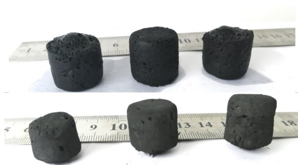
Figure S2. Optical images of hydrogels and aerogels for GMN2 (the hydrogel does not significantly shrink after atmospheric drying).
