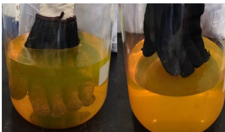
Figure S37 Waterproofing test of the fabric glove treated with \text{Si}_{\text{Pa-160}}/\text{CNTs-3} .
