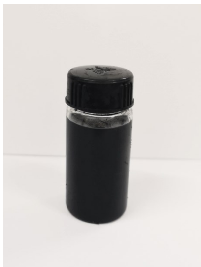
Figure S26 Visual images of uncured \text{Si}_{\text{Pa-160}} systems' cyclohexane solution dispersing multi-walled carbon nanotubes.
