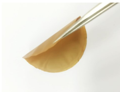
Fig. S13 Optical image of Vr/PEO-LCSE with thickness of 10 \mu\text{m} .
