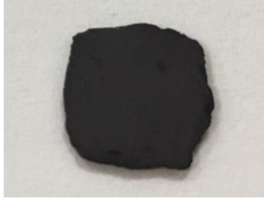
Figure S1. Optical image of pellet formed by starting with powders that had been annealed 4 times in Cu rich atmosphere, pressing these into a Cu box, and annealing again in a tube furnace at 600 °C for 9 hours with 500 sccm flow rate of argon to obtain a dense sintered pellet.
