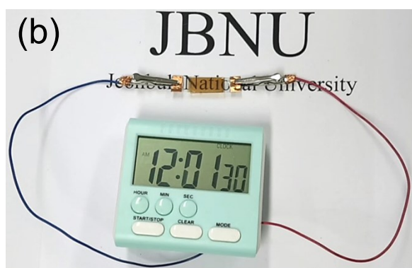
Fig. S12 Digital photographs of a digital clock power up by a single FT-ASSc device at a different time scale: (a) 30 sec (b) 1 min 30 sec and (c) 2 min 30 sec demonstrating the high energy density and power density of the FT-ASSc device.
