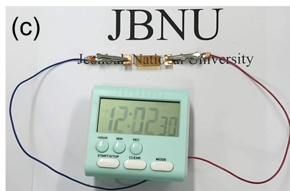
Fig. S12 Digital photographs of a digital clock power up by a single FT-ASSc device at a different time scale: (a) 30 sec (b) 1 min 30 sec and (c) 2 min 30 sec demonstrating the high energy density and power density of the FT-ASSc device.
