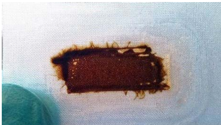
Figure S9. Fumasep®FAP-375-PP AEM after galvanostatic battery cycling.
