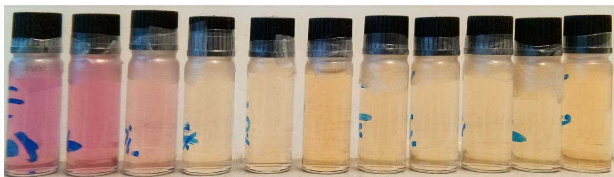
Figure S8, UV-Vis samples ordered as follows (from left to right): negolyte 100%, 80%, 60%, 40%, 20%, original electrolyte solution, posolyte 20%, 40%, 60%, 80%, 100%.
