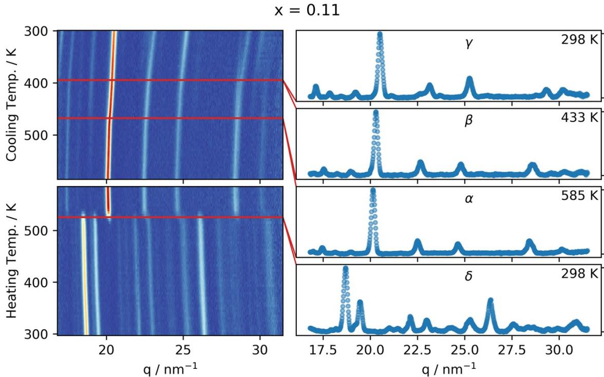
**Fig. S4** Left, integrated GIWAXS pattern as a function of temperature for  $\text{CsPb}(\text{Br}_x\text{I}_{1-x})_3$  with  $x = 0.11$  (determined by in-situ XRF) as the sample is heated and then cooled at a rate of 2.5 K/min. Red lines indicate the phase transitions. Right, integrated GIWAXS patterns for the four different phases in the sample.
