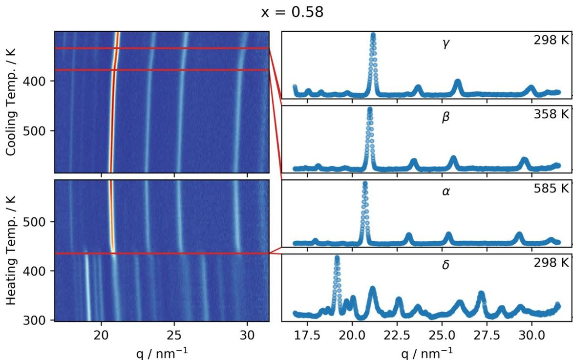
**Fig. S10** Left, integrated GIWAXS pattern as a function of temperature for  $\text{CsPb}(\text{Br}_x\text{I}_{1-x})_3$  with  $x = 0.58$  (determined by in-situ XRF) as the sample is heated and then cooled at a rate of 2.5 K/min. Red lines indicate the phase transitions. Right, integrated GIWAXS patterns for the four different phases in the sample.
