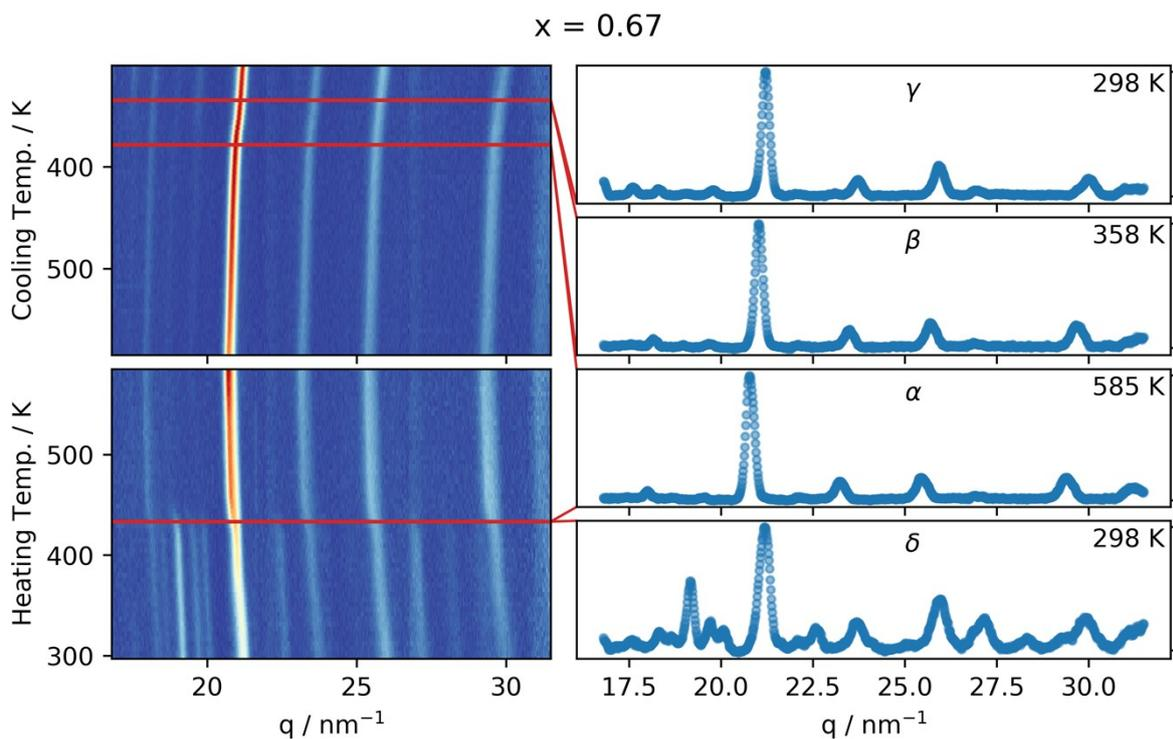
**Fig. S11** Left, integrated GIWAXS pattern as a function of temperature for  $\text{CsPb}(\text{Br}_x\text{I}_{1-x})_3$  with  $x = 0.67$  (determined by in-situ XRF) as the sample is heated and then cooled at a rate of 2.5 K/min. Red lines indicate the phase transitions. Right, integrated GIWAXS patterns for the four different phases in the sample.
