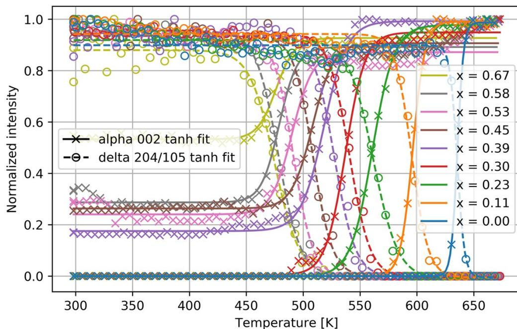
**Fig. S1** The normalized integrated intensity of the 002 peak of the  $\alpha$ -phase (crosses) and 204/105 peaks of the  $\delta$ -phase (circles) as well as the sigmoid fit as a function of heating temperature.
