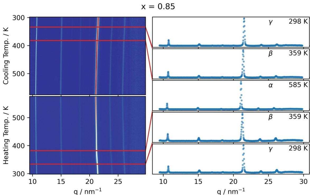
**Fig. S12** Left, integrated GIWAXS pattern as a function of temperature for the spincoated  $\text{CsPb}(\text{Br}_x\text{I}_{1-x})_3$  reference with  $x = 0.85$  (determined by ex-situ XRF) as the sample is heated and then cooled at a rate of 2.5 K/min. Red lines indicate the phase transitions. Right, integrated GIWAXS patterns for the three different phases in the sample.
