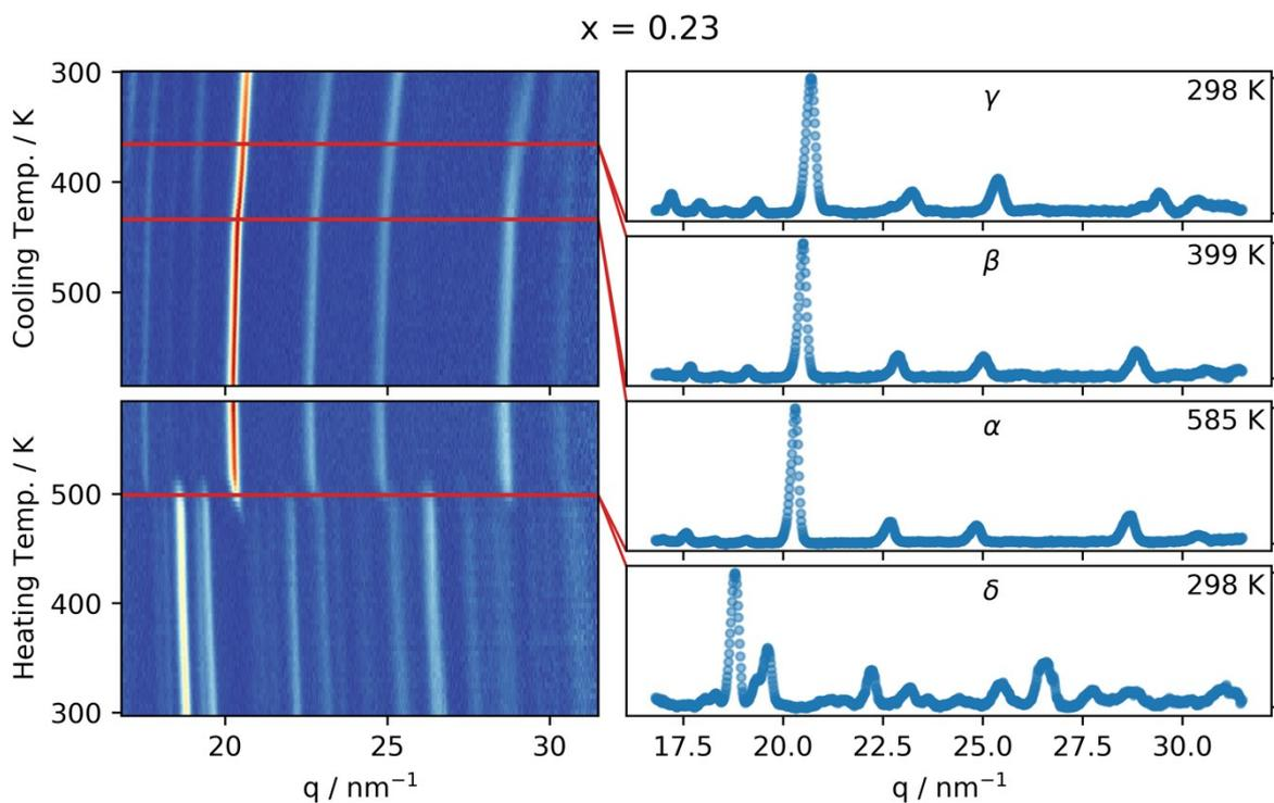
**Fig. S5** Left, integrated GIWAXS pattern as a function of temperature for  $\text{CsPb}(\text{Br}_x\text{I}_{1-x})_3$  with  $x = 0.23$  (determined by in-situ XRF) as the sample is heated and then cooled at a rate of 2.5 K/min. Red lines indicate the phase transitions. Right, integrated GIWAXS patterns for the four different phases in the sample.
