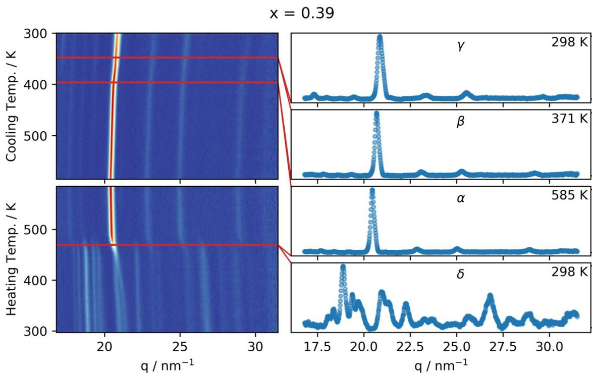
**Fig. S7** Left, integrated GIWAXS pattern as a function of temperature for  $\text{CsPb}(\text{Br}_x\text{I}_{1-x})_3$  with  $x = 0.39$  (determined by in-situ XRF) as the sample is heated and then cooled at a rate of 2.5 K/min. Red lines indicate the phase transitions. Right, integrated GIWAXS patterns for the four different phases in the sample.
