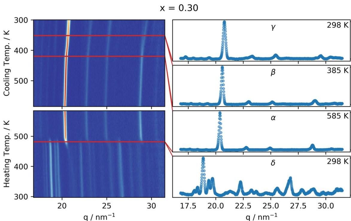
**Fig. S6** Left, integrated GIWAXS pattern as a function of temperature for  $\text{CsPb}(\text{Br}_x\text{I}_{1-x})_3$  with  $x = 0.30$  (determined by in-situ XRF) as the sample is heated and then cooled at a rate of 2.5 K/min. Red lines indicate the phase transitions. Right, integrated GIWAXS patterns for the four different phases in the sample.
