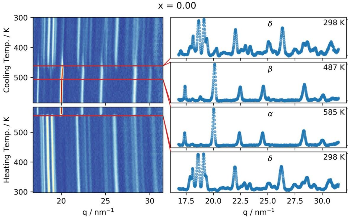
**Fig. S3** Left, integrated GIWAXS pattern as a function of temperature for  $\text{CsPb}(\text{Br}_x\text{I}_{1-x})_3$  with  $x = 0.00$  (determined by in-situ XRF) as the sample is heated and then cooled at a rate of 2.5 K/min. Red lines indicate the phase transitions. Right, integrated GIWAXS patterns for the four different phases in the sample.
