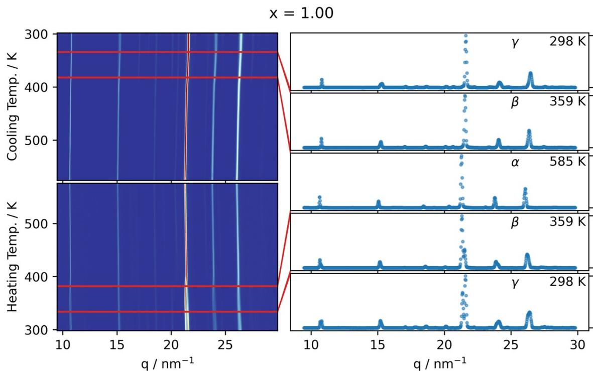
**Fig. S13** Left, integrated GIWAXS pattern as a function of temperature for the blade-coated  $\text{CsPb}(\text{Br}_x\text{I}_{1-x})_3$  reference with  $x = 1$  as the sample is heated and then cooled at a rate of 2.5 K/min. Red lines indicate the phase transitions. Right, integrated GIWAXS patterns for the three different phases in the sample.
