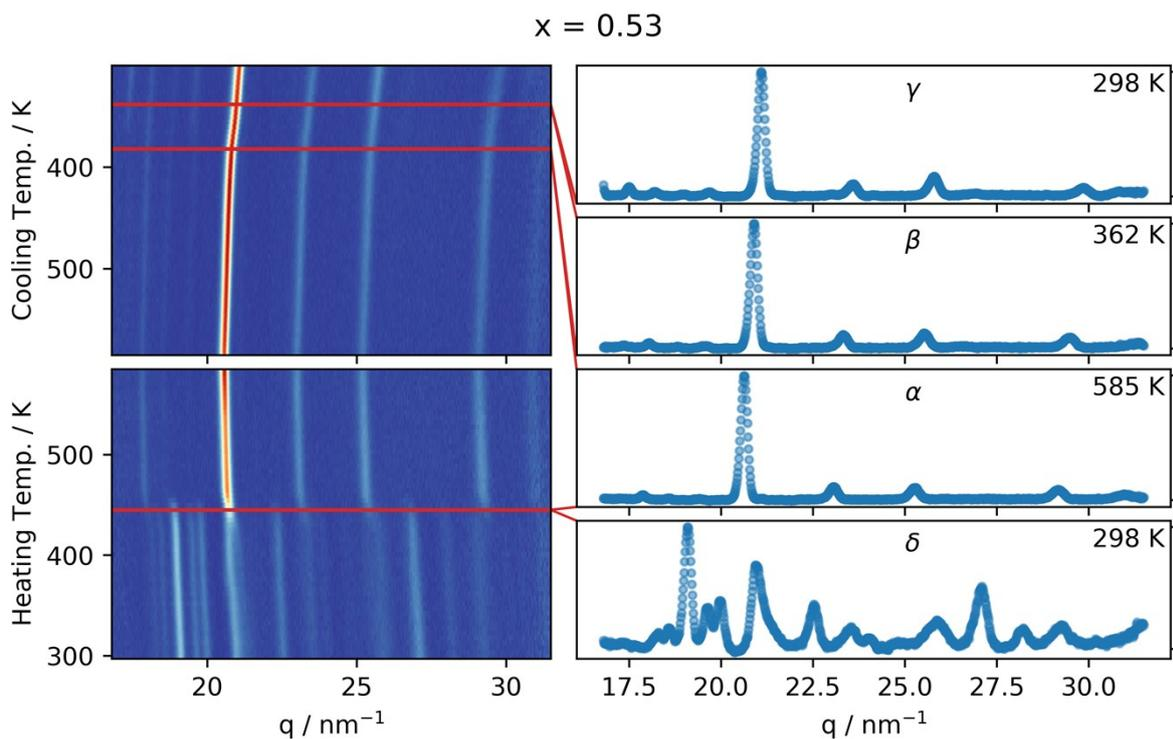
**Fig. S9** Left, integrated GIWAXS pattern as a function of temperature for  $\text{CsPb}(\text{Br}_x\text{I}_{1-x})_3$  with  $x = 0.53$  (determined by in-situ XRF) as the sample is heated and then cooled at a rate of 2.5 K/min. Red lines indicate the phase transitions. Right, integrated GIWAXS patterns for the four different phases in the sample.
