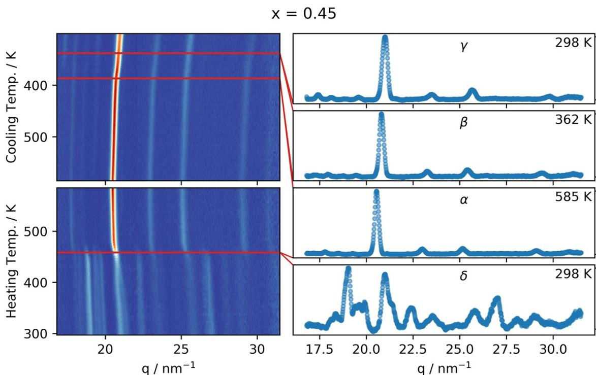
**Fig. S8** Left, integrated GIWAXS pattern as a function of temperature for  $\text{CsPb}(\text{Br}_x\text{I}_{1-x})_3$  with  $x = 0.45$  (determined by in-situ XRF) as the sample is heated and then cooled at a rate of 2.5 K/min. Red lines indicate the phase transitions. Right, integrated GIWAXS patterns for the four different phases in the sample.
