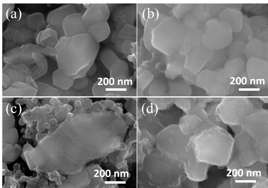
**Fig. S4** The FE-SEM images of (a)LL, (b)LLM2 before cycling and (c)LL, (d)LLM2 after cycling at 1C for 100 cycles.
