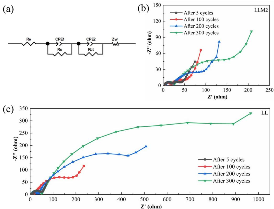
**Fig. S5** (a) the equivalent circuit model, and the EIS Nyquist plots of (b)LLM2, (c)LL.
