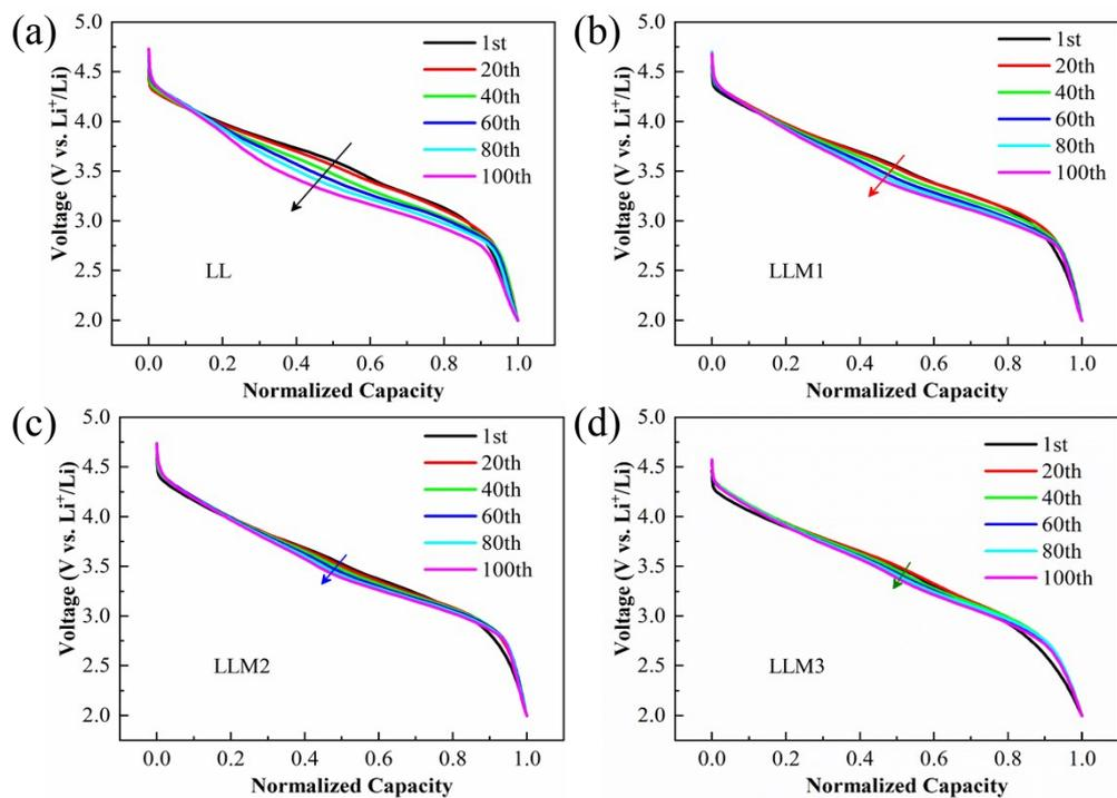
**Fig. S1** The discharge curves of cycling at 1C normalized by discharging capacities of LL, LLM1, LLM2, and LLM3 respectively.
