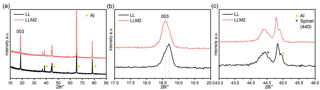
**Fig. S3** (a) XRD patterns of the electrodes after 100 cycles at 1C, (b) the enlarge XRD pattern between 17.0 and 20.0 degree, (c) the enlarge XRD pattern between 43.0 and 46.0 degree.
