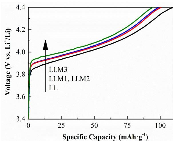
**Fig. S2** Initial charge curves at 3.4-4.4 V of LL, LLM1, LLM2 and LLM3 cathodes.
