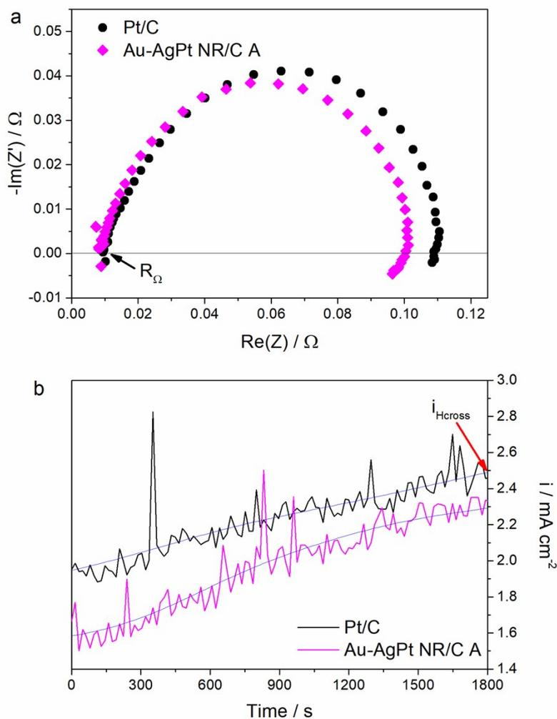
Fig. S10. a) EIS measured in  $\text{H}_2/\text{O}_2$  at  $30 \text{ mA cm}^{-2}$  with an amplitude of  $4.5 \text{ mA cm}^{-2}$  in the frequency range of  $10 \text{ kHz} - 0.1 \text{ Hz}$ ; and b)  $\text{H}_2$  - crossover current density recorded by holding at  $0.5 \text{ V}$  vs. RHE under  $\text{H}_2/\text{N}_2$  feeds.
