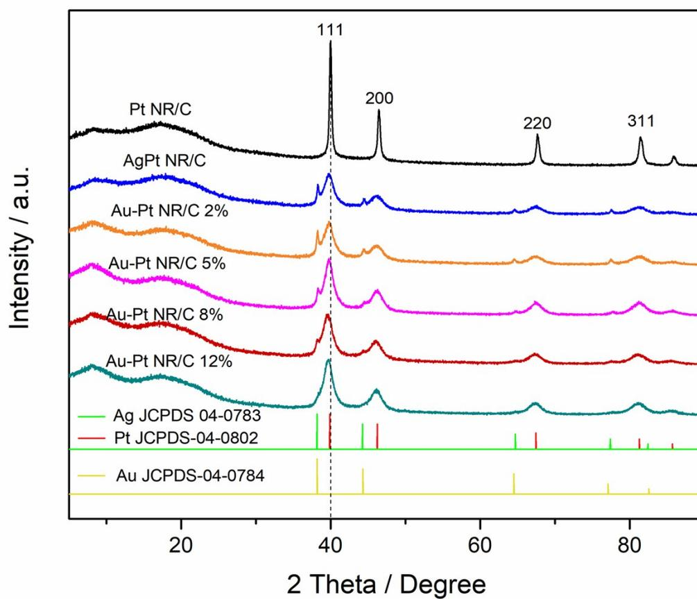
Fig. S3. XRD patterns of the Pt NR/C, AgPt NR/C and Au-AgPt NR/C catalysts with various Au contents synthesized following the reaction scheme A.
