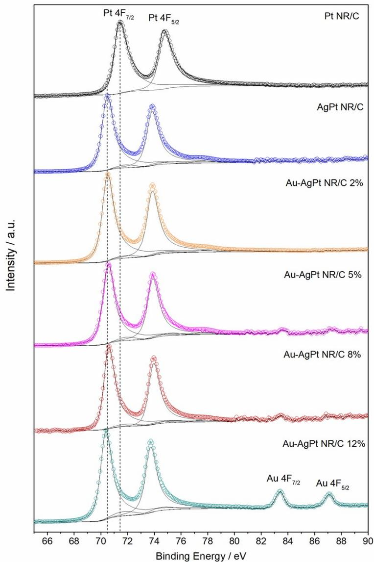
Fig. S4. High-resolution XPS spectra of the Pt 4f region generated for the Pt NR/C, AgPt NR/C and Au-AgPt NR/C catalysts with various Au contents synthesized following the reaction scheme A.
