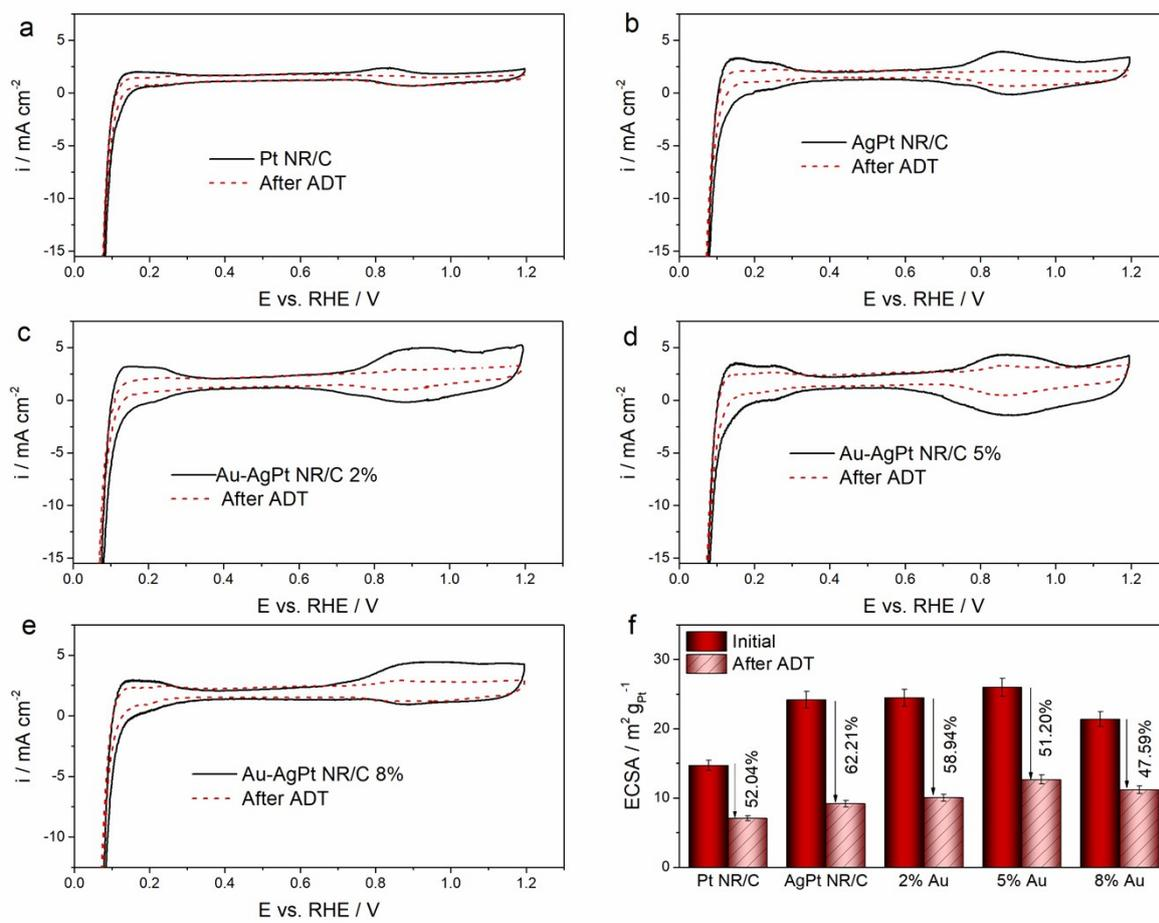
Fig. S12. Cathode CVs and the corresponding ECSA decline ratio after the ADT for MEAs with the cathode catalysts made of Pt NR/C, AgPt NR/C and Au-AgPt NR/C with various Au contents synthesized following the reaction scheme A. The ADT was performed using potential sweeping between 0.6-1.2 V at a scan rate of  $100 \text{ mV s}^{-1}$  for 5000 cycles with  $\text{H}_2/\text{N}_2$ .
