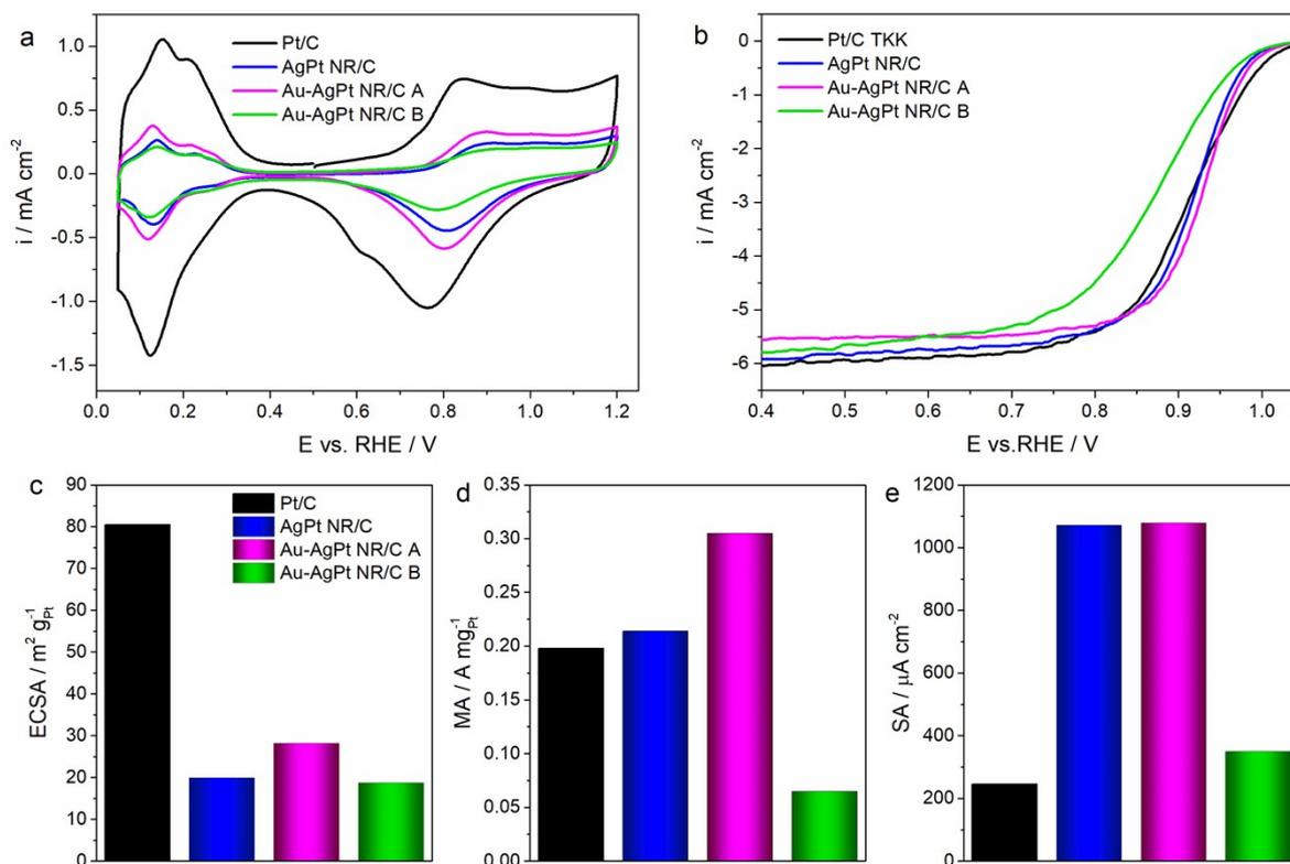
Fig. S8. Catalytic activities of the commercial Pt/C and as-prepared catalysts measured in 0.1 M HClO<sub>4</sub>(aq) electrolyte using the rotating disc electrode (RDE) method; a) CV plots recorded with a scan rate of 20 mV s<sup>-1</sup> in the N<sub>2</sub> saturated electrolyte, and b) LSV plots recorded at 1600 rpm with a scan rate of 20 mV s<sup>-1</sup> in the oxygen saturated electrolyte. The corresponding c) ECSA, b) mass activity (MA) and c) specific activity (SA).
