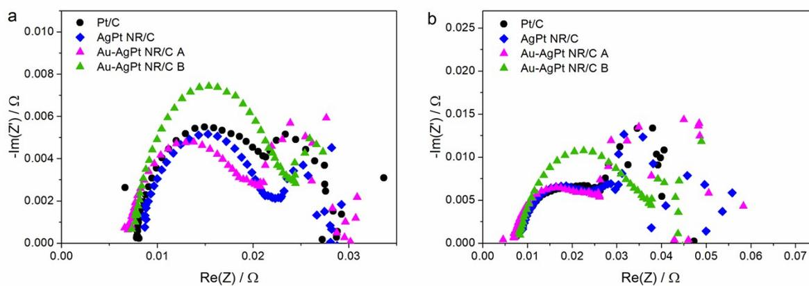
Fig. S6. EIS spectra recorded at a) 0.65 V and b) 0.5 V with an amplitude of 10 mV in the frequency range 10k–0.1 Hz.
