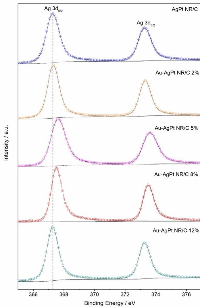
Fig. S5. High resolution XPS spectra of the Ag 3d region generated for the AgPt NR/C and Au-AgPt NR/C catalysts with various Au contents synthesized following the reaction scheme A.
