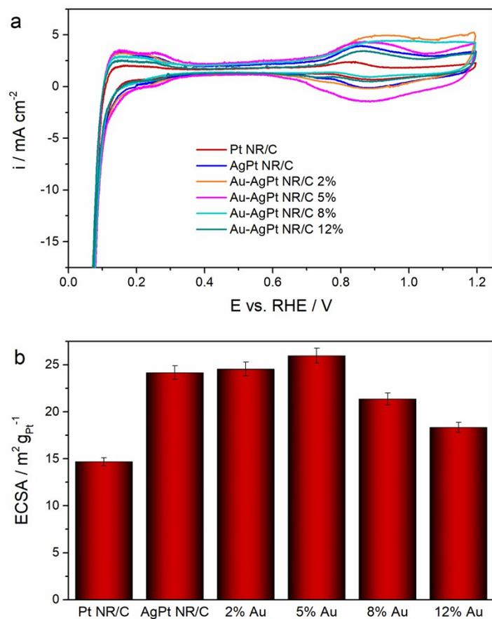
Fig. S9. a) Cathode CVs recorded between 0.05-1.2 V with a scan rate of 20 mV s<sup>-1</sup> in the MEAs under H<sub>2</sub>/N<sub>2</sub>, and b) corresponding ECSA.
