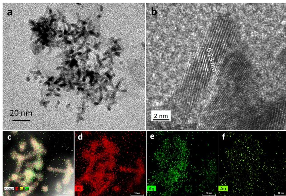
Fig. S1. a-c) TEM images of the Au-AgPt NR/C B catalyst synthesized following the reaction scheme B, and d-g) show the element mapping by EDX analysis.
