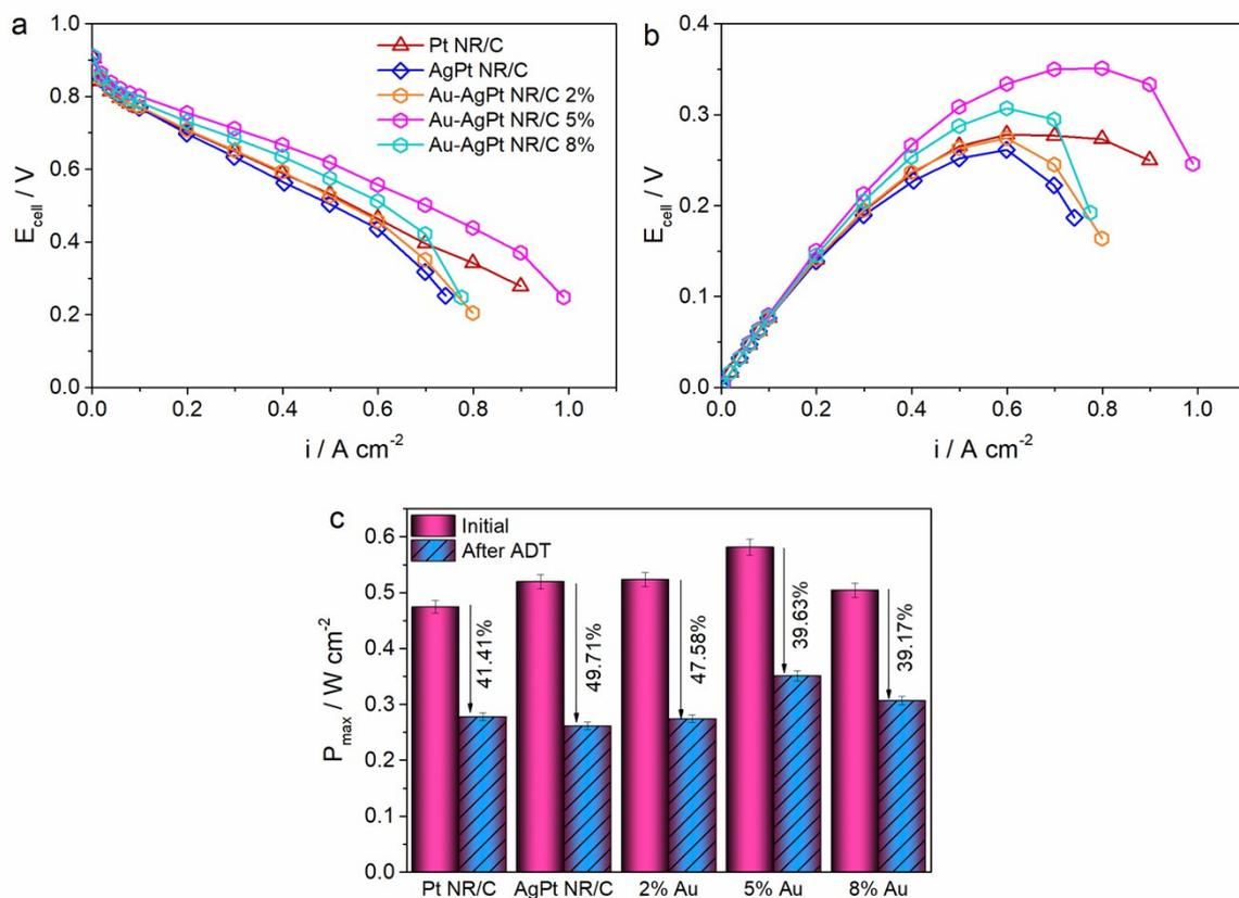
Fig. S11. a) Polarization and b) power density curves recorded after the ADT and c) corresponding peak power density comparison before and after the ADT for MEAs with the cathode catalysts made of Pt NR/C, AgPt NR/C and Au-AgPt NR/C with various Au contents synthesized following the reaction scheme A. The ADT was performed using potential sweeping between 0.6-1.2 V at a scan rate of  $100 \text{ mV s}^{-1}$  for 5000 cycles with  $\text{H}_2/\text{N}_2$ .
