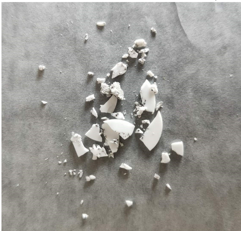
Figure S4. The optical image of the LAGP pellet after cycling in Li-LAGP-Li cell.
